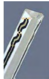
Figure 3.3 Probe Thick-Film Technique
