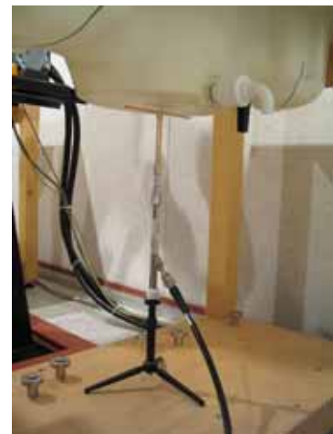
Photo of the dipole Antenna
