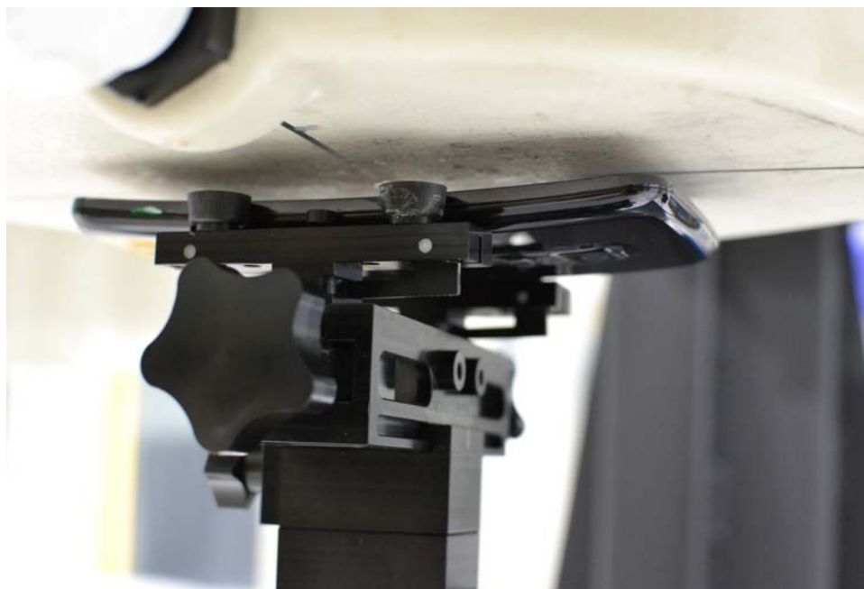
SAR Test Setup Photo 7: Front Side at 0.8 cm
