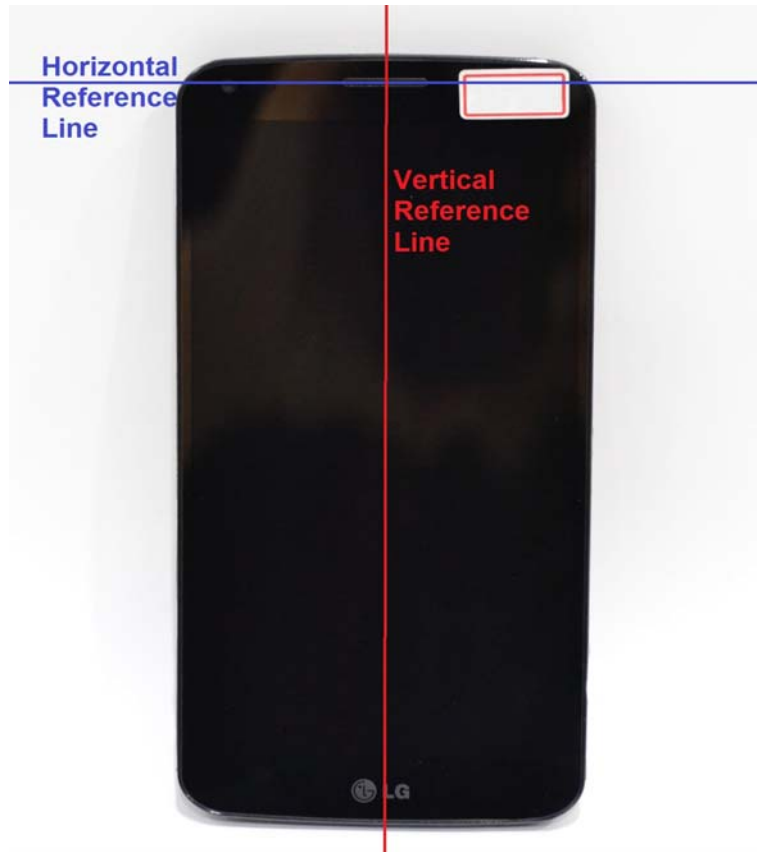
SAR Test Setup Photo 15: Horizontal and Vertical Reference Lines
