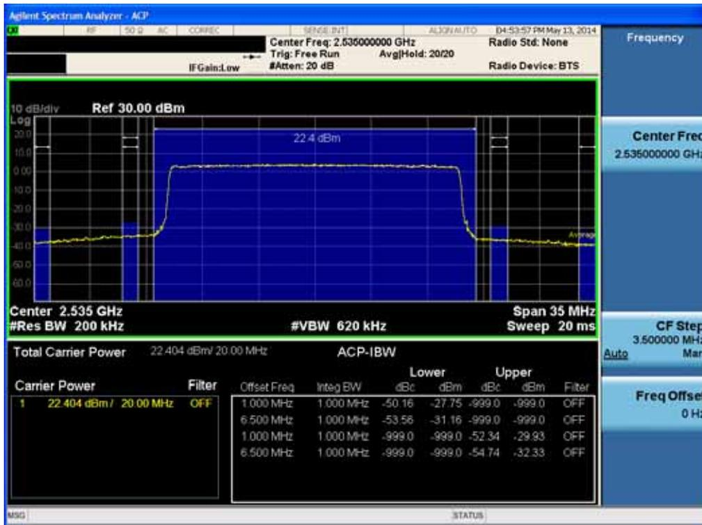
High Channel Edge Plot (20MHz Ch.21350 QPSK RB 100)
