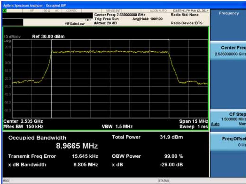
Occupied Bandwidth Plot (10MHz Ch.21100 16-QAM RB 50)
