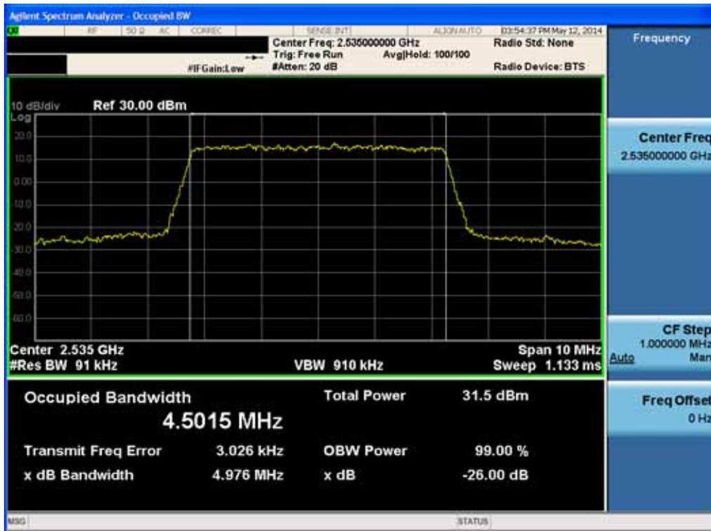
Occupied Bandwidth Plot (5MHz Ch.21100 16-QAM RB 25)
