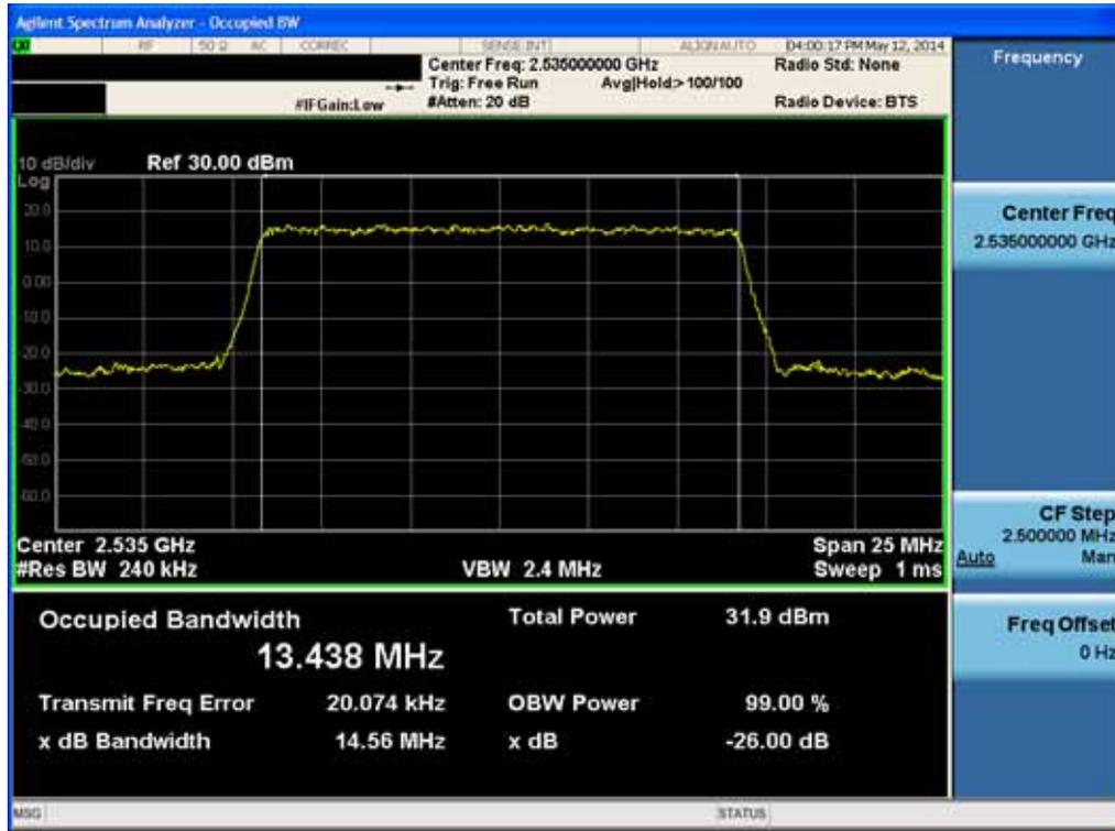
Occupied Bandwidth Plot (15MHz Ch.21100 16-QAM RB 75)
