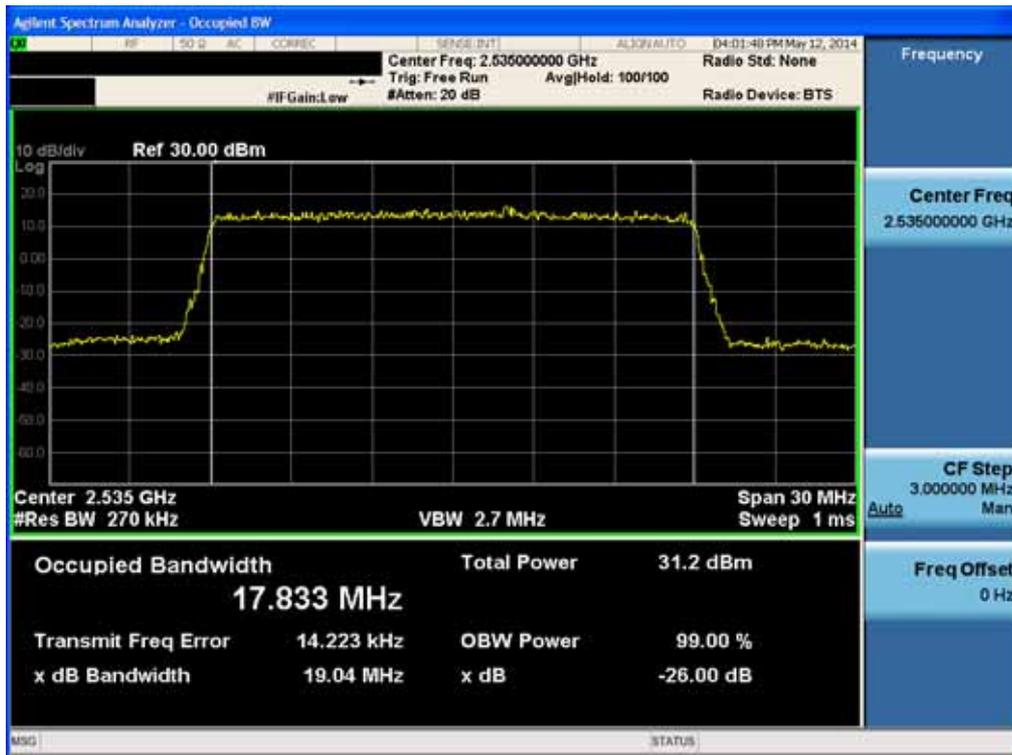
Occupied Bandwidth Plot (20MHz Ch.21100 16-QAM RB 100)
