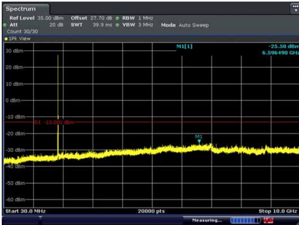
BAND 2. Conducted Spurious\_2 (18675ch\_15MHz\_QPSK\_RB 1\_0)
