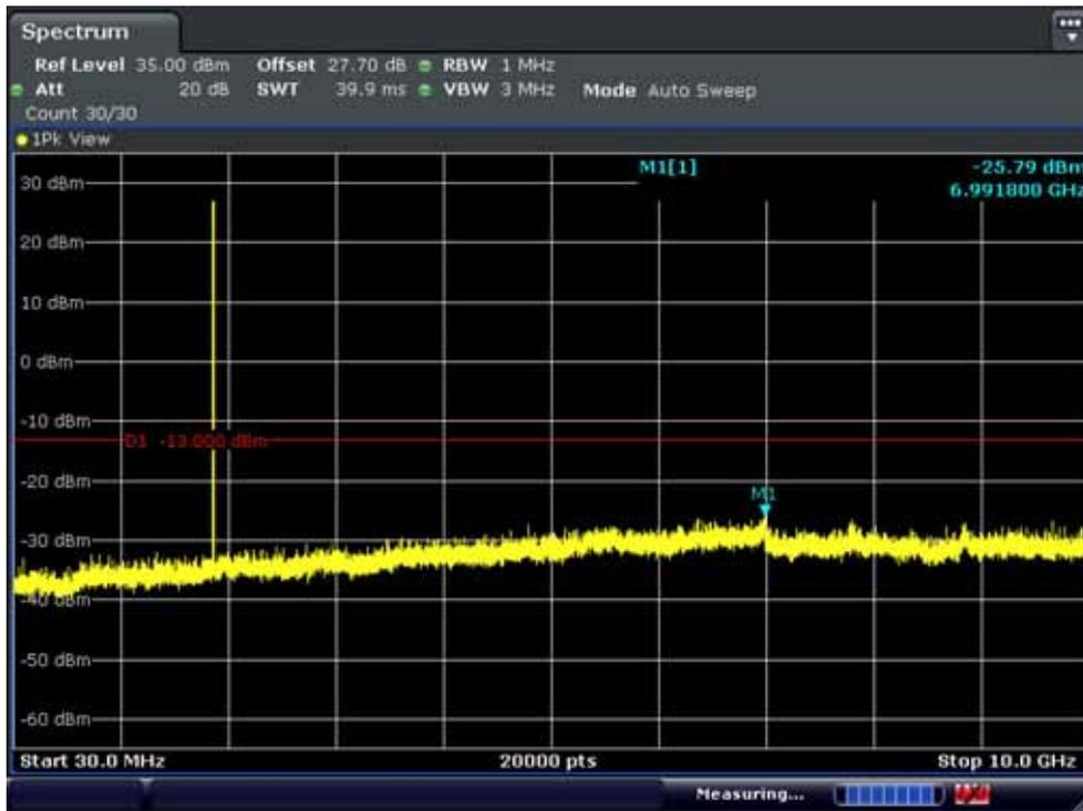
BAND 2. Conducted Spurious\_2 (18900ch\_3MHz\_QPSK\_RB 1\_0)
