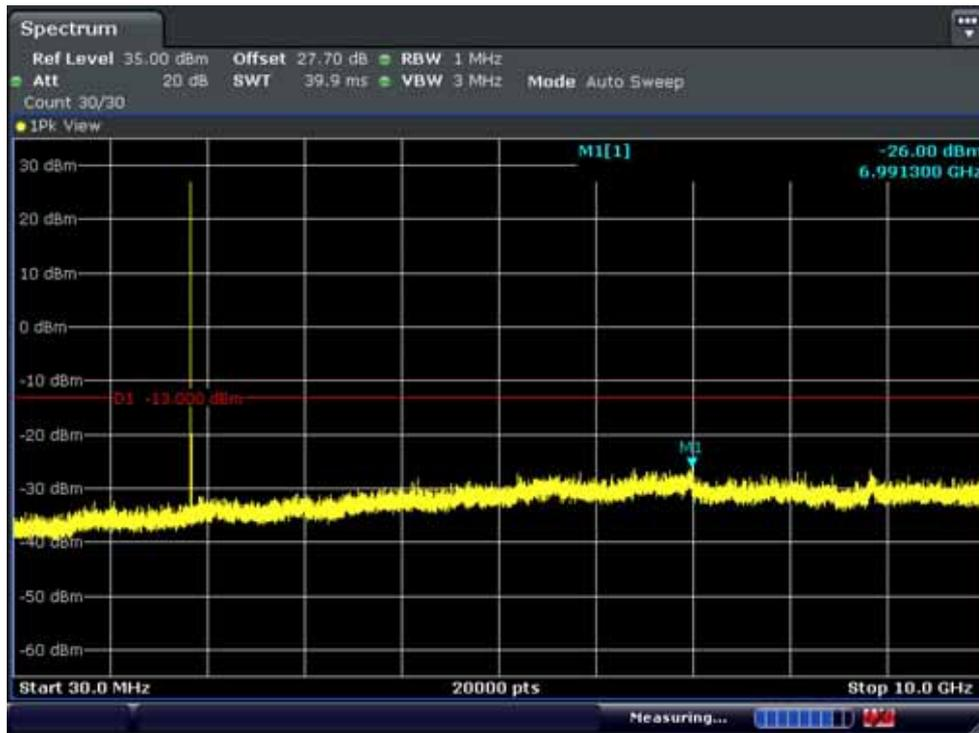
BAND 2. Conducted Spurious (18615ch\_3MHz\_QPSK\_RB 1\_0)
