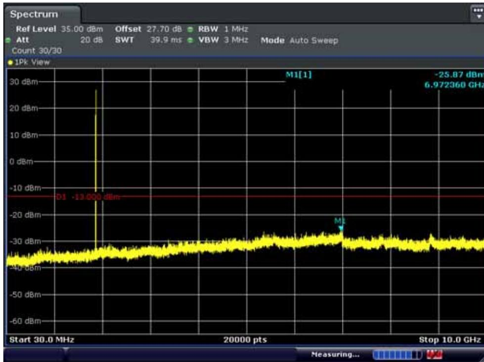
BAND 2. Conducted Spurious\_2 (18900ch\_1.4MHz\_QPSK\_RB 1\_0)
