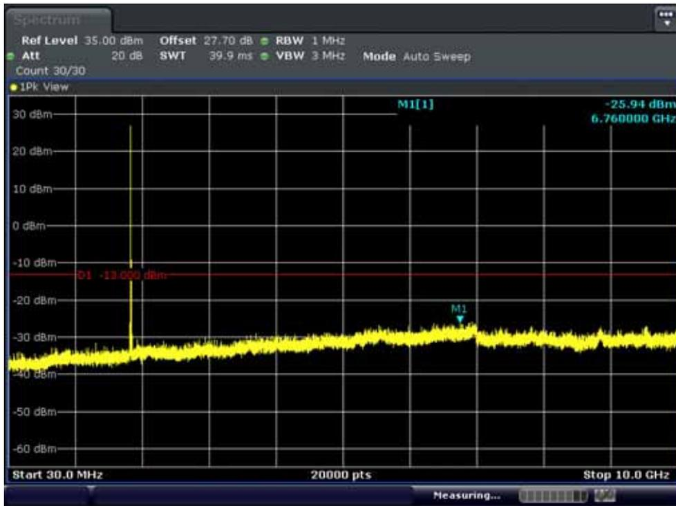
BAND 2. Conducted Spurious\_2 (18650ch\_10MHz\_QPSK\_RB 1\_0)
