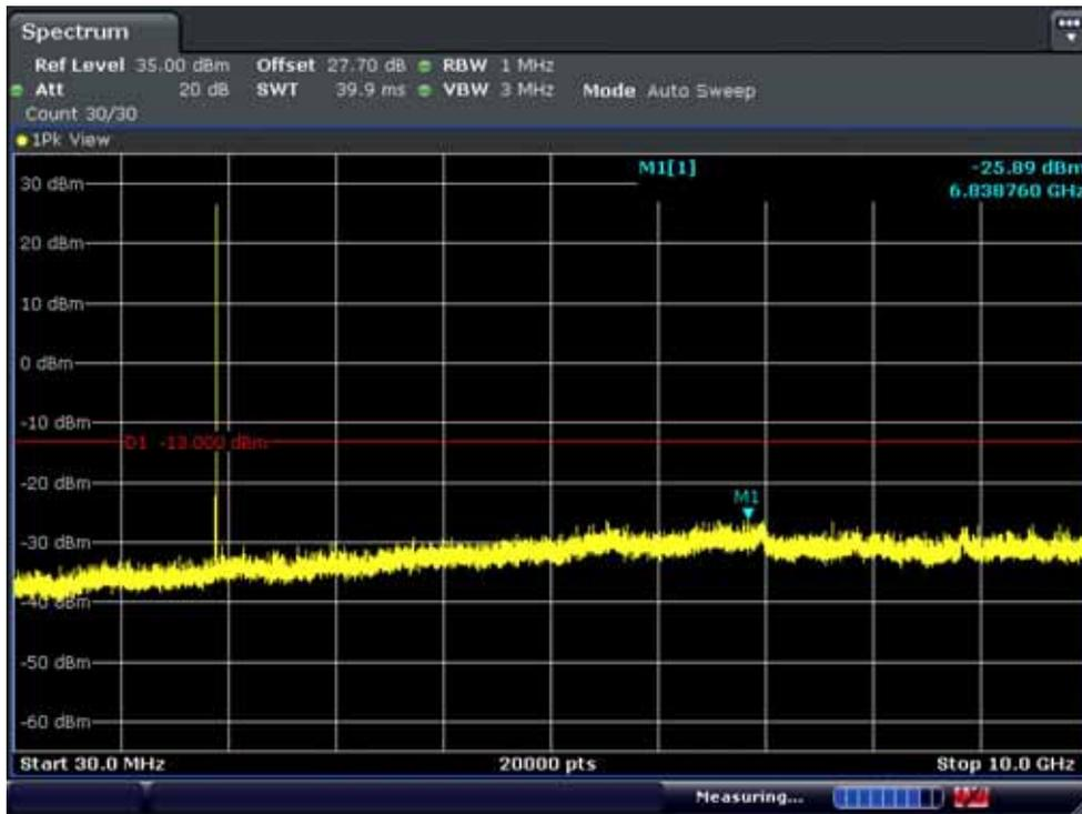
BAND 2. Conducted Spurious\_2 (19185ch\_3MHz\_QPSK\_RB 1\_0)
