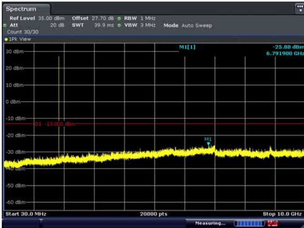
BAND 2. Conducted Spurious (18607ch\_1.4MHz\_QPSK\_RB 1\_0)
