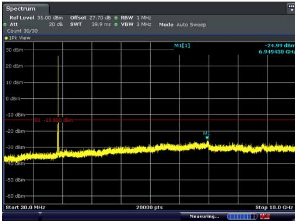
BAND 2. Conducted Spurious\_2 (18900ch\_20MHz\_QPSK\_RB 1\_0)
