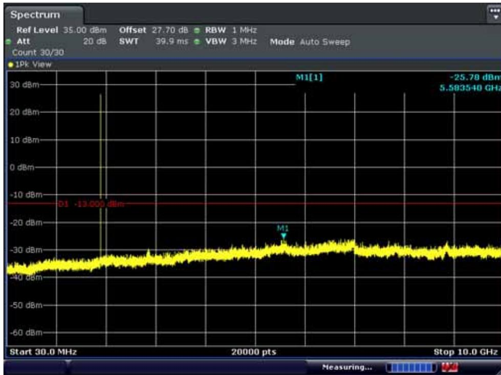
BAND 2. Conducted Spurious\_2 (19193ch\_1.4MHz\_QPSK\_RB 1\_0)
