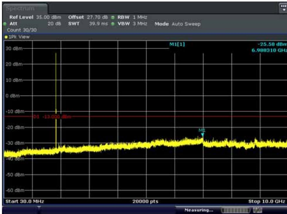
BAND 2. Conducted Spurious (18625ch\_5MHz\_QPSK\_RB 1\_0)
