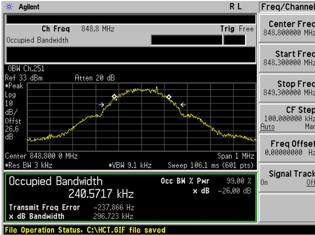
■ GSM850 EDGE (190 CH.) Occupied Bandwidth
