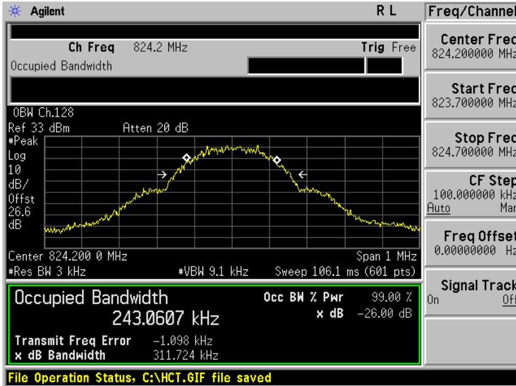
■ GSM850 MODE (190 CH.) Occupied Bandwidth
