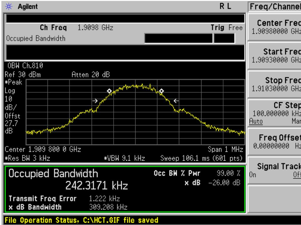
■ GSM1900 EDGE (661 CH.) Occupied Bandwidth
