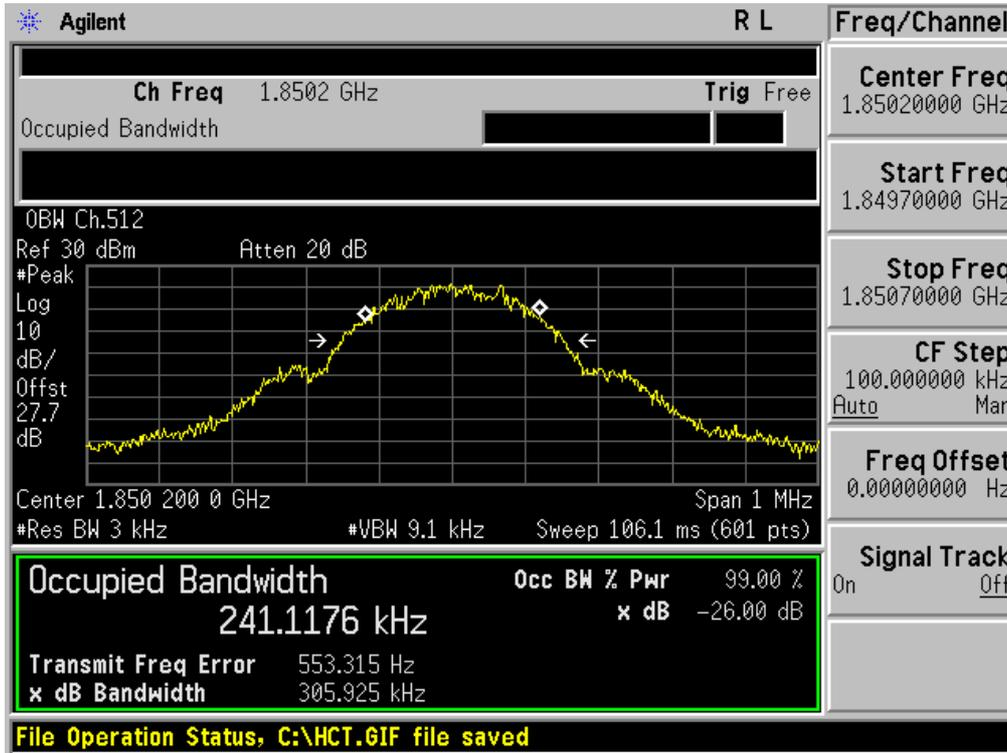
■ GSM1900 MODE (661 CH.) Occupied Bandwidth
