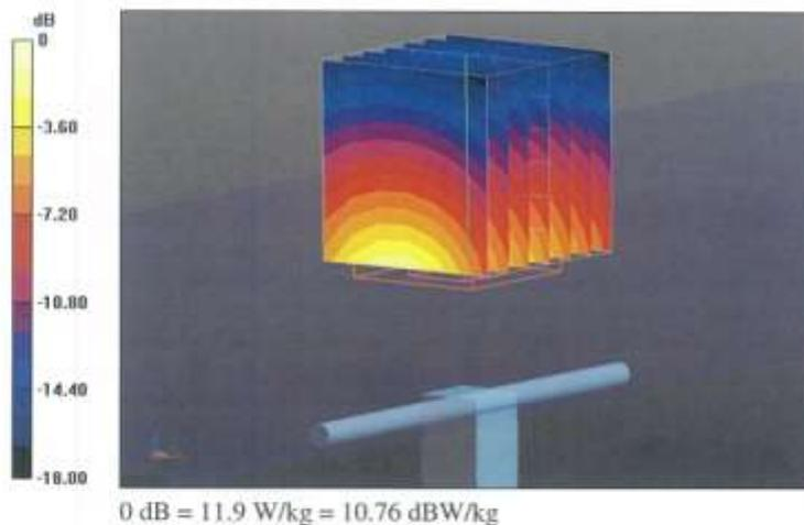
Impedance Measurement Plot for Head TSL
