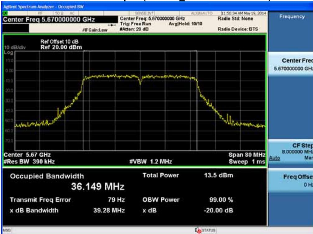
20 dB Bandwidth plot (802.11ac\_40 MHz BW-CH 134)
