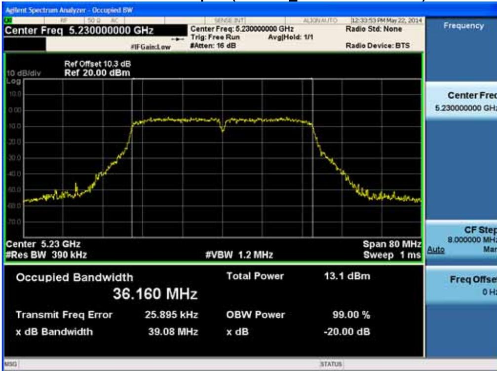
20 dB Bandwidth plot (802.11n\_40 MHz BW-CH 54)
