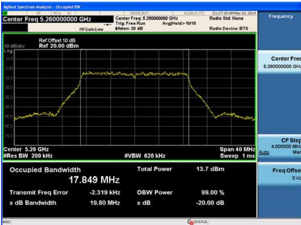
20 dB Bandwidth plot (802.11n\_40 MHz BW-CH 46)
