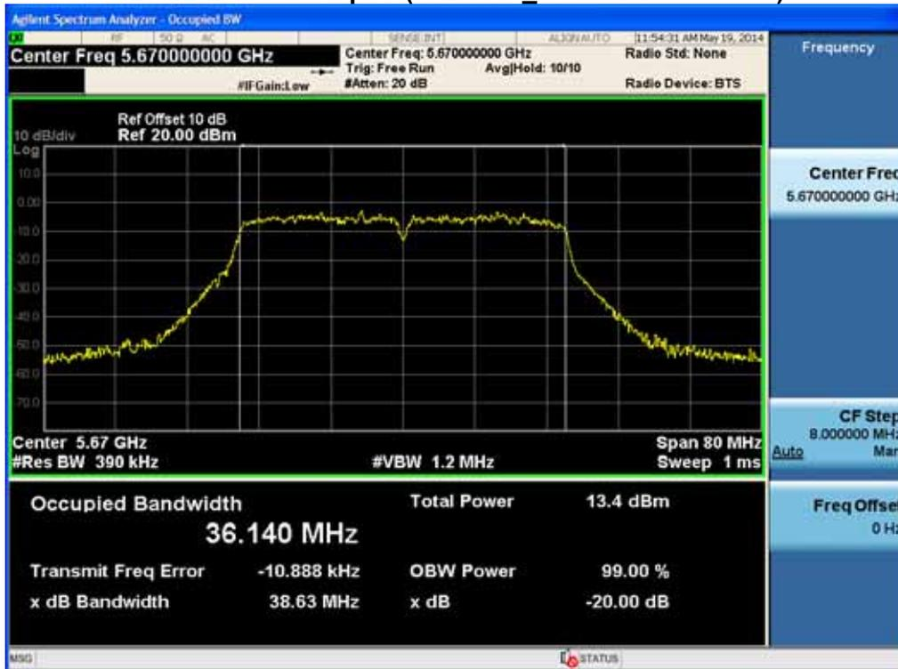
20 dB Bandwidth plot (802.11ac\_80 MHz BW-CH 138)
