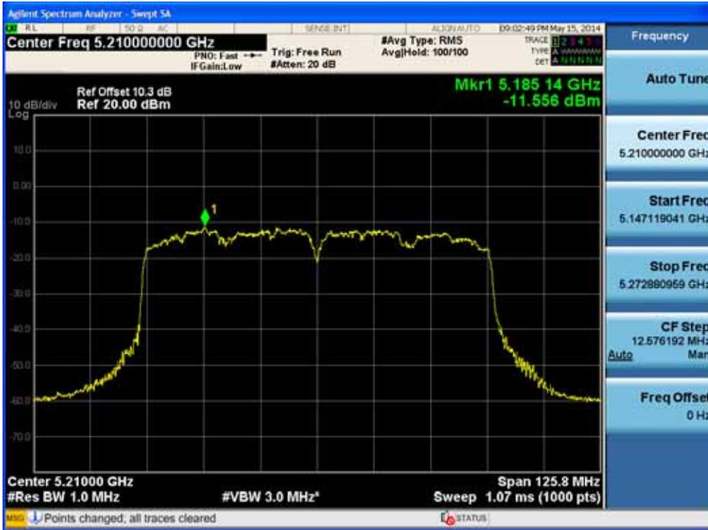
Power Spectral Density (802.11ac-CH 58)
