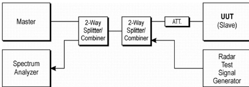
**Figure 3-1. Conducted Test Setup for DFS**
