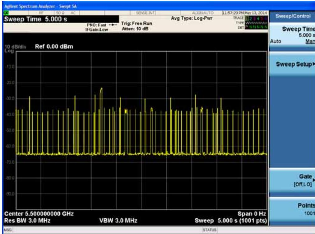
Time Display, WLAN Channel Traffic (Streaming Video)
