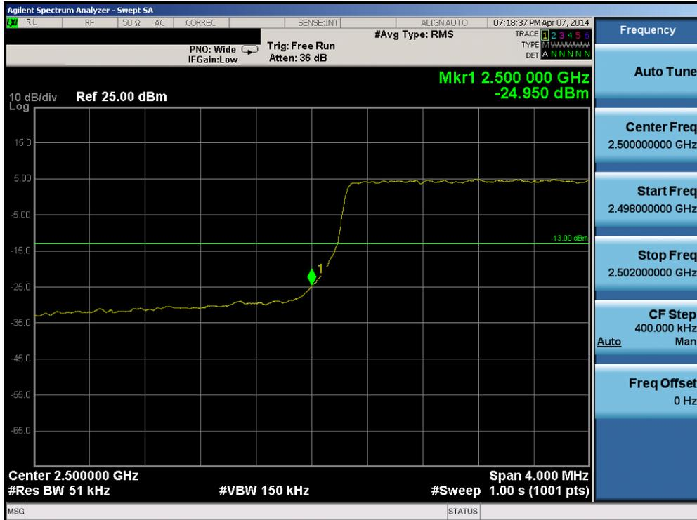
Plot 6-103. Lower Band Edge Plot (Band 7 – 5.0MHz QPSK – RB Size 25)
