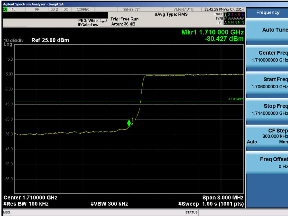
Plot 6-75. Lower Band Edge Plot (Band 4 – 10.0MHz QPSK – RB Size 50)
