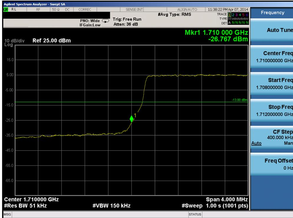
Plot 6-71. Lower Band Edge Plot (Band 4 – 5.0MHz QPSK – RB Size 25)
