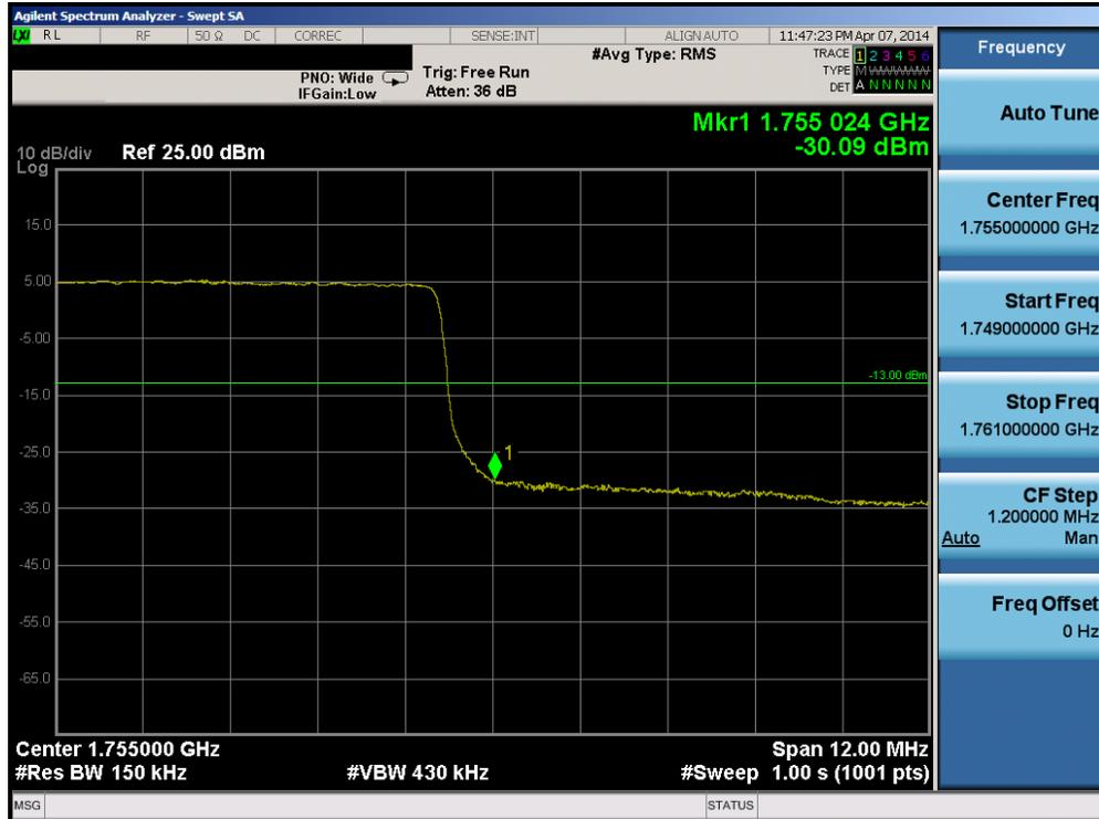
Plot 6-81. Upper Band Edge Plot (Band 4 – 15.0MHz QPSK – RB Size 75)
