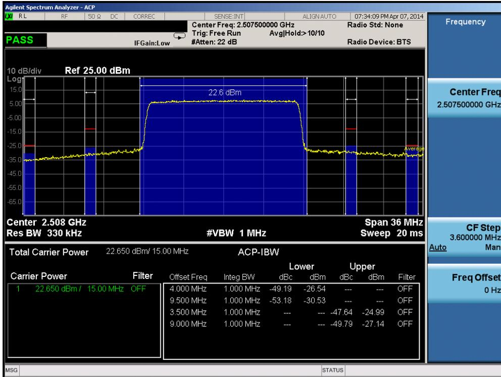
Plot 6-121. Lower ACP Plot (Band 7 – 15.0MHz QPSK – RB Size 75)
