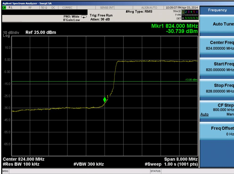
Plot 6-69. Lower Band Edge Plot (Band 5 – 10.0MHz QPSK – RB Size 50)
