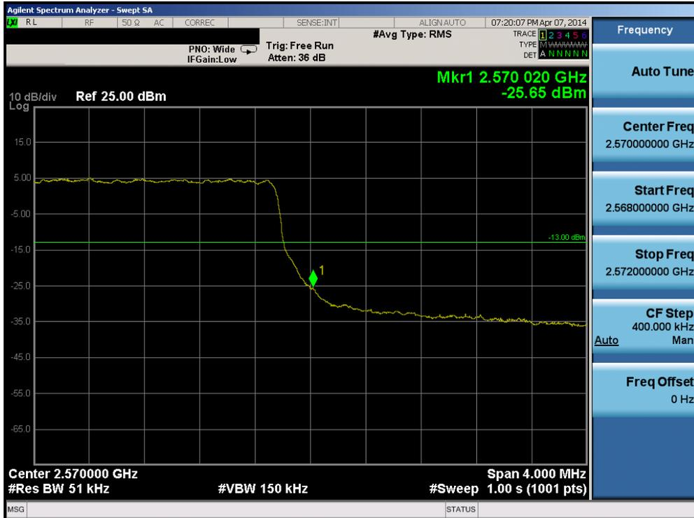
Plot 6-105. Upper Band Edge Plot (Band 7 – 5.0MHz QPSK – RB Size 25)
