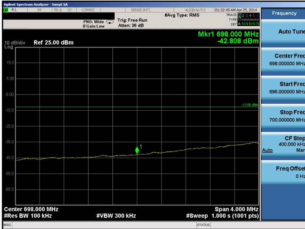
Plot 6-63. Lower Band Edge Plot (Band 17 – 5.0MHz QPSK – RB Size 25)
