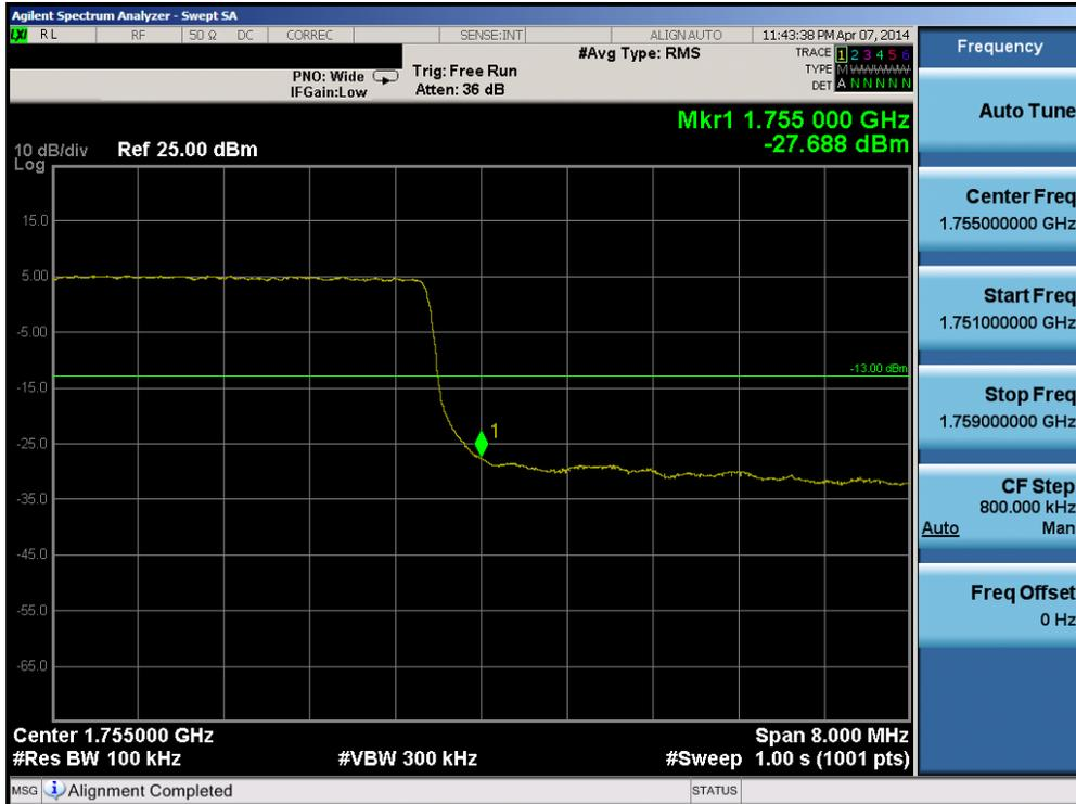
Plot 6-77. Upper Band Edge Plot (Band 4 – 10.0MHz QPSK – RB Size 50)
