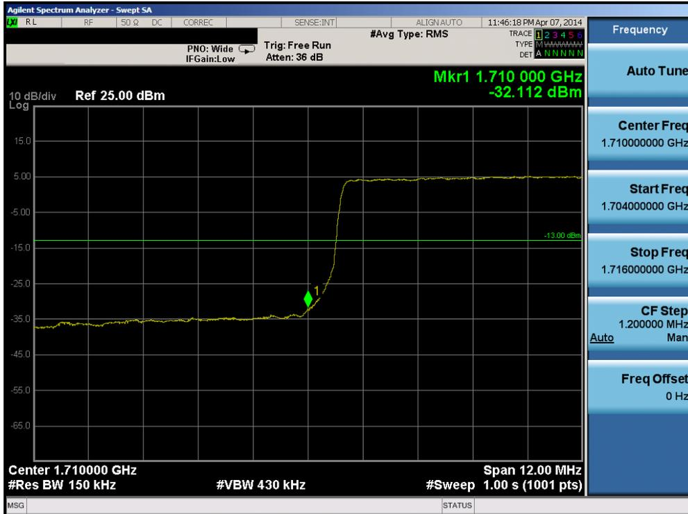
Plot 6-79. Lower Band Edge Plot (Band 4 – 15.0MHz QPSK – RB Size 75)
