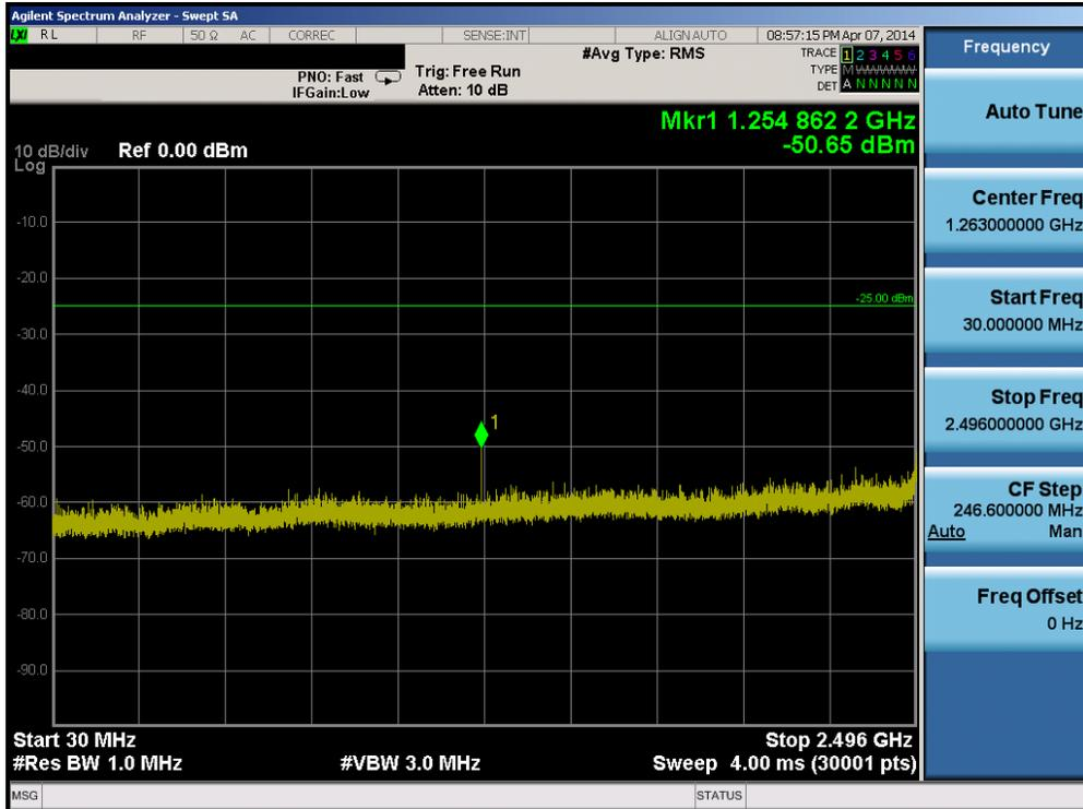
Plot 6-59. Conducted Spurious Plot (Band 7 – 5.0MHz QPSK – RB Size 1, RB Offset 0 – Mid Channel)
