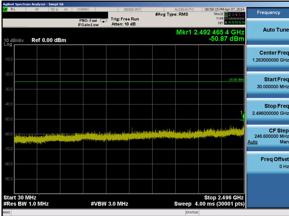
Plot 6-61. Conducted Spurious Plot (Band 7 – 5.0MHz QPSK – RB Size 1, RB Offset 0 – High Channel)
