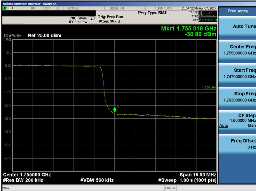
Plot 6-85. Upper Band Edge Plot (Band 4 – 20.0MHz QPSK – RB Size 100)
