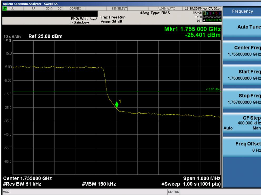
Plot 6-73. Upper Band Edge Plot (Band 4 – 5.0MHz QPSK – RB Size 25)
