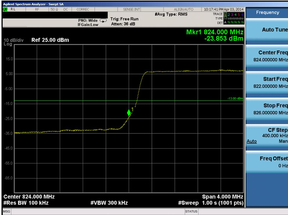
Plot 6-67. Lower Band Edge Plot (Band 5 – 5.0MHz QPSK – RB Size 25)
