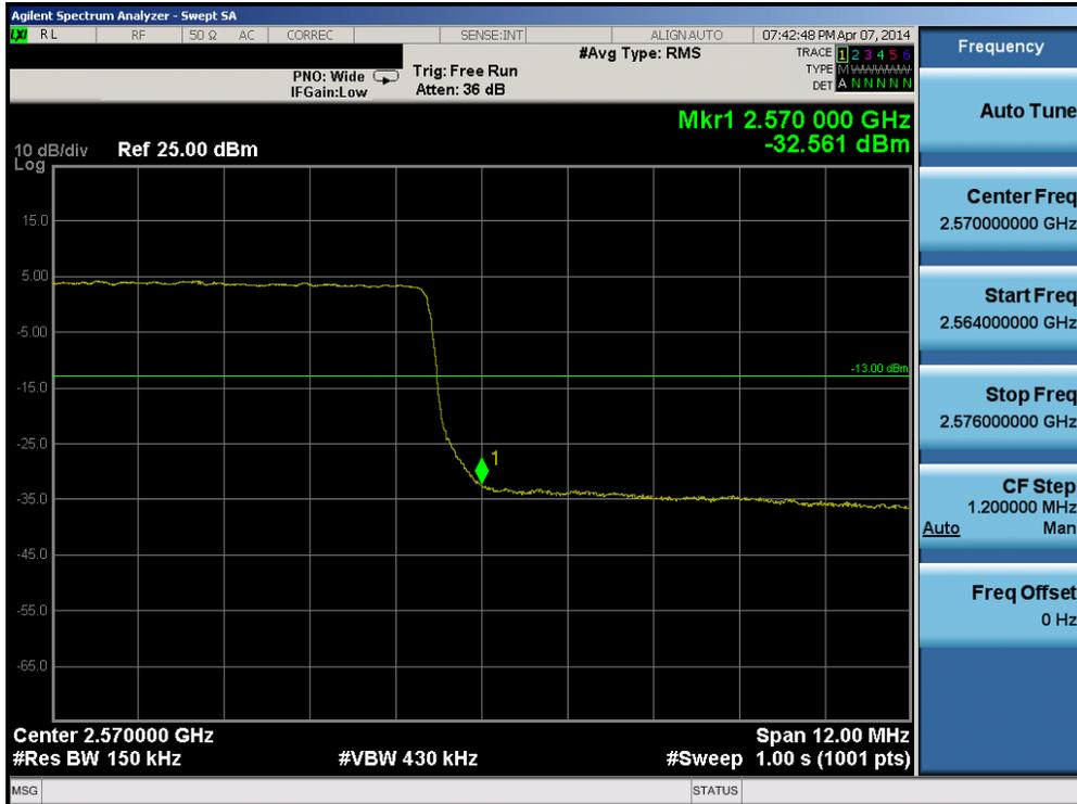
Plot 6-119. Upper Band Edge Plot (Band 7 – 15.0MHz QPSK – RB Size 75)
