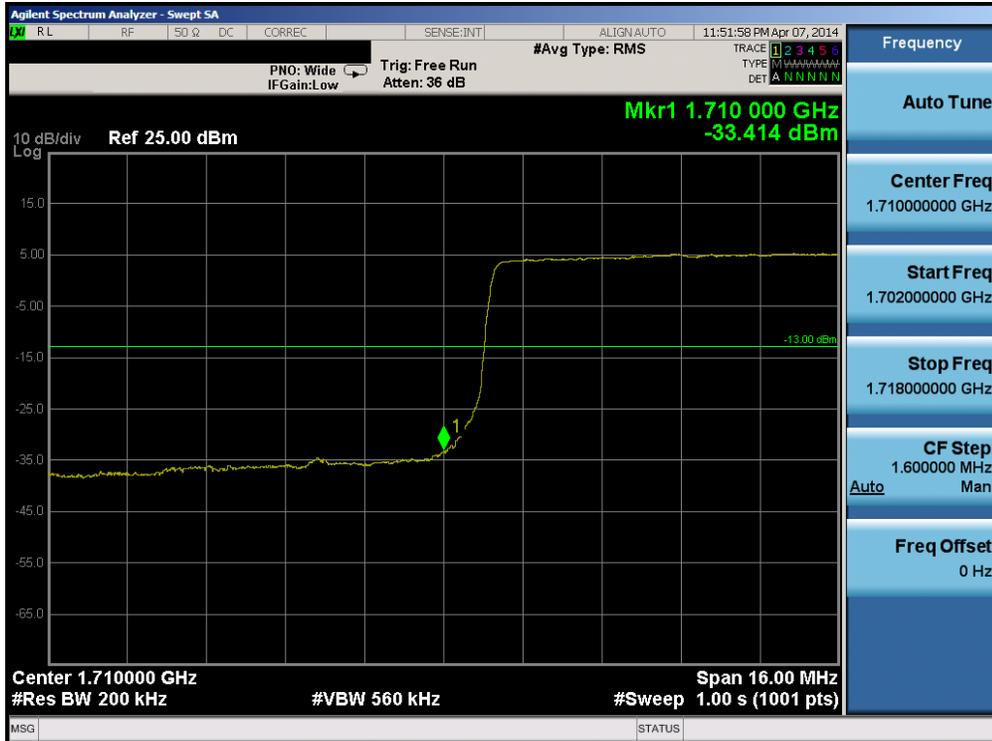
Plot 6-83. Lower Band Edge Plot (Band 4 – 20.0MHz QPSK – RB Size 100)
