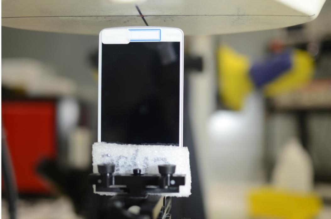
**SAR Test Setup Photo 15 - Bottom at 10 mm**
