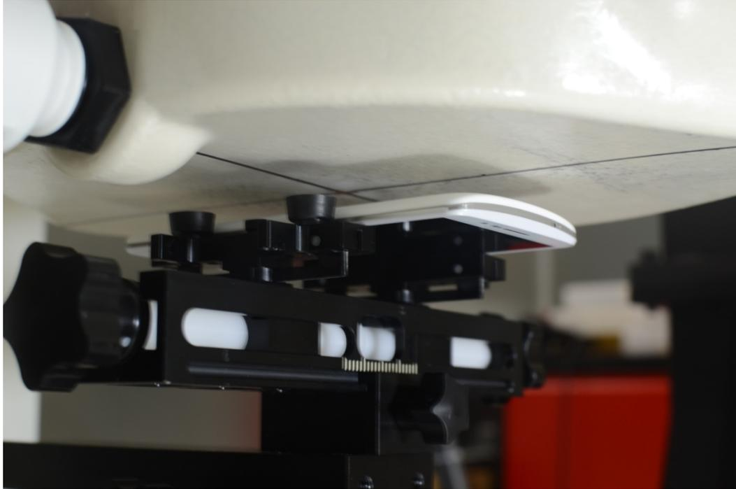
**SAR Test Setup Photo 11 - Back at 10 mm**
