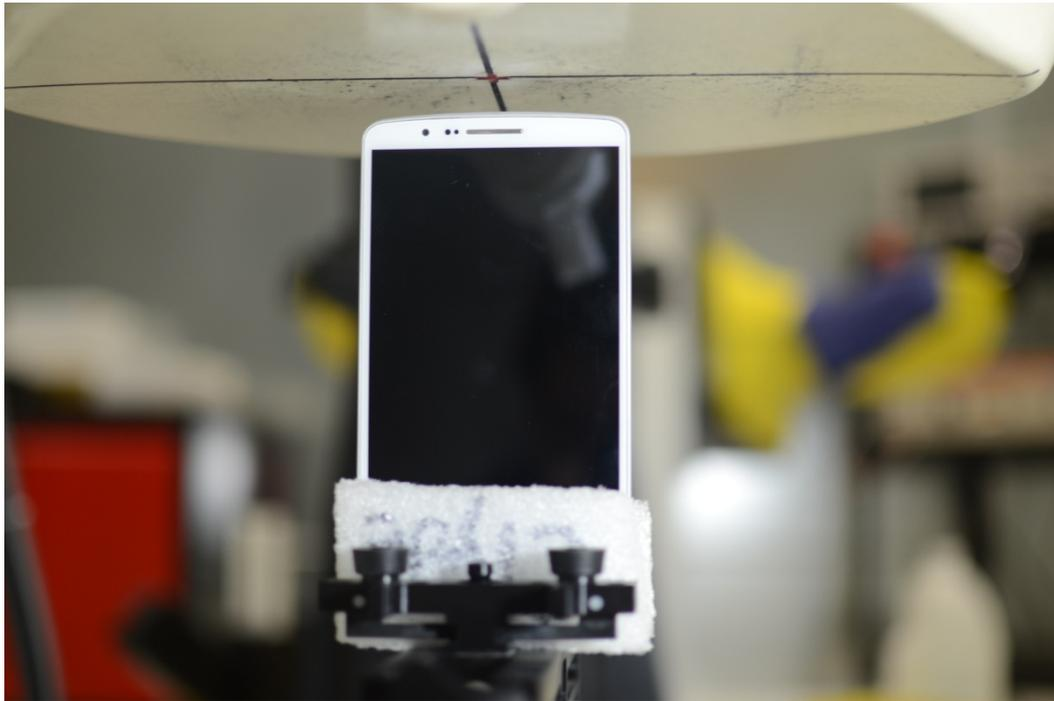
SAR Test Setup Photo 14 - Top at 10 mm
