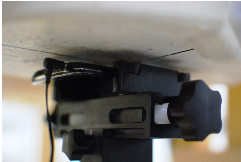
SAR Test Setup Photo 6: Back Side with Headset at 1.0 cm
