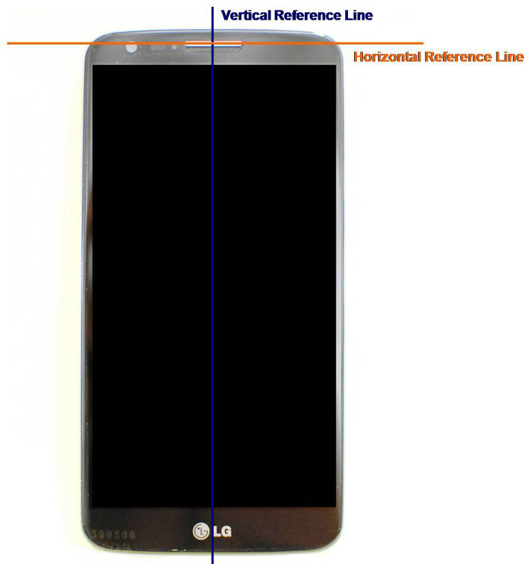
SAR Test Setup Photo 12: Horizontal and Vertical Reference Lines
