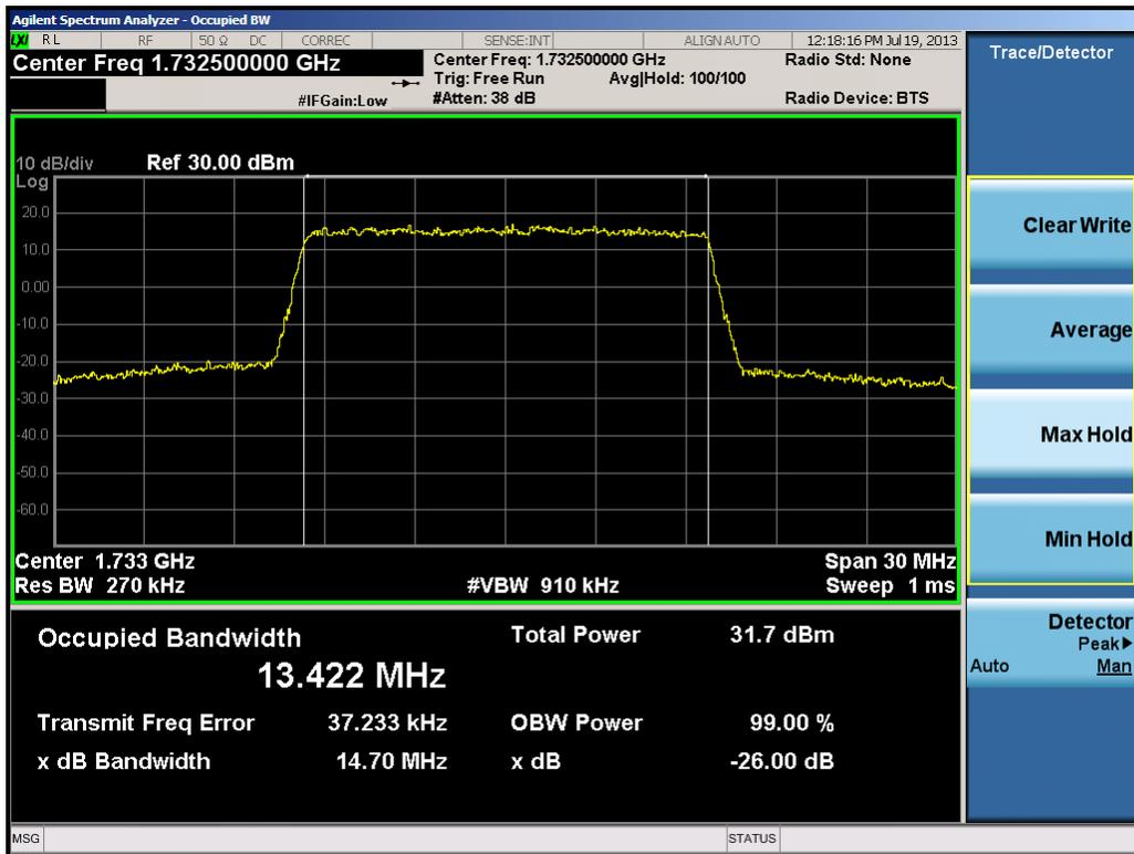
Plot 8-25. Occupied Bandwidth Plot (15.0MHz QPSK – RB Size 75)
