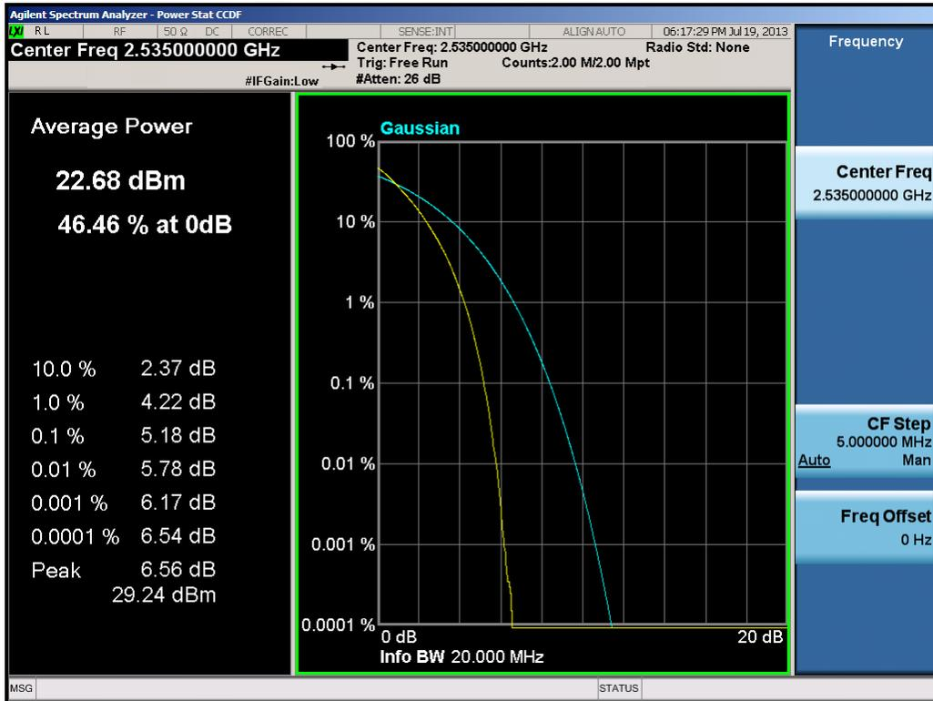
Plot 9-39. PAR Plot (20.0MHz QPSK – RB Size 100)
