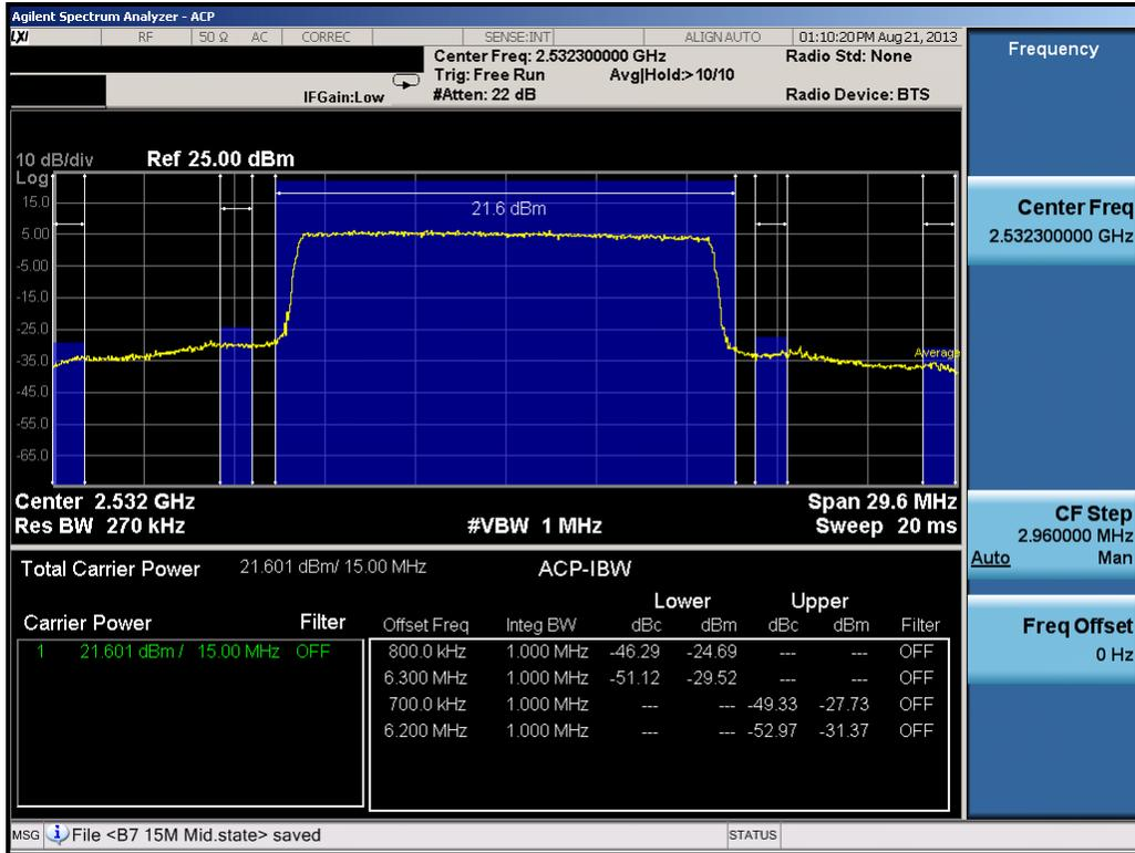
Plot 9-24. Mid Channel Adjacent Channel Power Plot (15.0MHz QPSK – RB Size 75)
