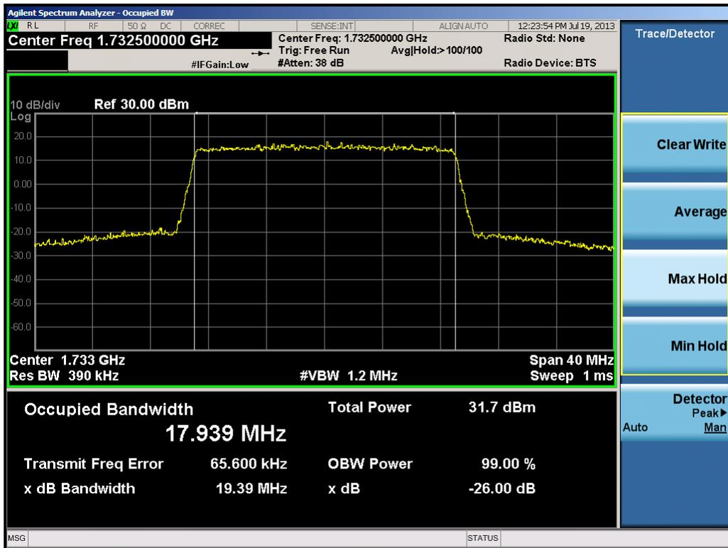
Plot 8-33. Occupied Bandwidth Plot (20.0MHz QPSK – RB Size 100)
