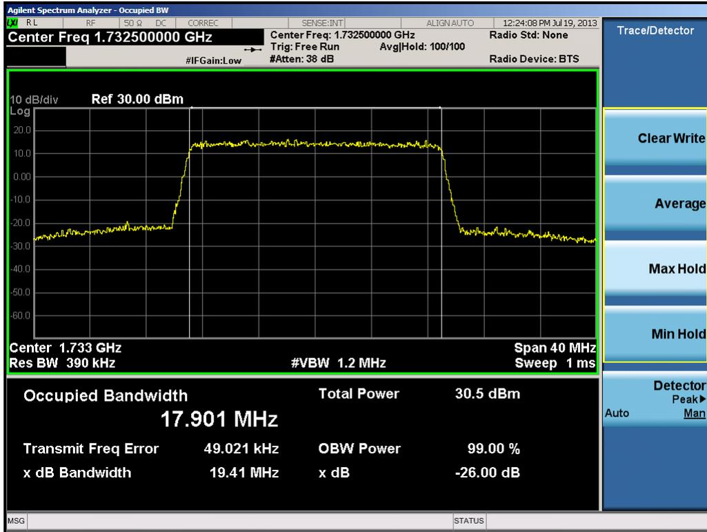
Plot 8-34. Occupied Bandwidth Plot (20.0MHz 16-QAM – RB Size 100)
