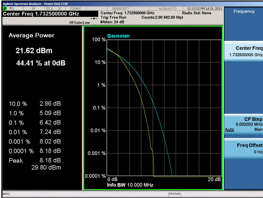
Plot 8-22. PAR Plot (10.0MHz 16-QAM – RB Size 50)
