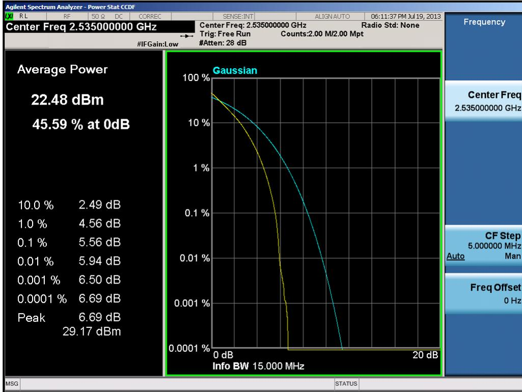
Plot 9-26. PAR Plot (15.0MHz QPSK – RB Size 75)
