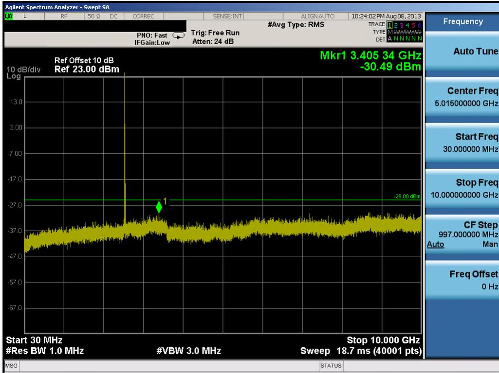
Plot 9-36. Conducted Spurious Plot (20.0MHz QPSK – RB Size 1, RB Offset 0 – High Channel)
