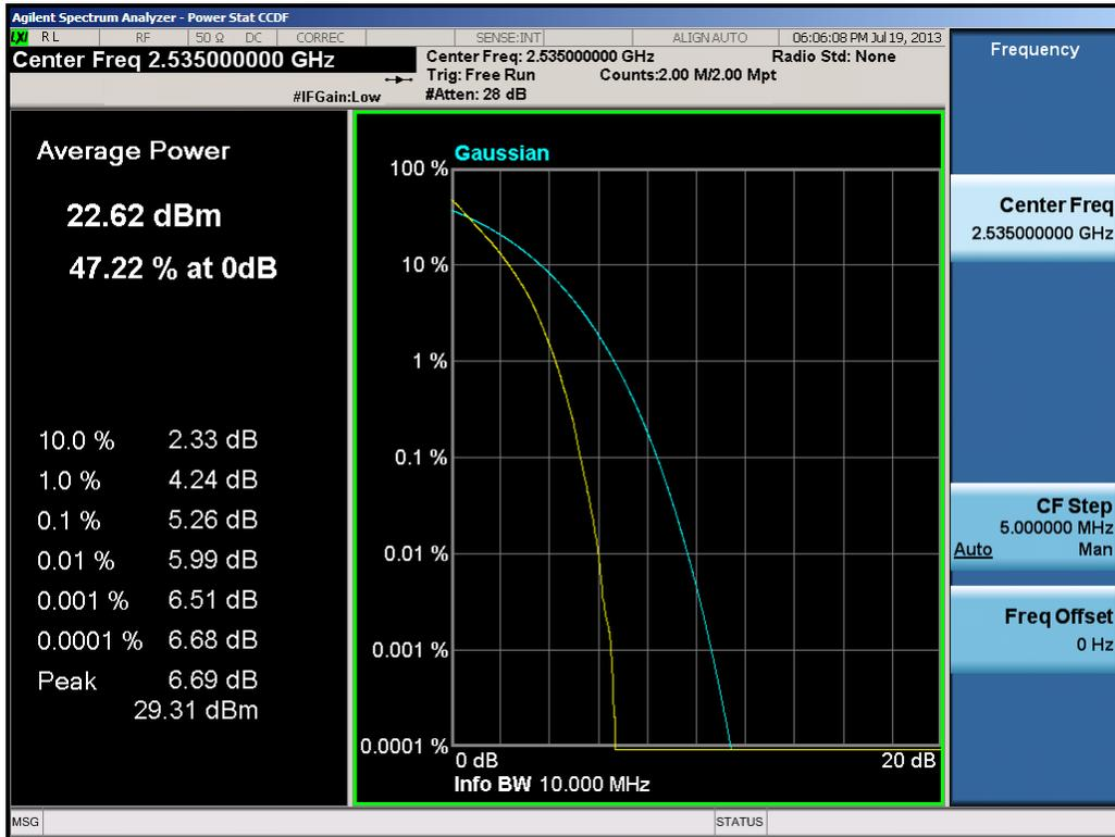
Plot 9-19. PAR Plot (10.0MHz QPSK – RB Size 50)
