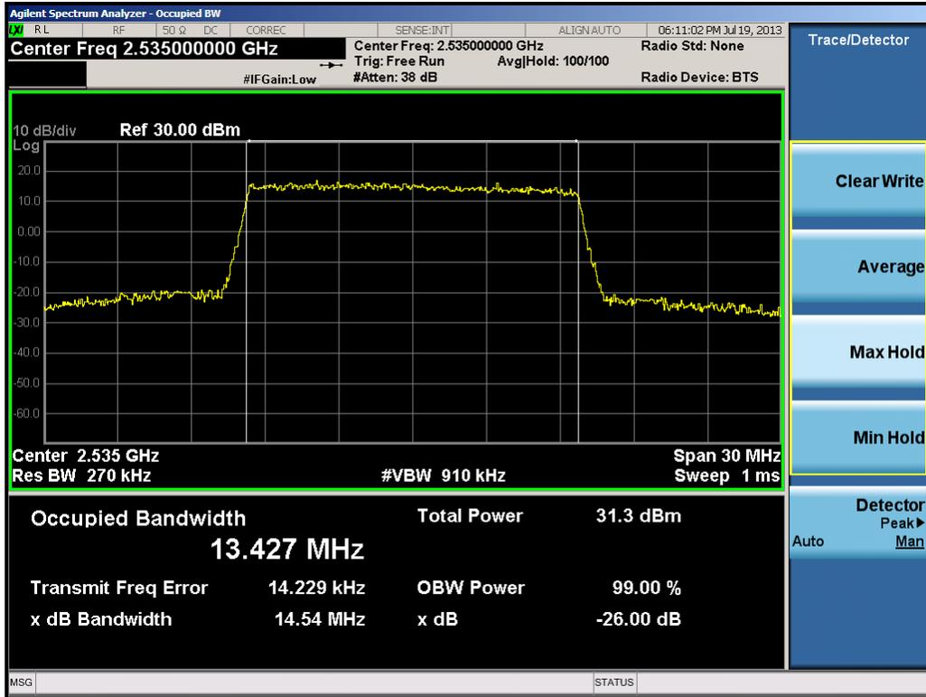
Plot 9-22. Occupied Bandwidth Plot (15.0MHz QPSK – RB Size 75)
