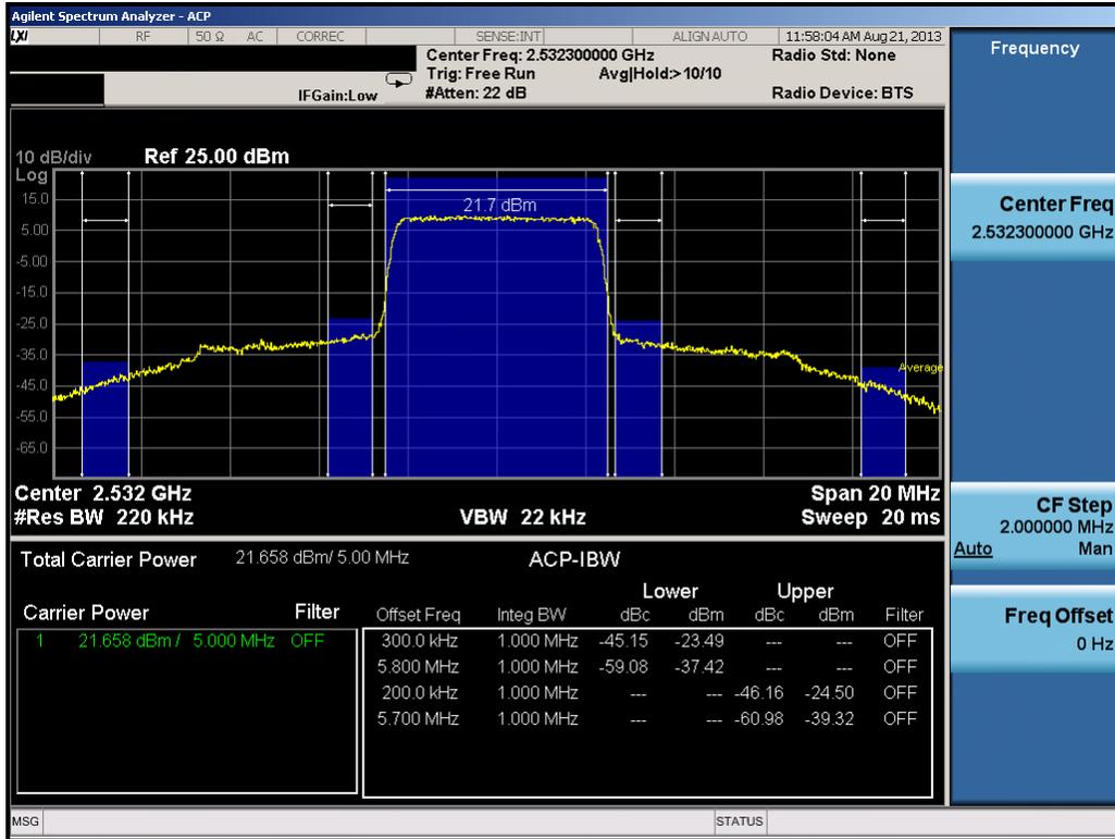
Plot 9-4. Mid Channel Adjacent Channel Power Plot (5.0MHz QPSK – RB Size 25)
