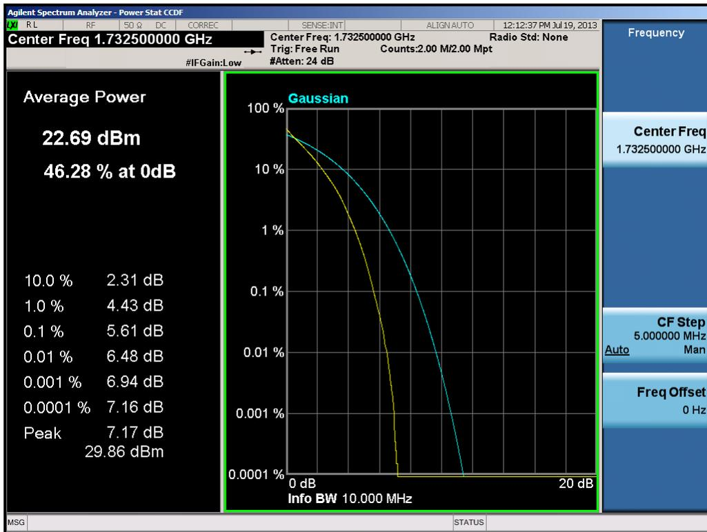
Plot 8-21. PAR Plot (10.0MHz QPSK – RB Size 50)
