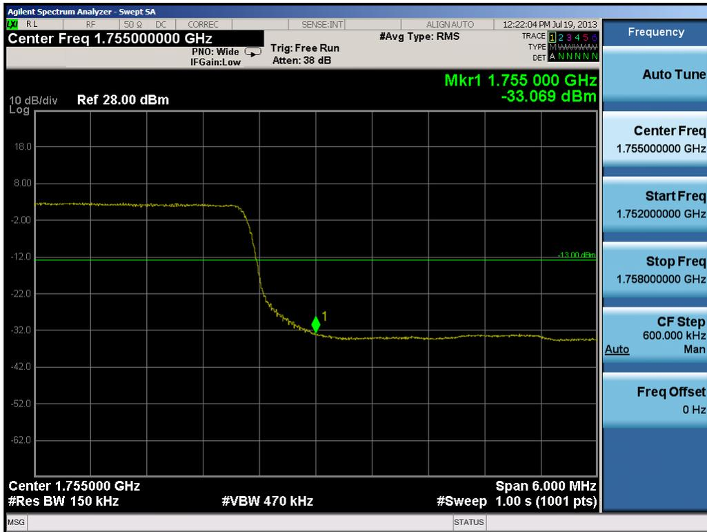
Plot 8-27. Upper Band Edge Plot (15.0MHz QPSK – RB Size 75)
