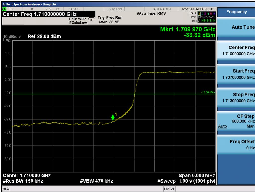
Plot 8-23. Lower Band Edge Plot (15.0MHz QPSK – RB Size 75)
