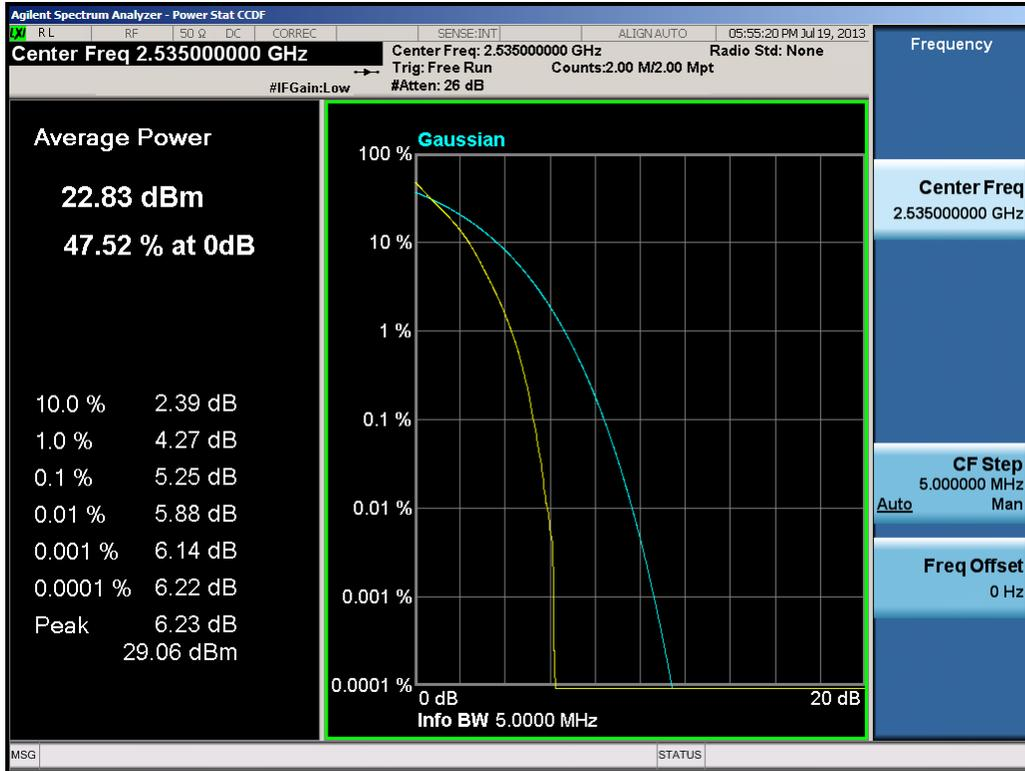
**Plot 9-12. PAR Plot (5.0MHz QPSK – RB Size 25)**
