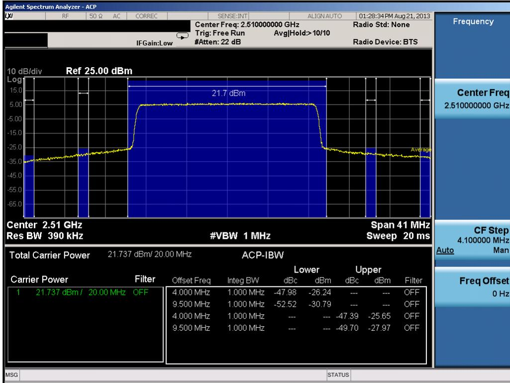
Plot 9-28. Low Channel Adjacent Channel Power Plot (20.0MHz QPSK – RB Size 100)
