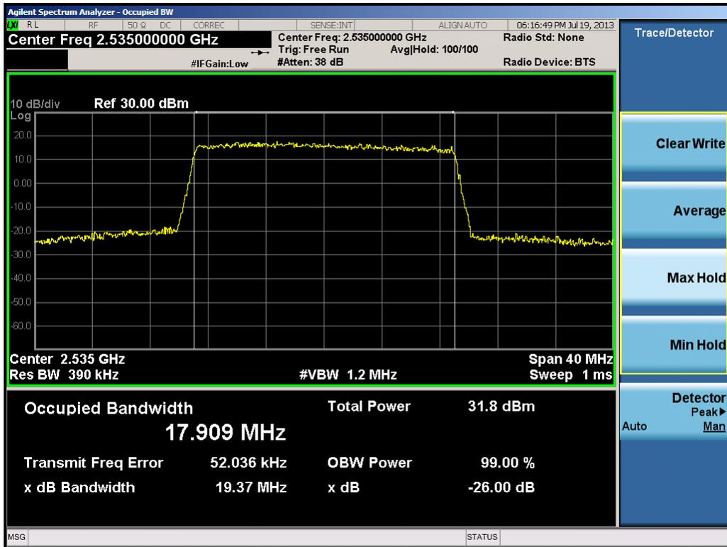
Plot 9-29. Occupied Bandwidth Plot (20.0MHz QPSK – RB Size 100)
