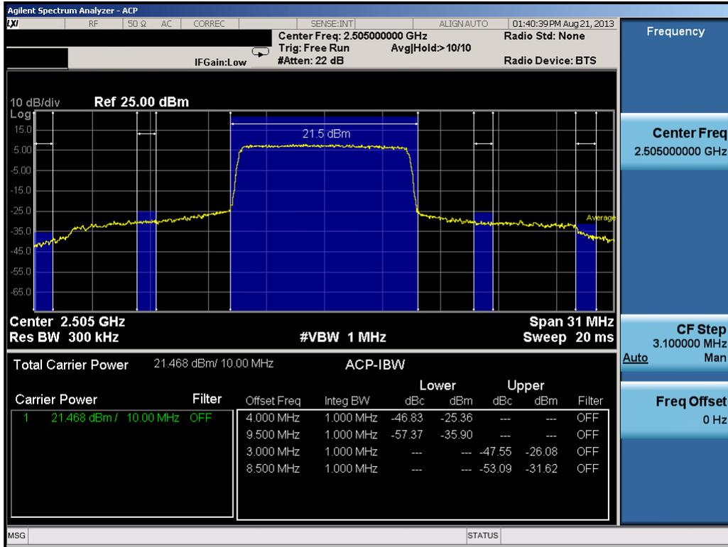
Plot 9-14. Low Channel Adjacent Channel Power Plot (10.0MHz QPSK – RB Size 50)
