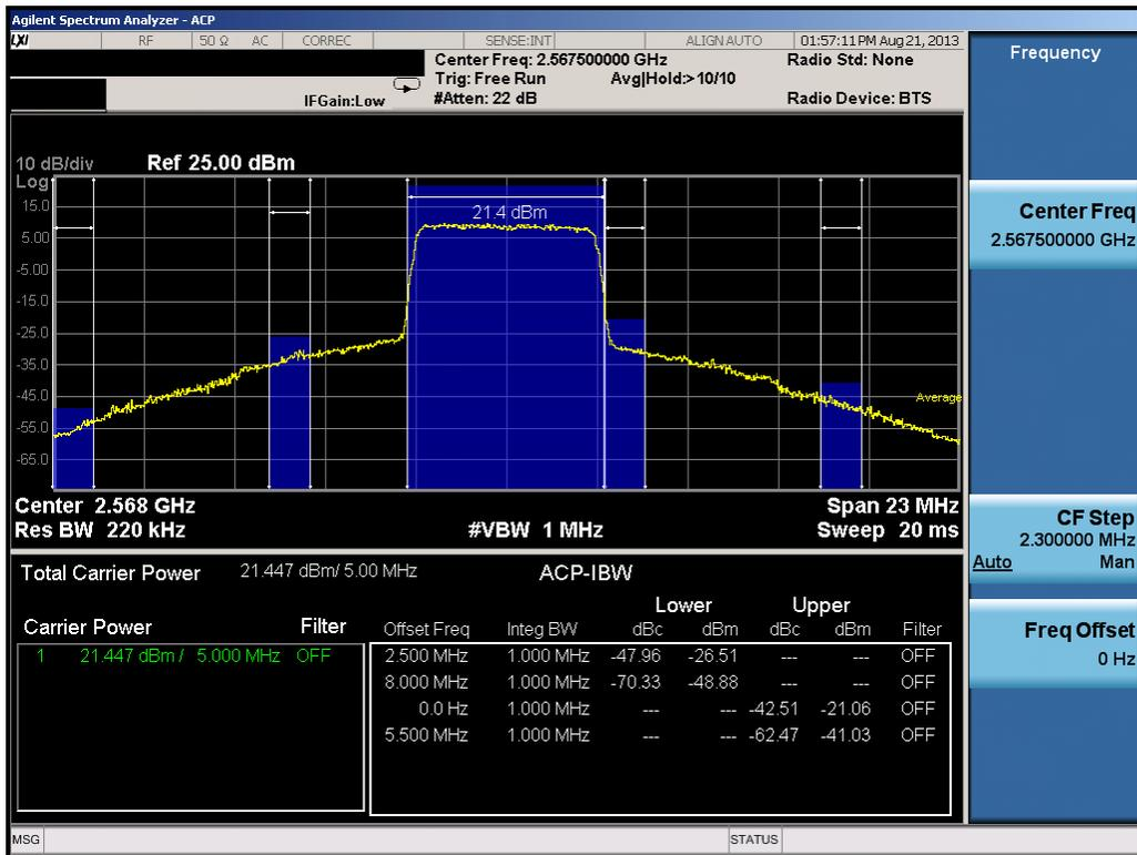
Plot 9-11. High Channel Adjacent Channel Power Plot (5.0MHz QPSK – RB Size 25)
