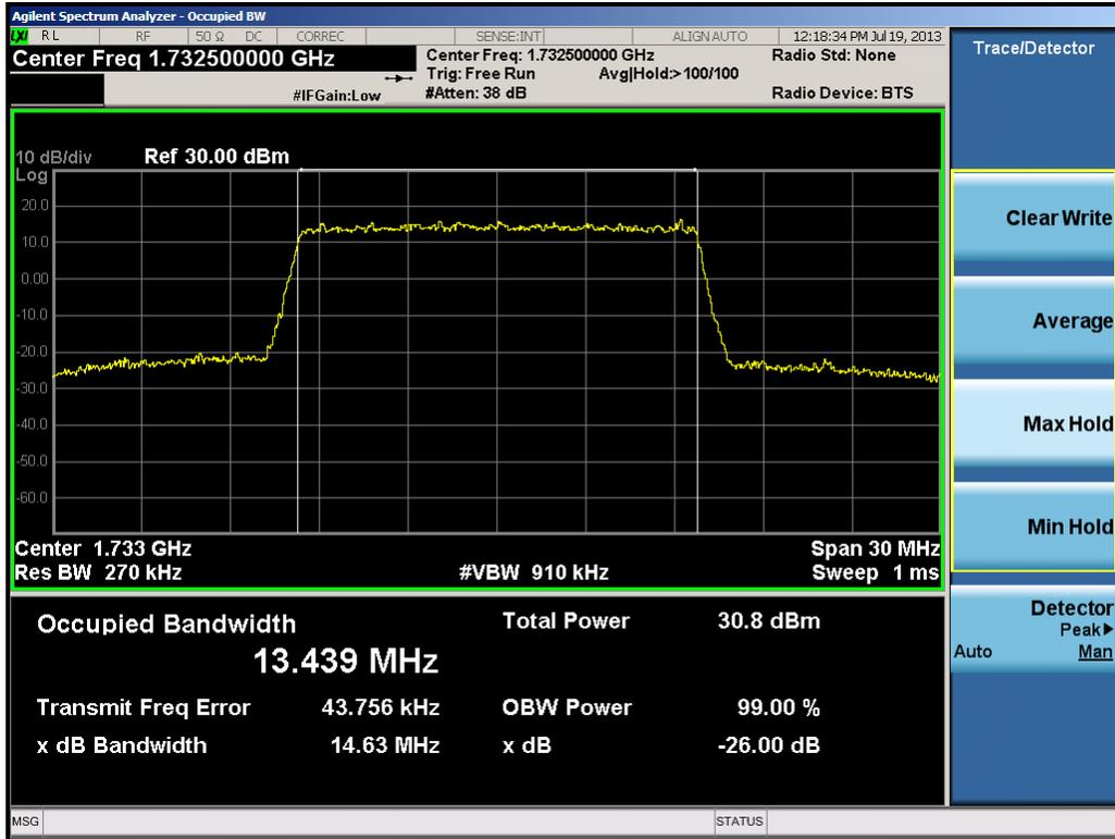
Plot 8-26. Occupied Bandwidth Plot (15.0MHz 16-QAM – RB Size 75)
