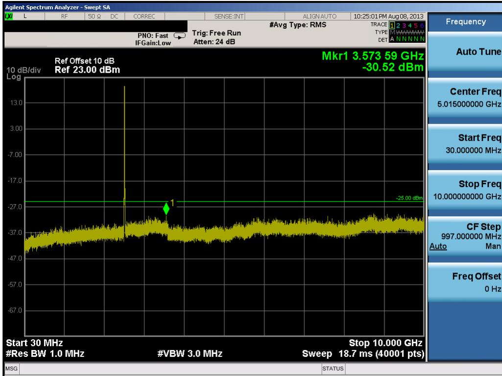
Plot 9-34. Conducted Spurious Plot (20.0MHz QPSK – RB Size 1, RB Offset 0 – Mid Channel)
