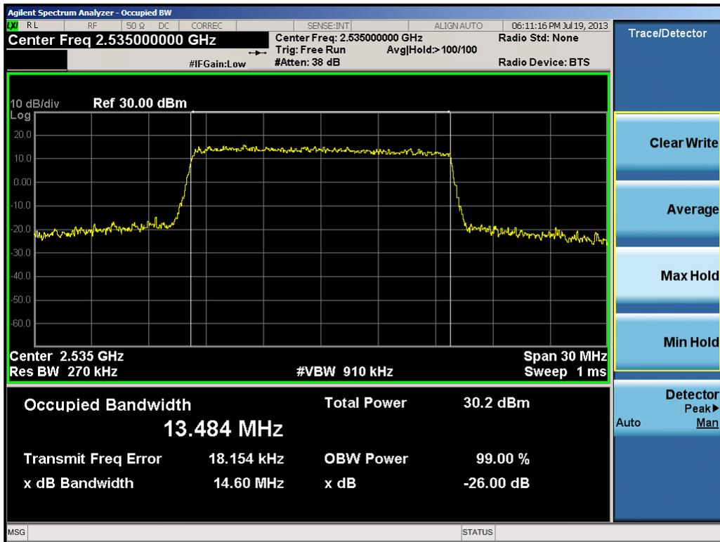
Plot 9-23. Occupied Bandwidth Plot (15.0MHz 16-QAM – RB Size 75)
