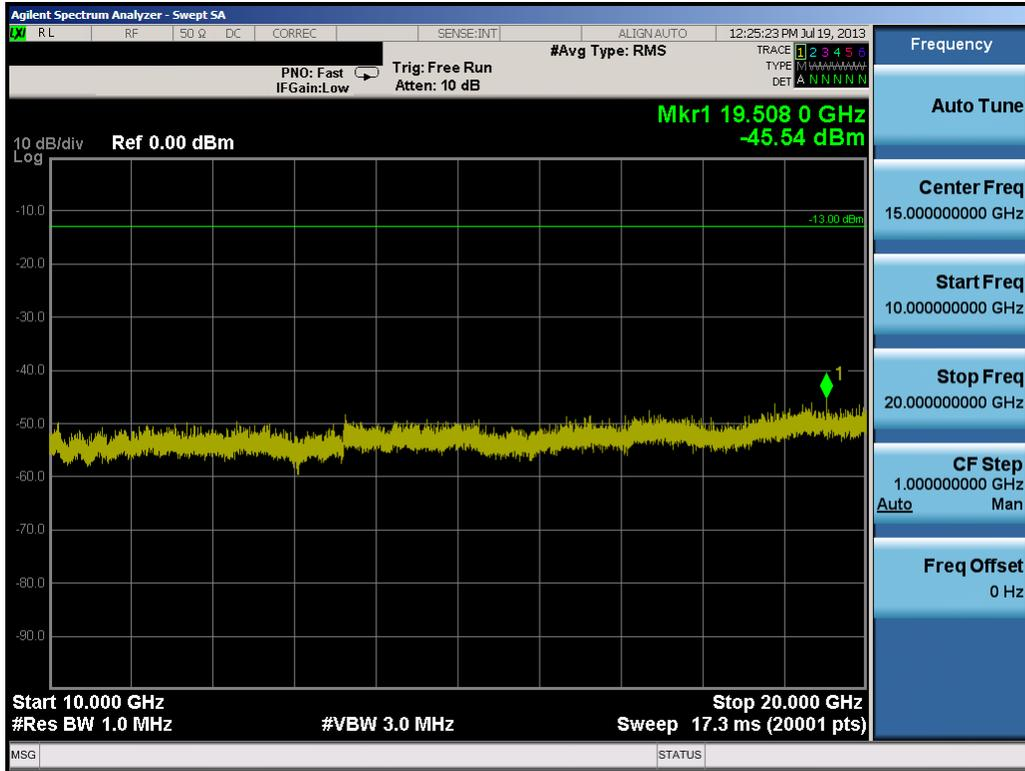
Plot 8-38. Conducted Spurious Plot (20.0MHz QPSK – RB Size 1, RB Offset 0 – Mid Channel)
