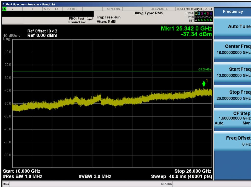
Plot 9-37. Conducted Spurious Plot (20.0MHz QPSK – RB Size 1, RB Offset 0 – High Channel)
