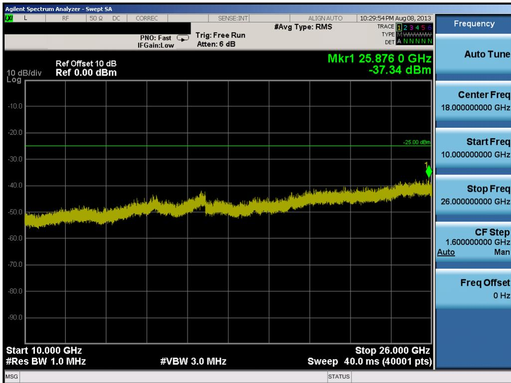
Plot 9-33. Conducted Spurious Plot (20.0MHz QPSK – RB Size 1, RB Offset 0 – Low Channel)
