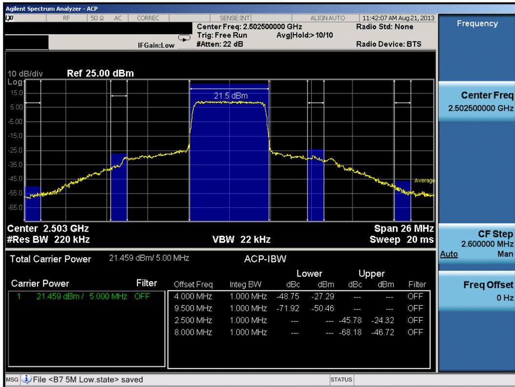
**Plot 9-1. Low Channel Adjacent Channel Power Plot (5.0MHz QPSK – RB Size 25)**
