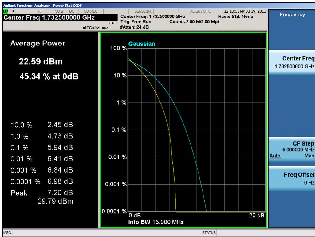
Plot 8-29. PAR Plot (15.0MHz QPSK – RB Size 75)
