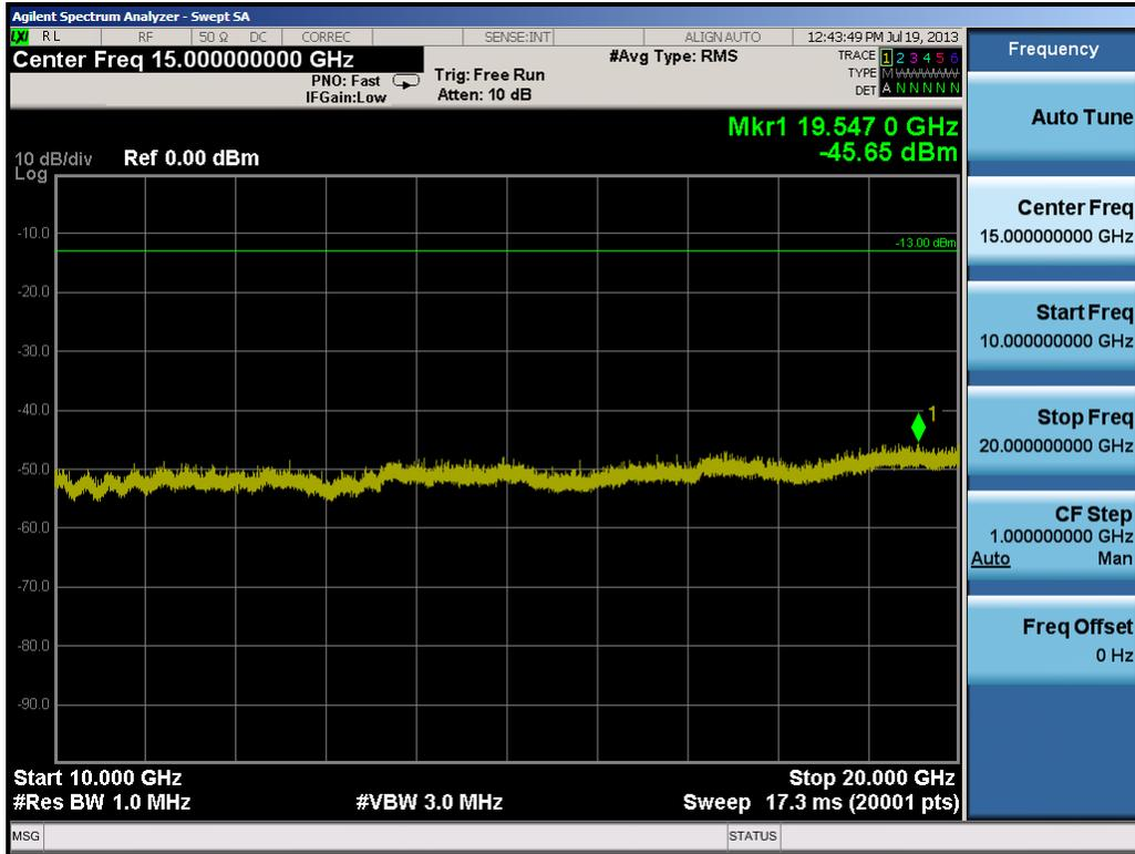
Plot 8-40. Conducted Spurious Plot (20.0MHz QPSK – RB Size 1, RB Offset 0 – High Channel)
