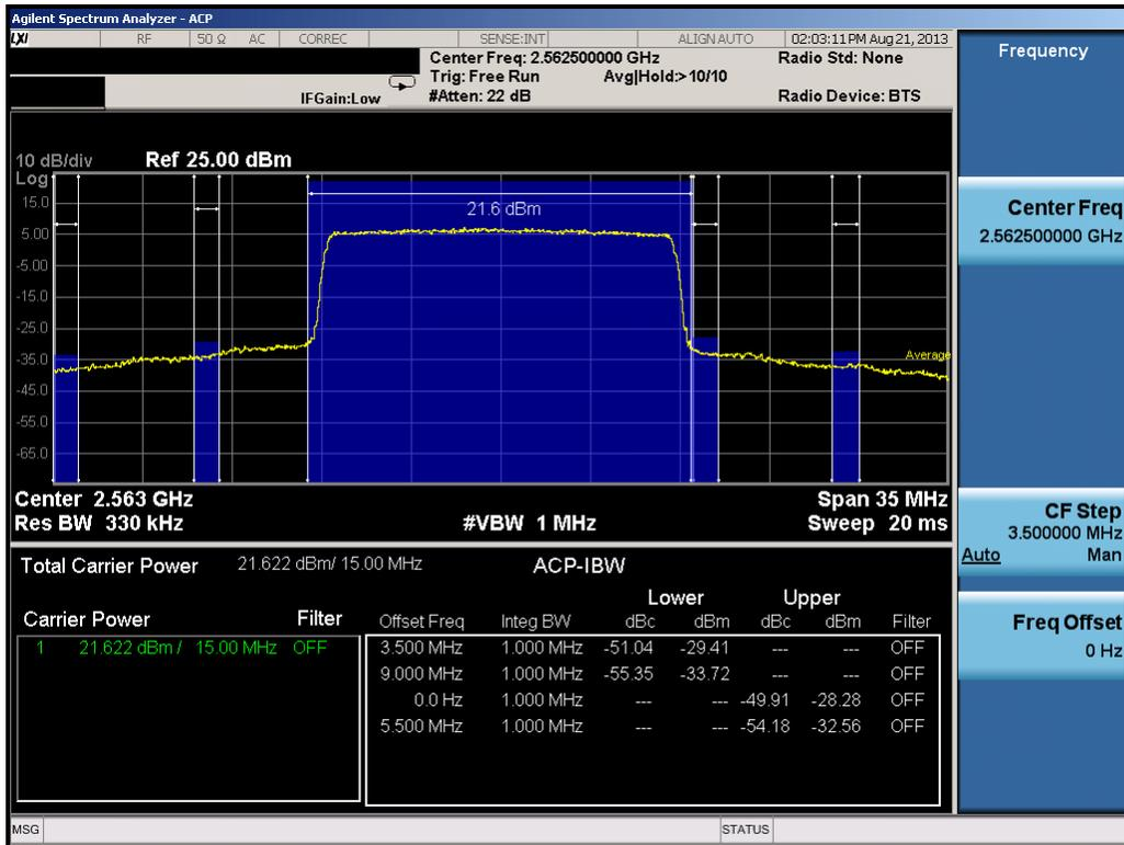
Plot 9-25. High Channel Adjacent Channel Power Plot (15.0MHz QPSK – RB Size 75)
