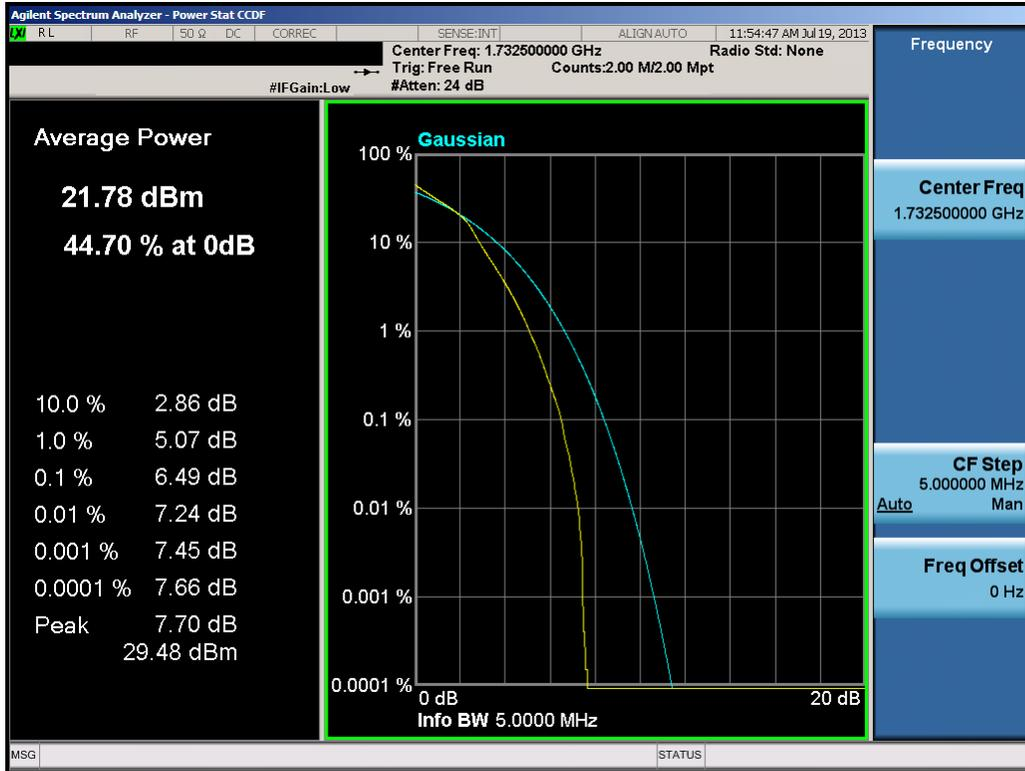
Plot 8-14. PAR Plot (5.0MHz 16-QAM – RB Size 25)
