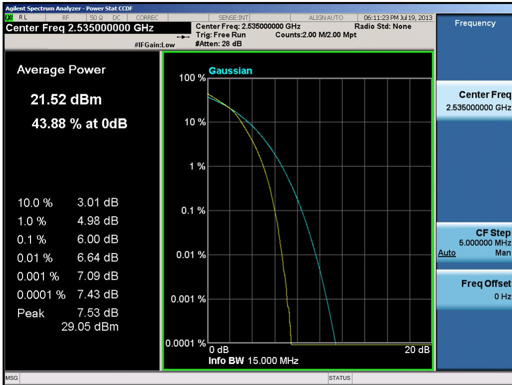
Plot 9-27. PAR Plot (15.0MHz 16-QAM – RB Size 75)
