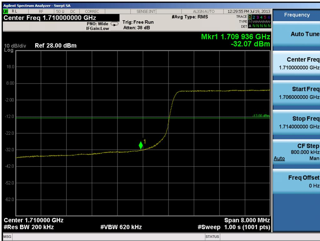
Plot 8-31. Lower Band Edge Plot (20.0MHz QPSK – RB Size 100)
