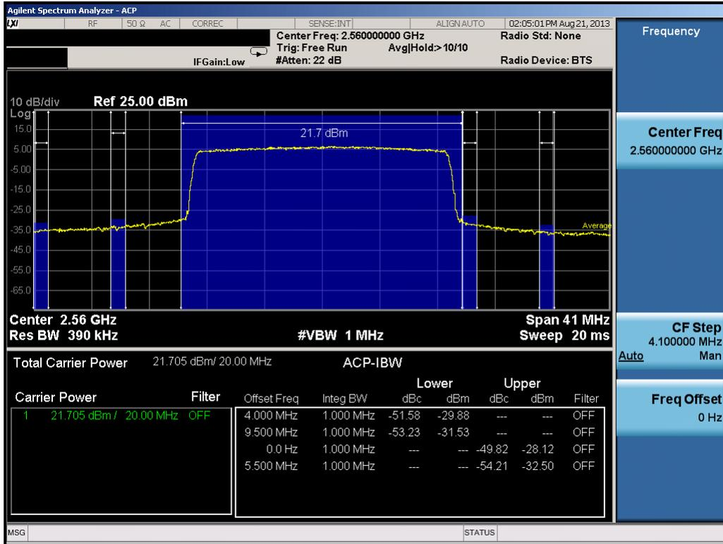
Plot 9-38. High Channel Adjacent Channel Power Plot (20.0MHz QPSK – RB Size 100)
