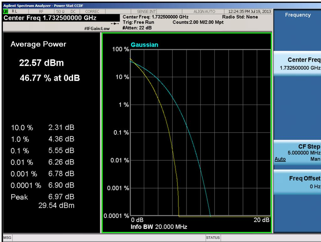
Plot 8-43. PAR Plot (20.0MHz QPSK – RB Size 100)
