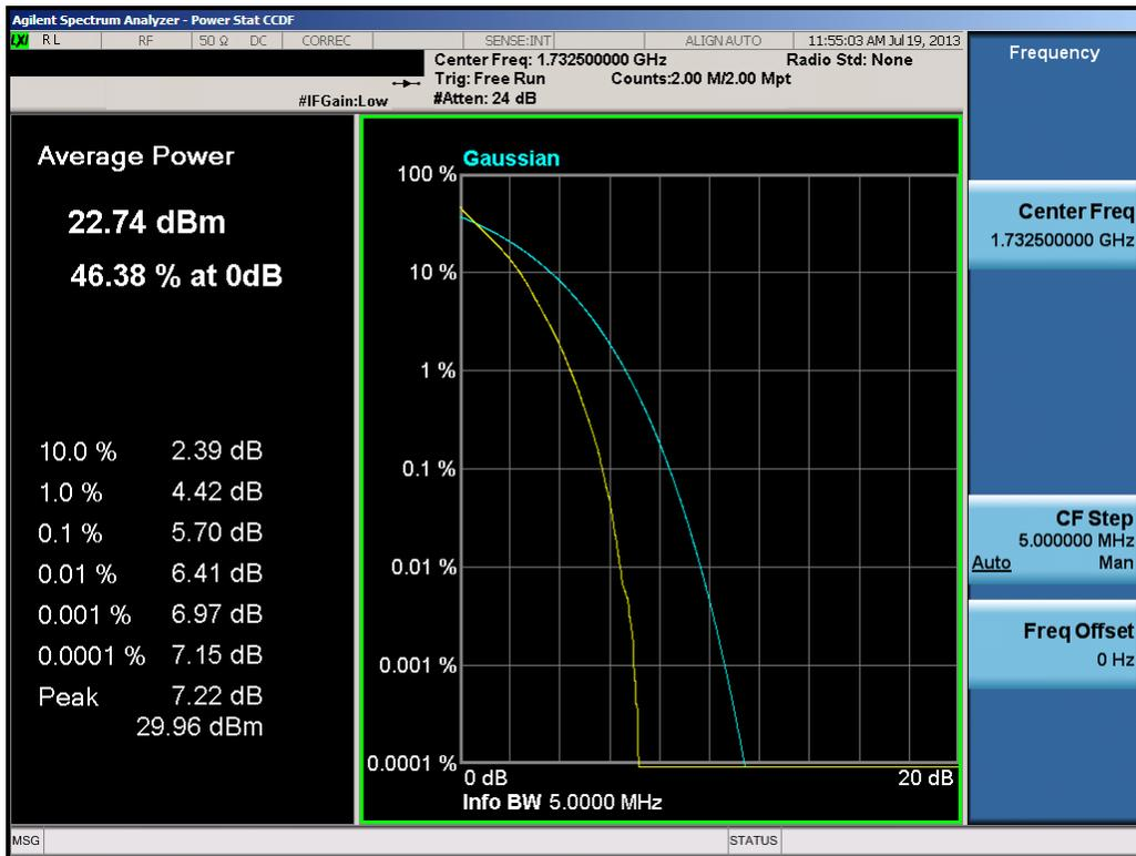
Plot 8-13. PAR Plot (5.0MHz QPSK – RB Size 25)
