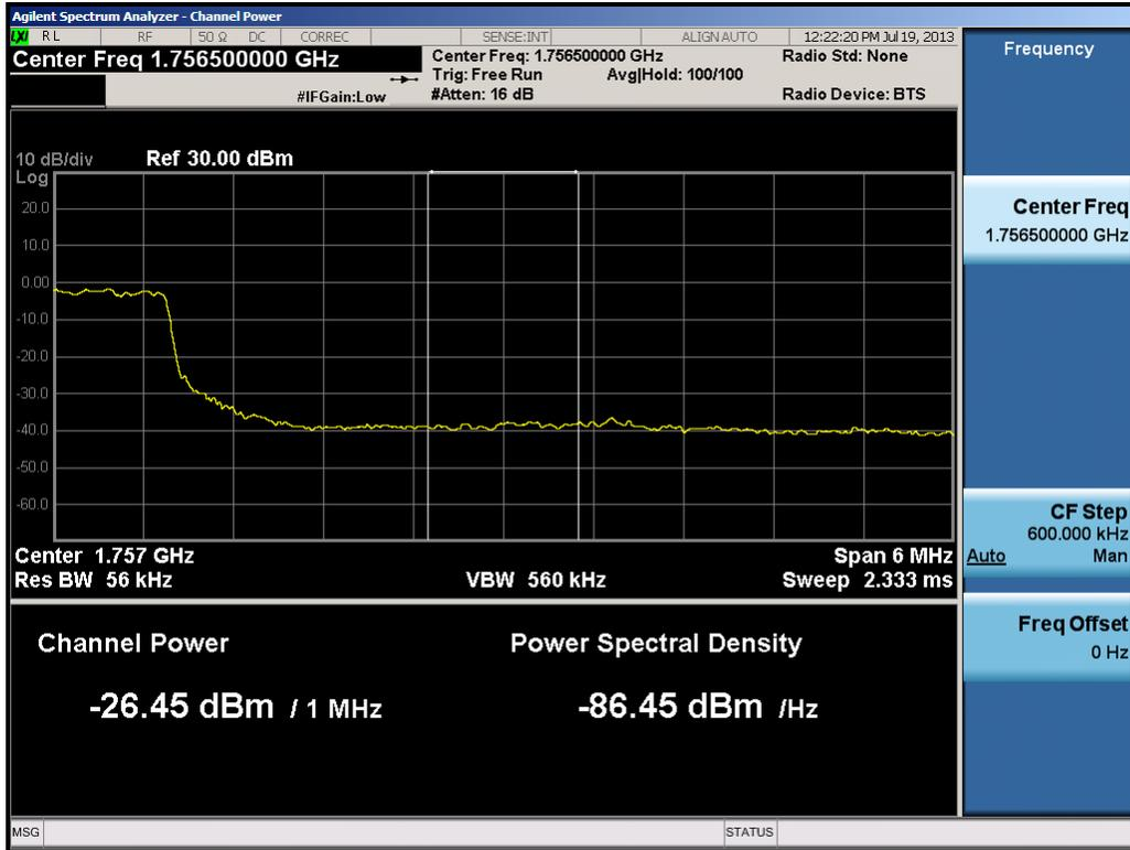
Plot 8-28. Upper Extended Band Edge Plot (15.0MHz QPSK – RB Size 75)
