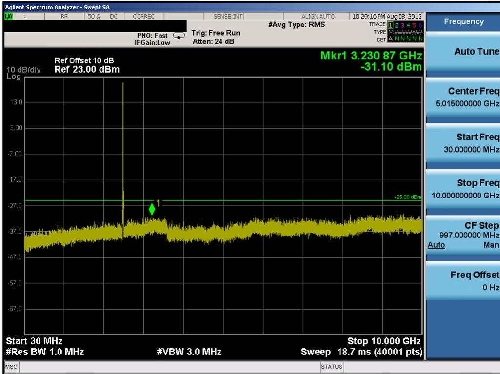
Plot 9-32. Conducted Spurious Plot (20.0MHz QPSK – RB Size 1, RB Offset 0– Low Channel)
