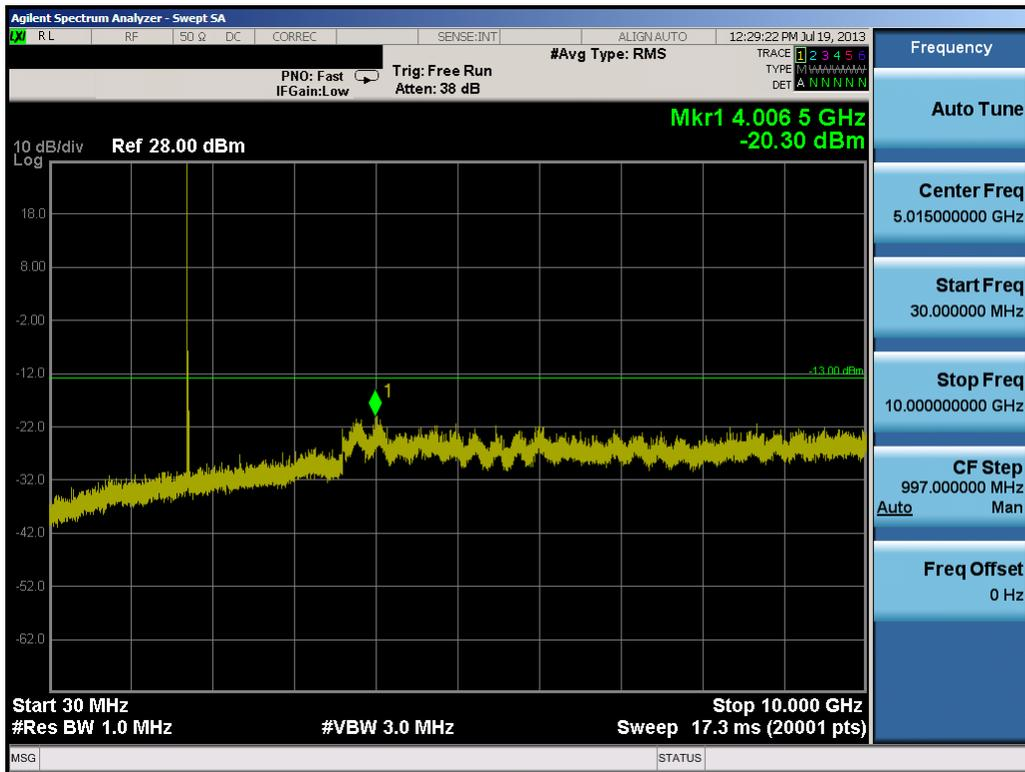
Plot 8-35. Conducted Spurious Plot (20.0MHz QPSK – RB Size 1, RB Offset 0– Low Channel)
