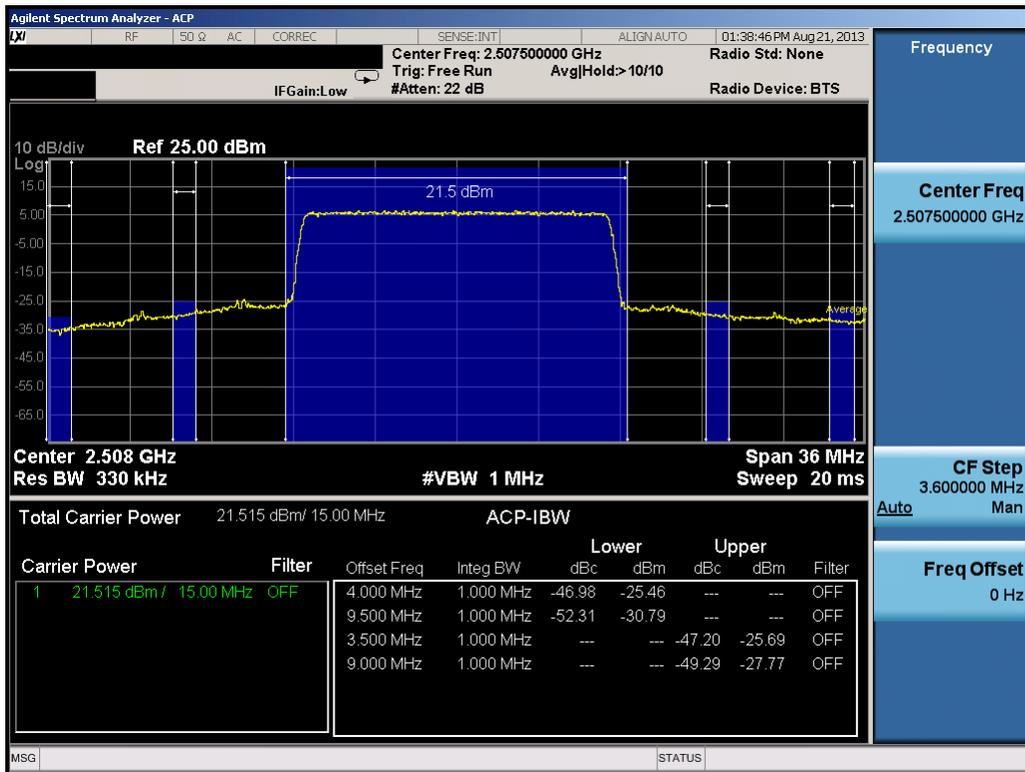
Plot 9-21. Low Channel Adjacent Channel Power Plot (15.0MHz QPSK – RB Size 75)
