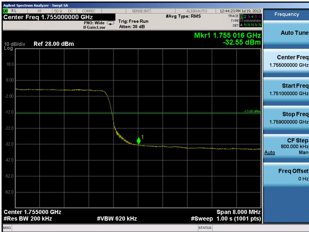
Plot 8-41. Upper Band Edge Plot (20.0MHz QPSK – RB Size 100)
