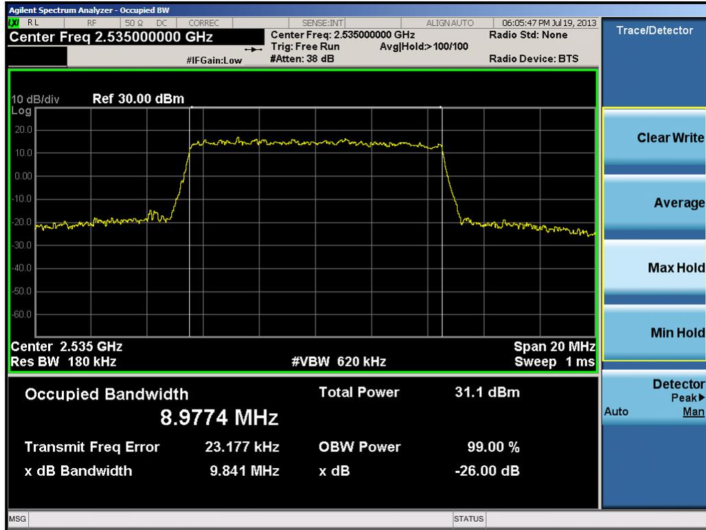
Plot 9-16. Occupied Bandwidth Plot (10.0MHz 16-QAM – RB Size 50)
