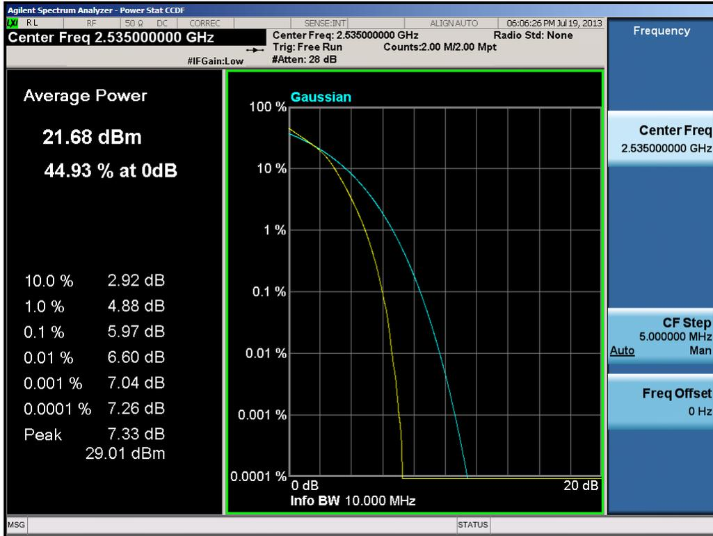
Plot 9-20. PAR Plot (10.0MHz 16-QAM – RB Size 50)
