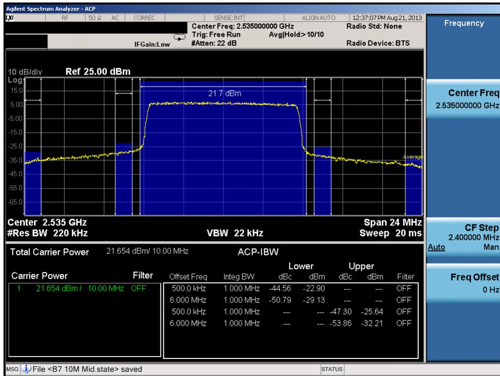
Plot 9-17. Mid Channel Adjacent Channel Power Plot (10.0MHz QPSK – RB Size 50)
