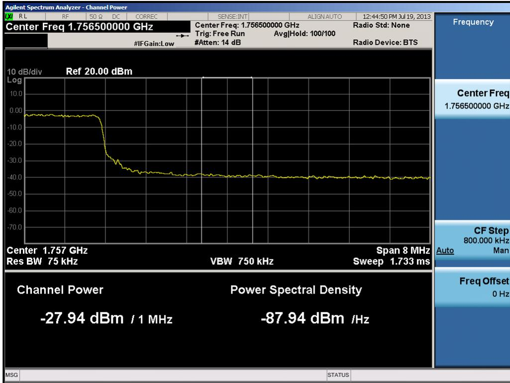
Plot 8-42. Upper Extended Band Edge Plot (20.0MHz QPSK – RB Size 100)
