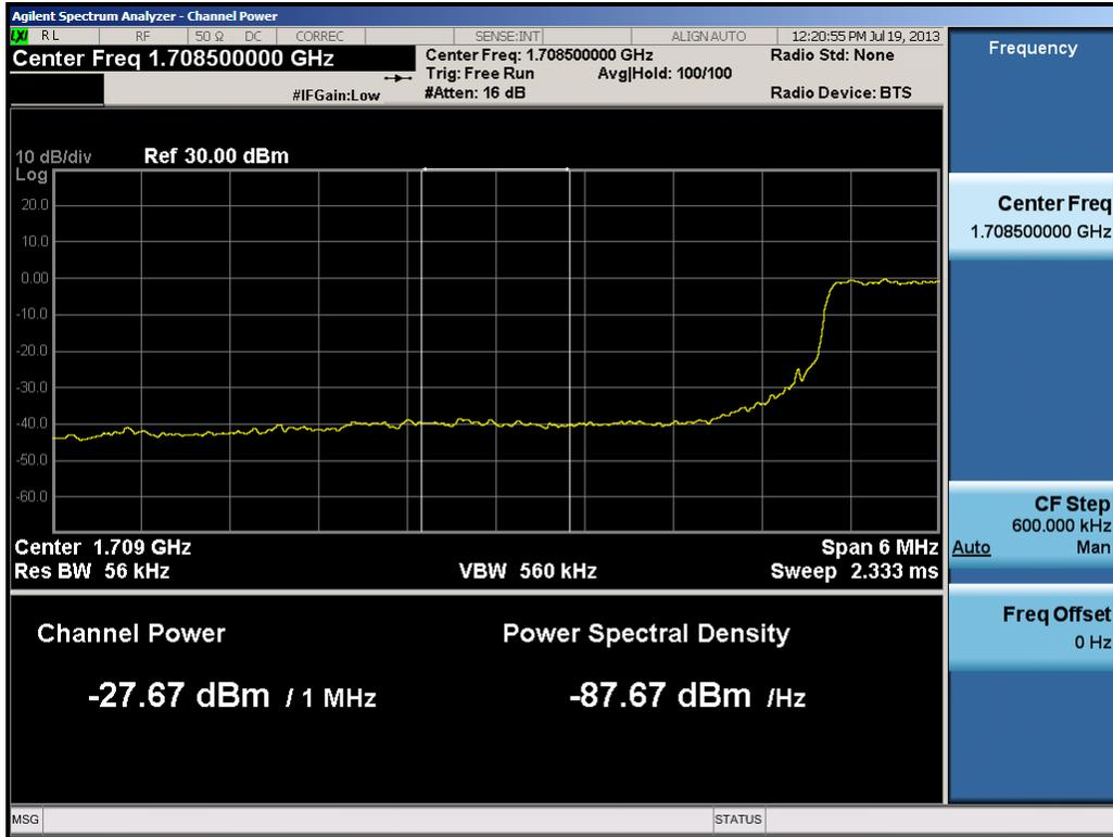
Plot 8-24. Lower Extended Band Edge Plot (15.0MHz QPSK – RB Size 75)
