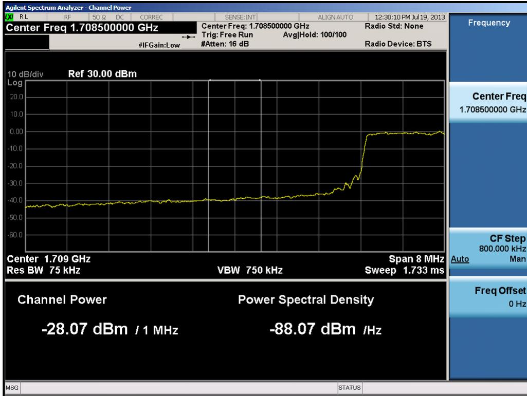
Plot 8-32. Lower Extended Band Edge Plot (20.0MHz QPSK – RB Size 100)
