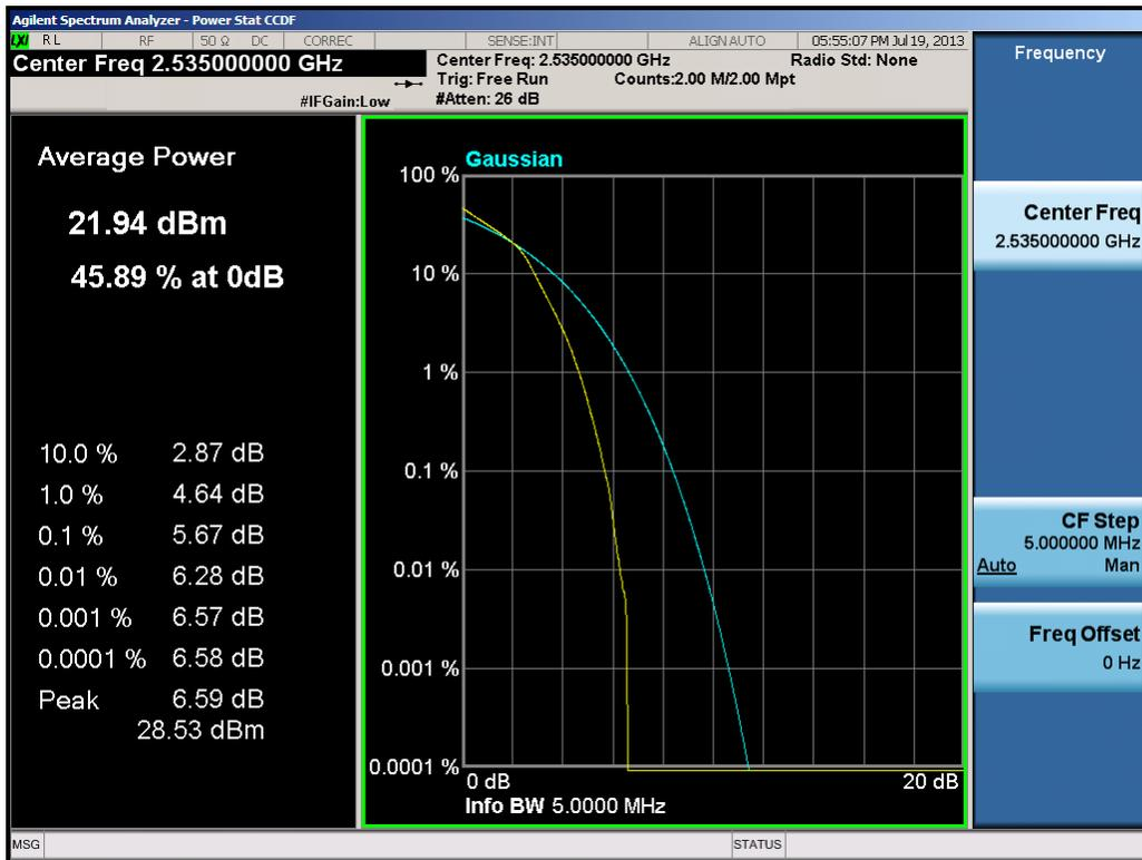
**Plot 9-13. PAR Plot (5.0MHz 16-QAM – RB Size 25)**
