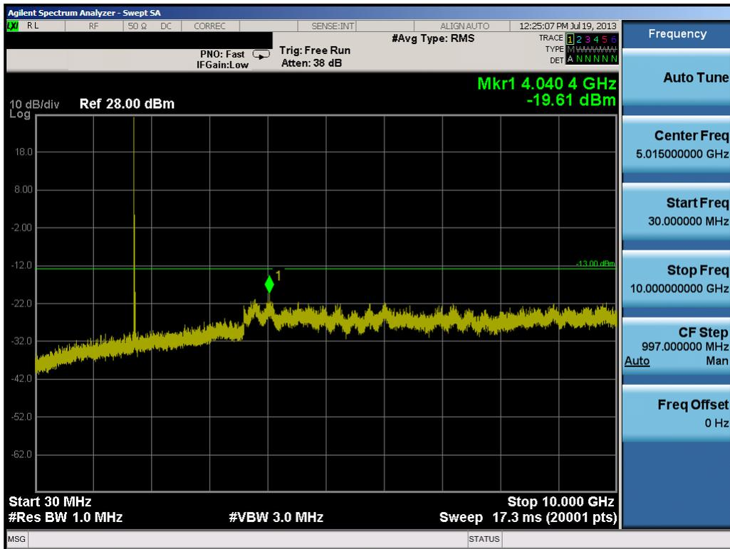
Plot 8-37. Conducted Spurious Plot (20.0MHz QPSK – RB Size 1, RB Offset 0 – Mid Channel)
