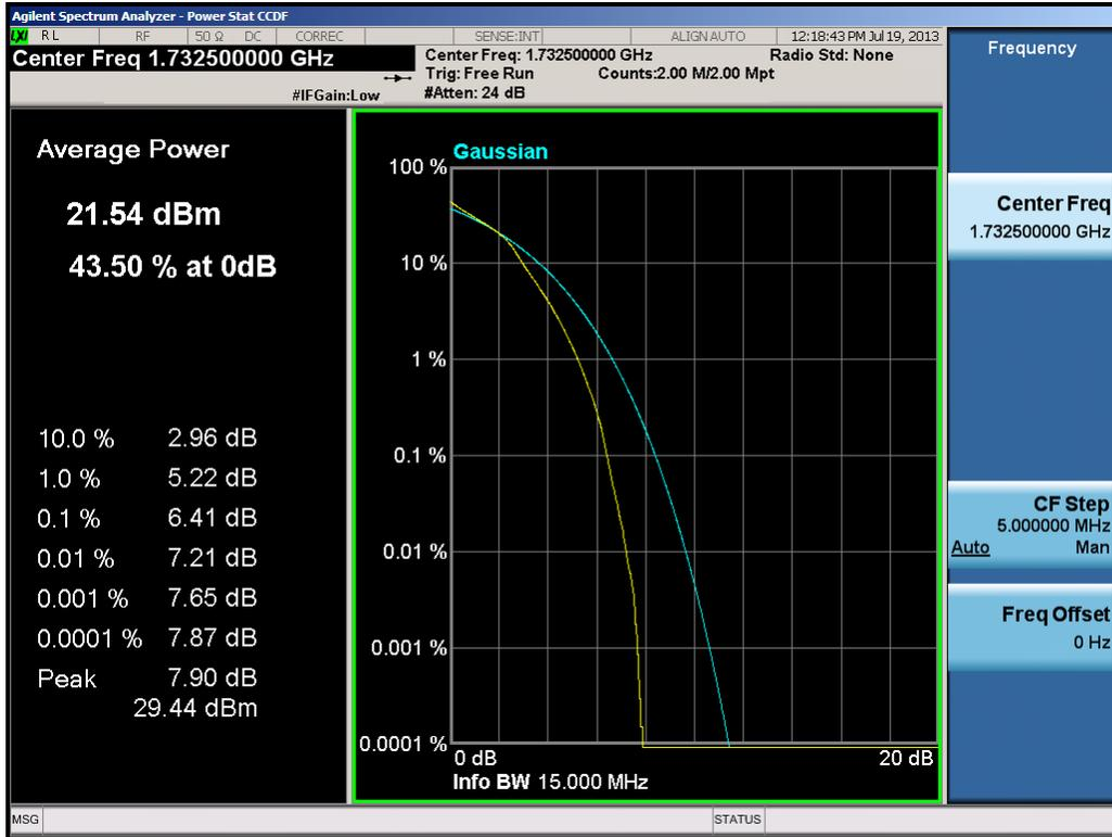
Plot 8-30. PAR Plot (15.0MHz 16-QAM – RB Size 75)
