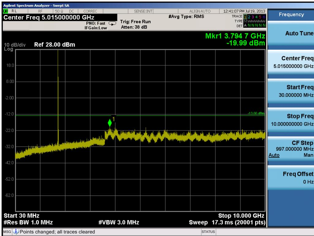
Plot 8-39. Conducted Spurious Plot (20.0MHz QPSK – RB Size 1, RB Offset 0 – High Channel)
