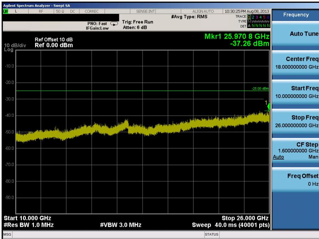
Plot 9-35. Conducted Spurious Plot (20.0MHz QPSK – RB Size 1, RB Offset 0 – Mid Channel)
