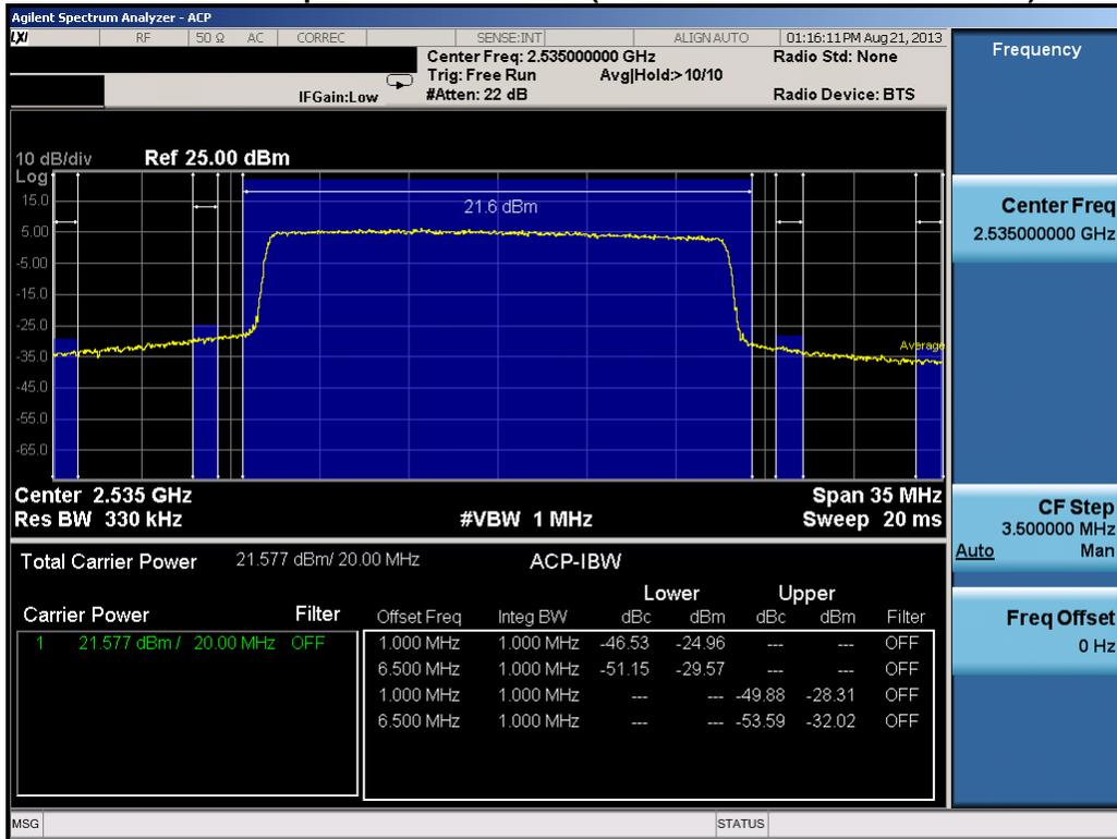
Plot 9-31. Mid Channel Adjacent Channel Power Plot (20.0MHz QPSK – RB Size 100)
