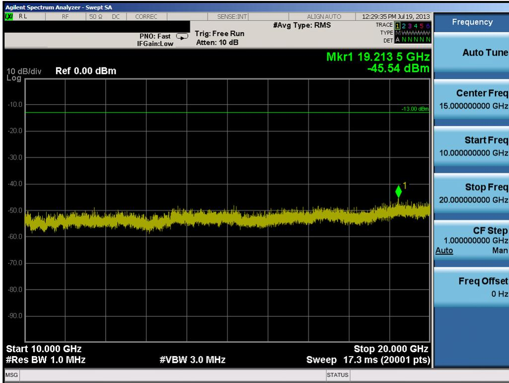
Plot 8-36. Conducted Spurious Plot (20.0MHz QPSK – RB Size 1, RB Offset 0 – Low Channel)
