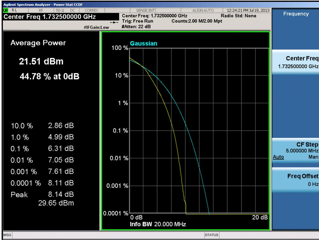
**Plot 8-44. PAR Plot (20.0MHz 16-QAM – RB Size 100)**
