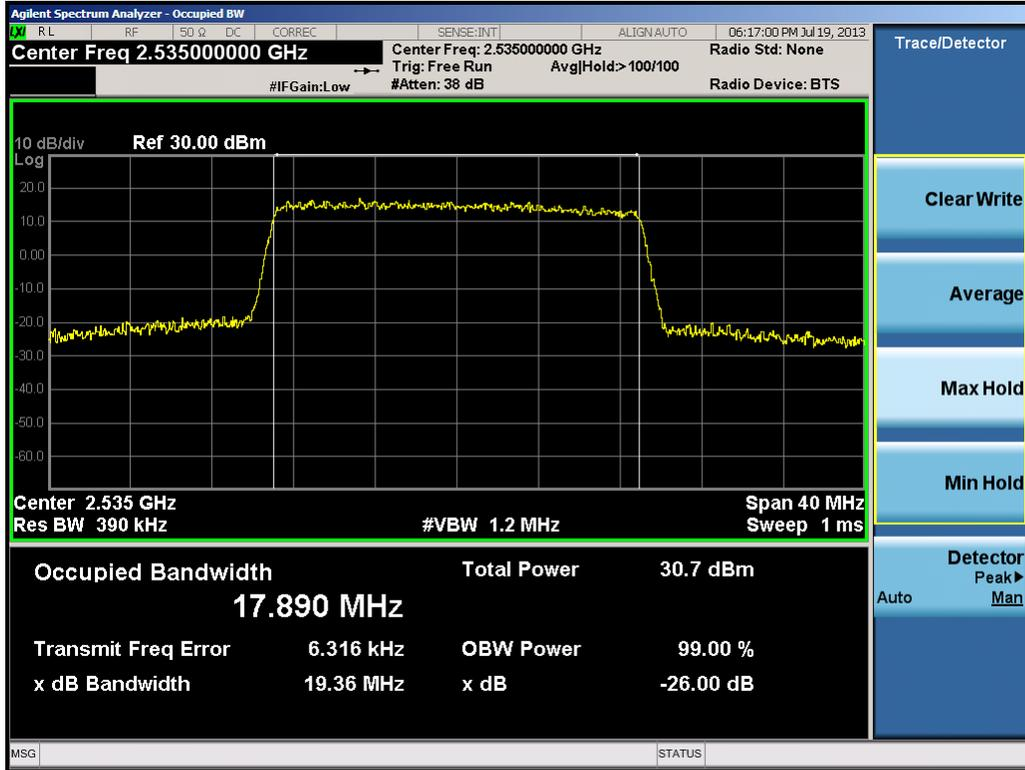
Plot 9-30. Occupied Bandwidth Plot (20.0MHz 16-QAM – RB Size 100)
