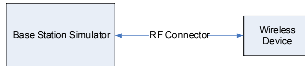
Figure 9-1 Power Measurement Setup
