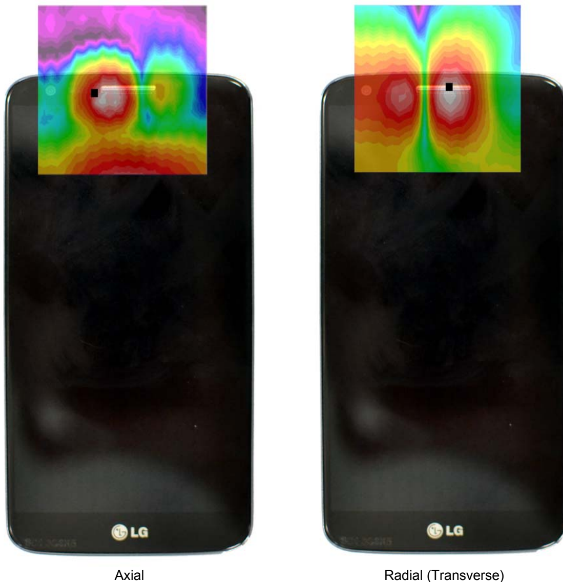
Figure 13-3 T-Coil Scan Overlay Magnetic Field Distributions
