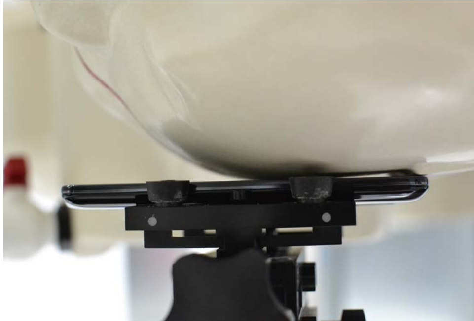
SAR Test Setup Photo 3: Left Cheek
