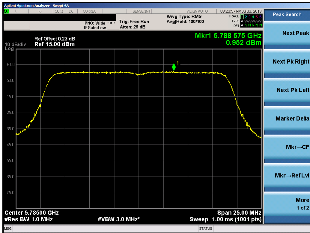
Plot 6-71. Peak Power Spectral Density Plot (20MHz BW 802.11n (UNII Band 4) – Ch. 157)
