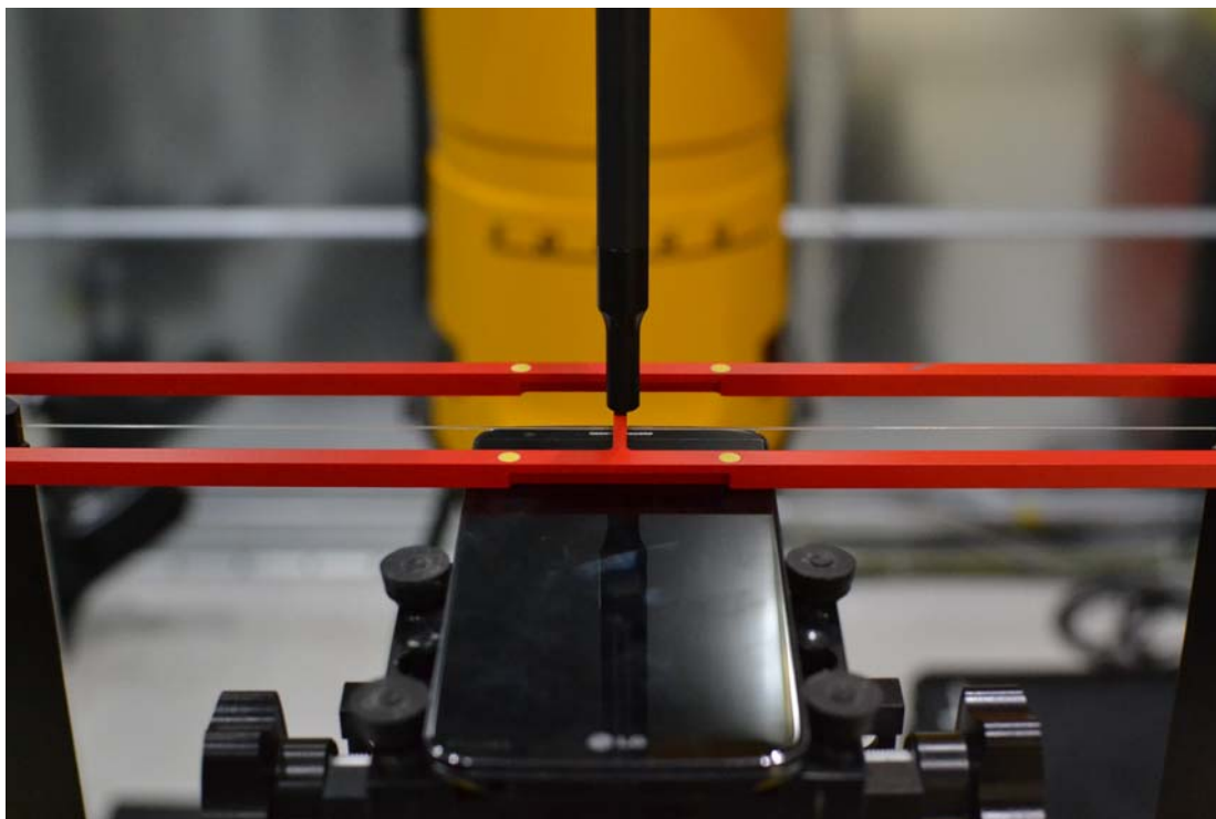
Figure 18-1 Ear Reference Point HAC Phantom Alignment
