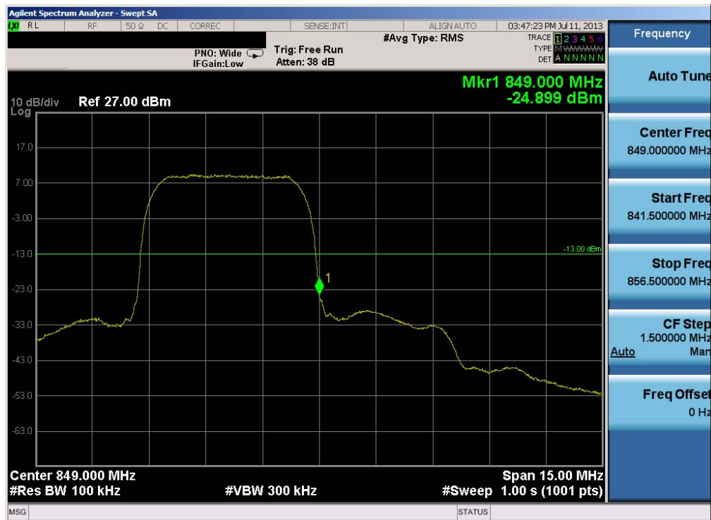
Plot 6-39. Band Edge Plot (Cellular WCDMA Mode – Ch. 4233)
