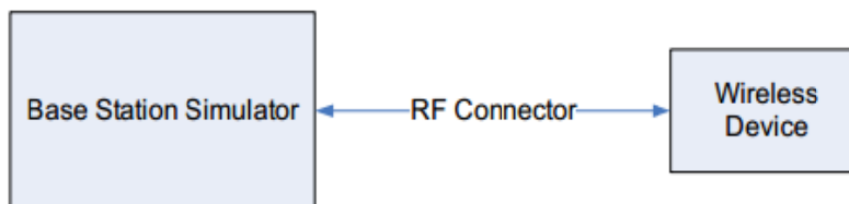
Figure 10.2 Power Measurement Setup
