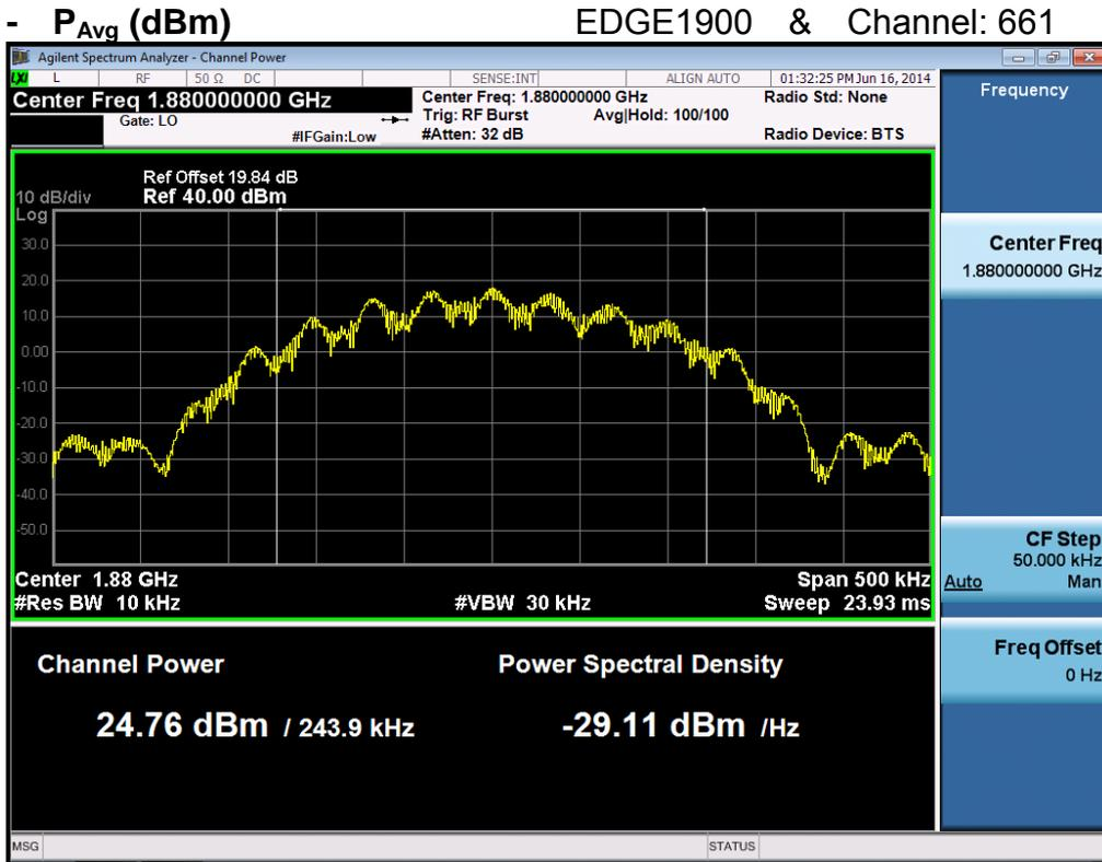
$$PAPR (dB) = P_{Pk} (dBm) - P_{Avg} (dBm) = 28.34 \text{ dBm} - 24.76 \text{ dBm} = 3.58 \text{ dB}$$
