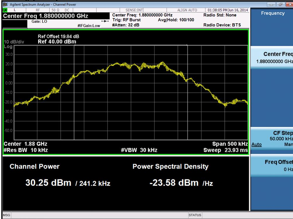
$$PAPR (dB) = P_{Pk} (dBm) - P_{Avg} (dBm) = 30.425dBm - 30.250dBm = 0.175 dB$$
