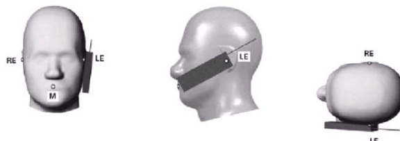
Figure 7.1 Front, Side and Top View of Cheek/Touch Position
