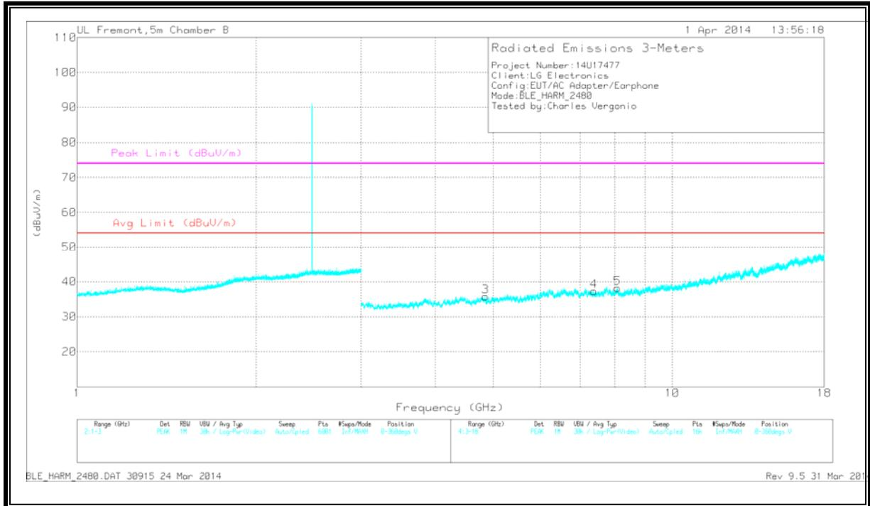
Note: Emission was scanned up to 26GHz; No emissions were detected above the noise floor which was at least 20dB below the specification limit.
