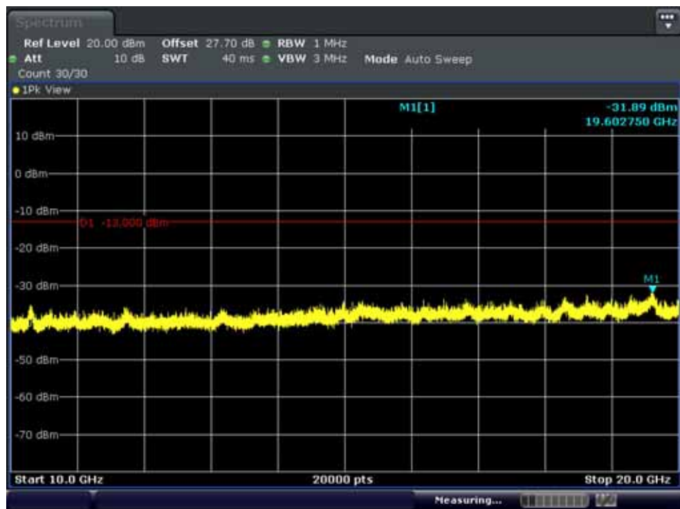
Band 4: Conducted Spurious Plot 2 (1.4MHz QPSK - RB Size 1, RB Offset 0 - Mid Band 4: Channel)
