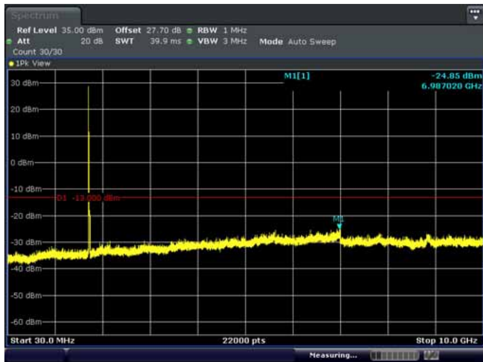
Band 4: Conducted Spurious Plot 1 (15MHz QPSK - RB Size 1, RB Offset 0 - Mid Band 4: Channel)
