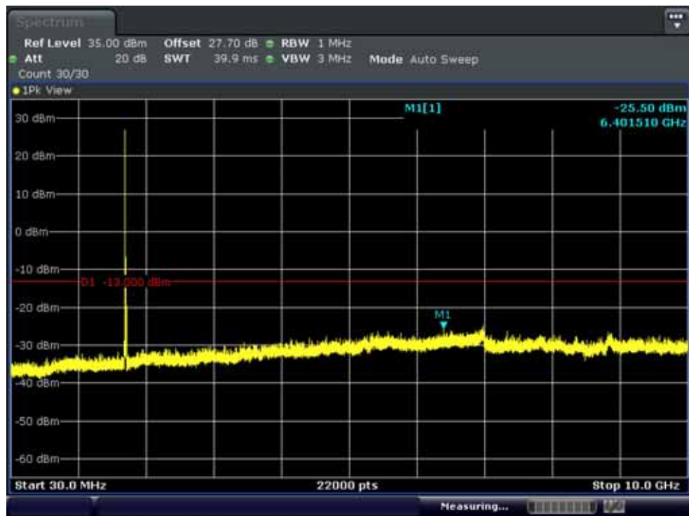
Band 4: Conducted Spurious Plot 1 (10MHz QPSK - RB Size 1, RB Offset 0 - Low Band 4: Channel)
