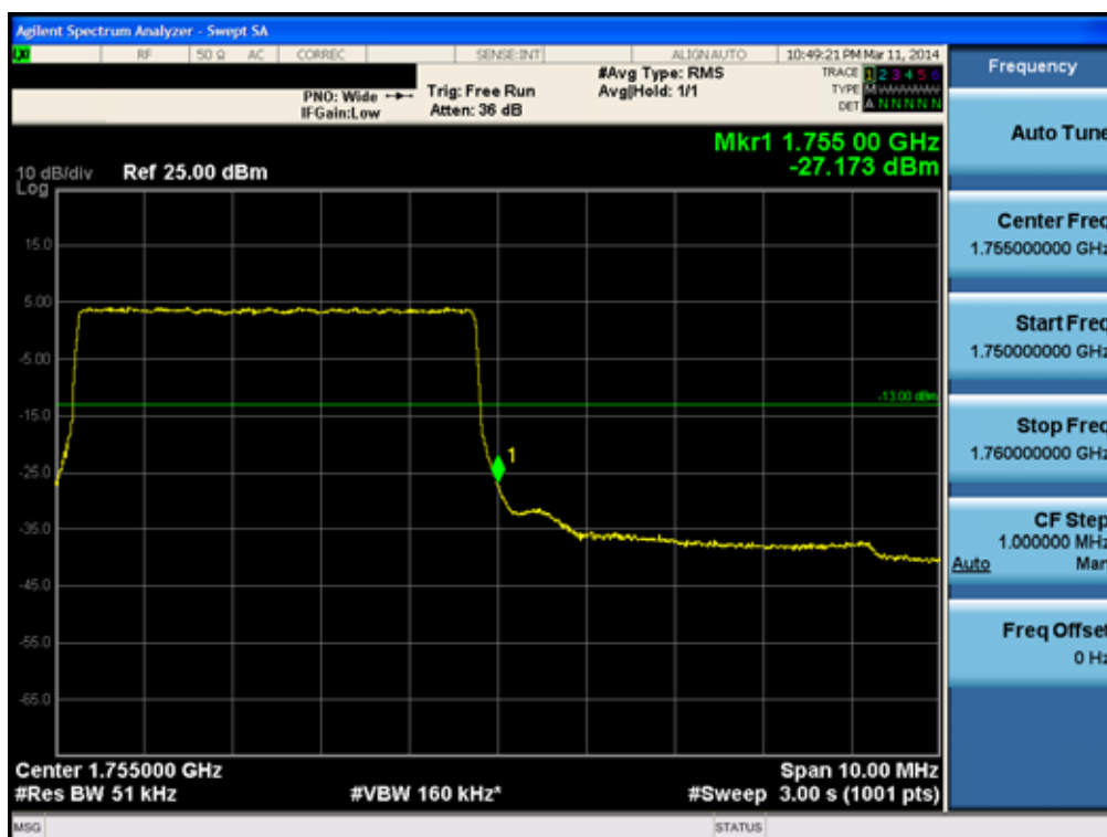
Upper Band Edge Plot (5M BW Ch.20375 QPSK RB 25) -2
