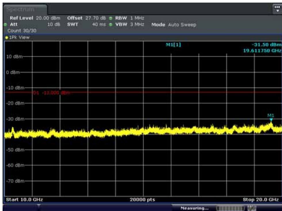
Band 4: Conducted Spurious Plot 2 (5MHz QPSK - RB Size 1, RB Offset 0 - Low Band 4: Channel)
