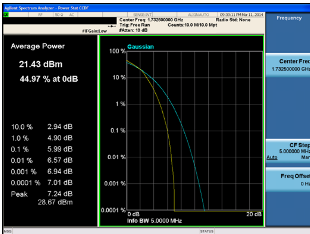
Peak to Average Ratio Plot (5M BW Ch.20175 16QAM RB 25)
