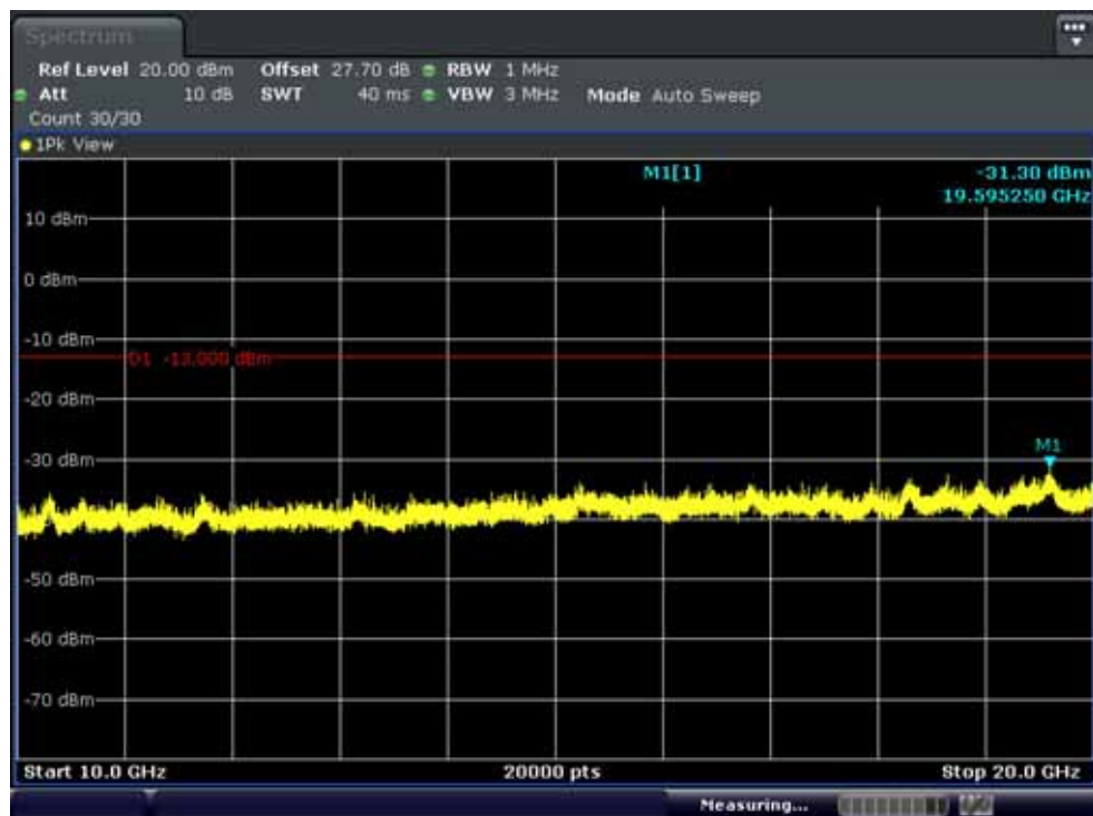
Band 4: Conducted Spurious Plot 2 (15MHz QPSK - RB Size 1, RB Offset 0 - Low Band 4: Channel)
