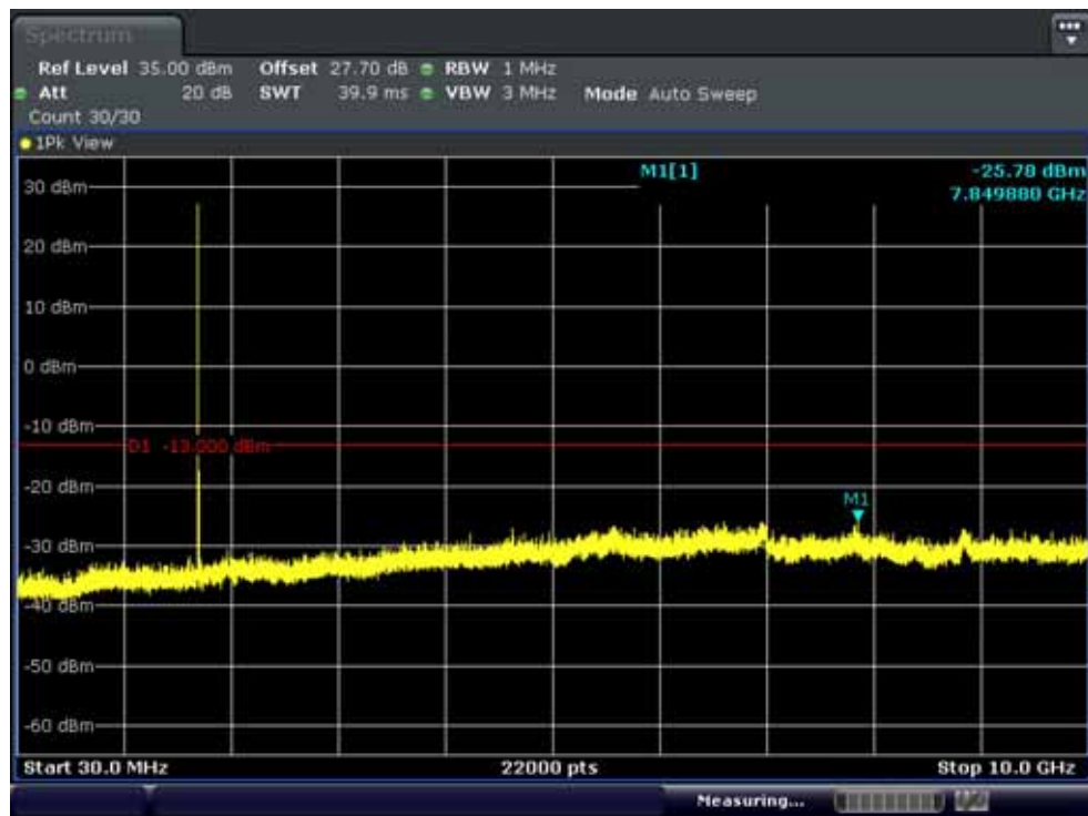
Band 4: Conducted Spurious Plot 1 (3MHz QPSK - RB Size 1, RB Offset 0 - Low Band 4: Channel)
