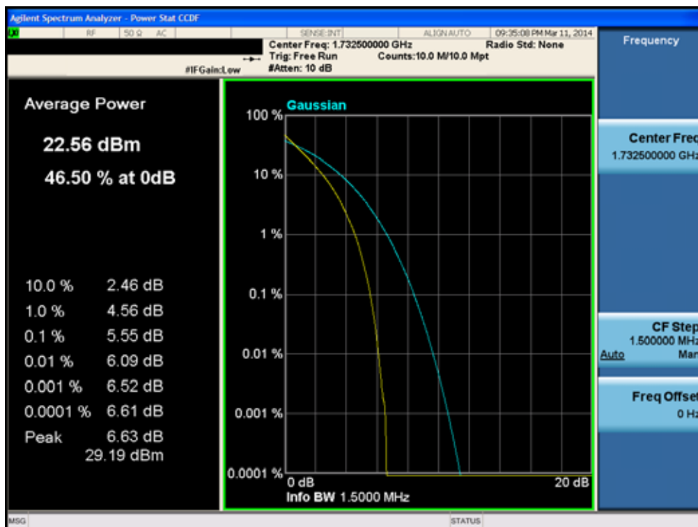
Peak to Average Ratio Plot (1.4M BW Ch.20175 16QAM RB 6)
