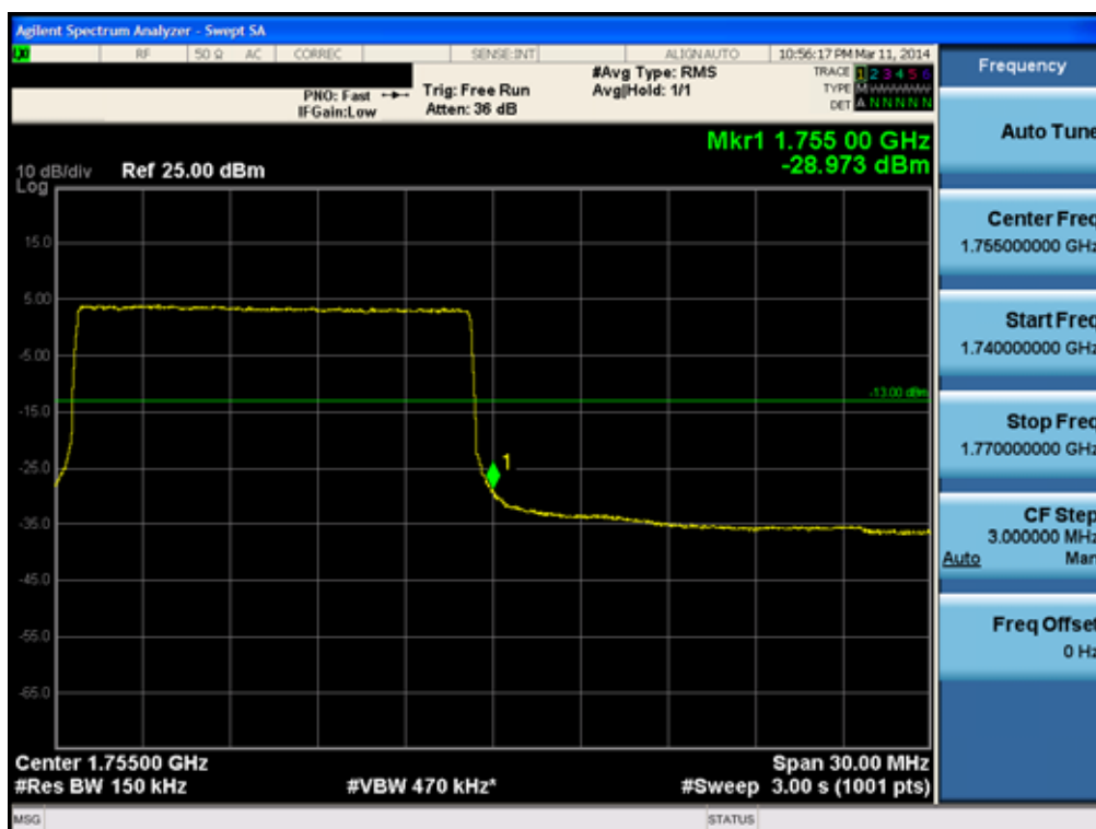
Upper Band Edge Plot (15M BW Ch.20325 QPSK RB 75) -2
