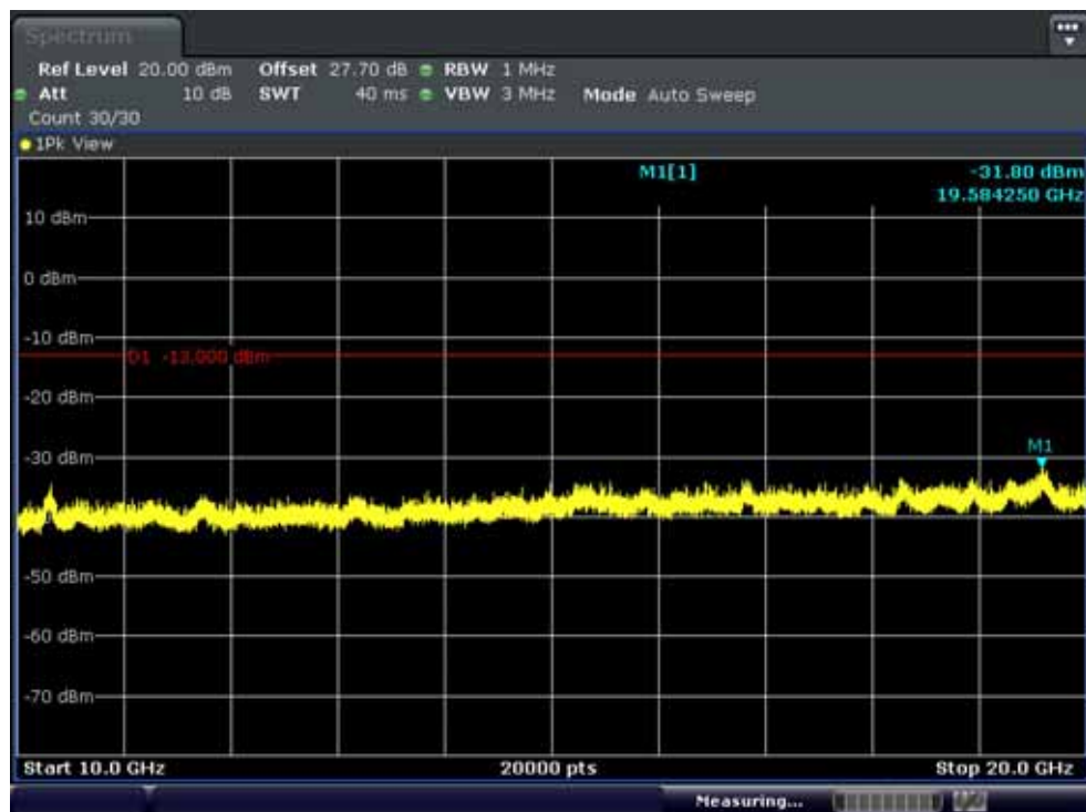
Band 4: Conducted Spurious Plot 2 (1.4MHz QPSK - RB Size 1, RB Offset 0 - High Band 4: Channel)
