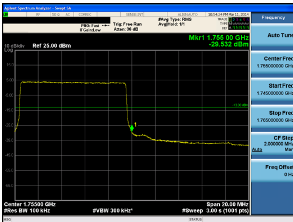
Upper Band Edge Plot (10M BW Ch.20350 QPSK RB 50) -2
