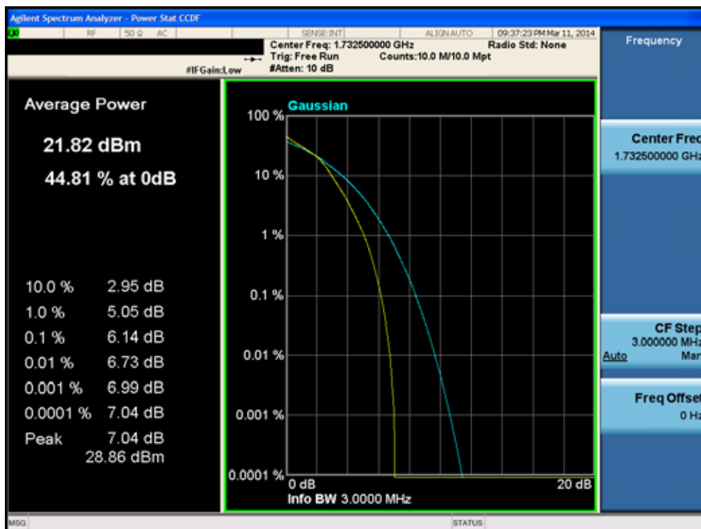
Peak to Average Ratio Plot (3M BW Ch.20175 16QAM RB 15)
