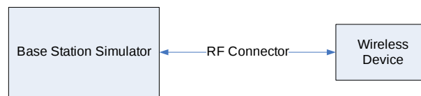
Figure 8-1 Power Measurement Setup
