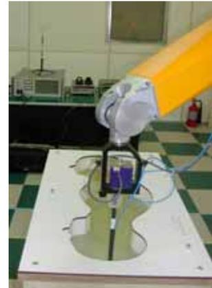
Figure 5. Photograph of the probe and the Phantom
