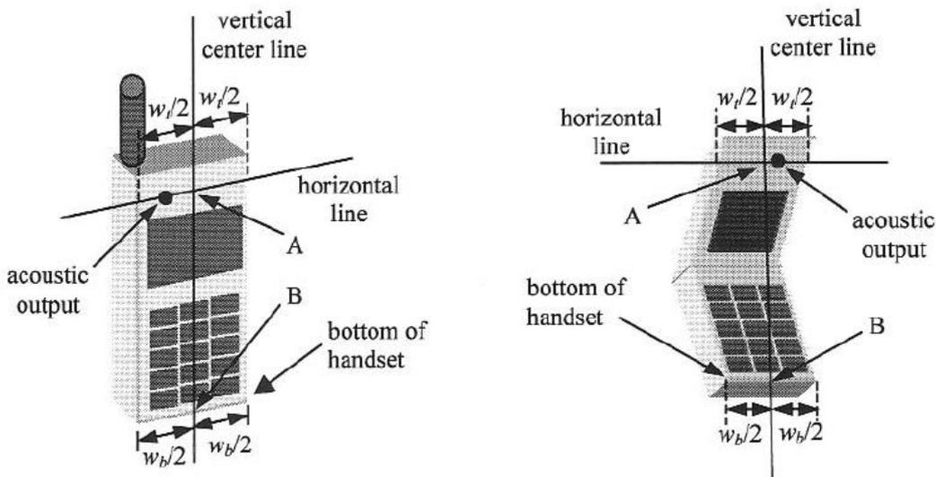
Figure 14. Handset vertical and horizontal reference lines
