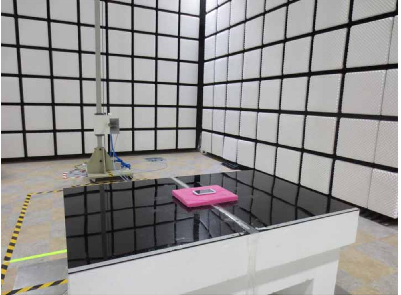
■ BT/WLAN Test Setup Photo
