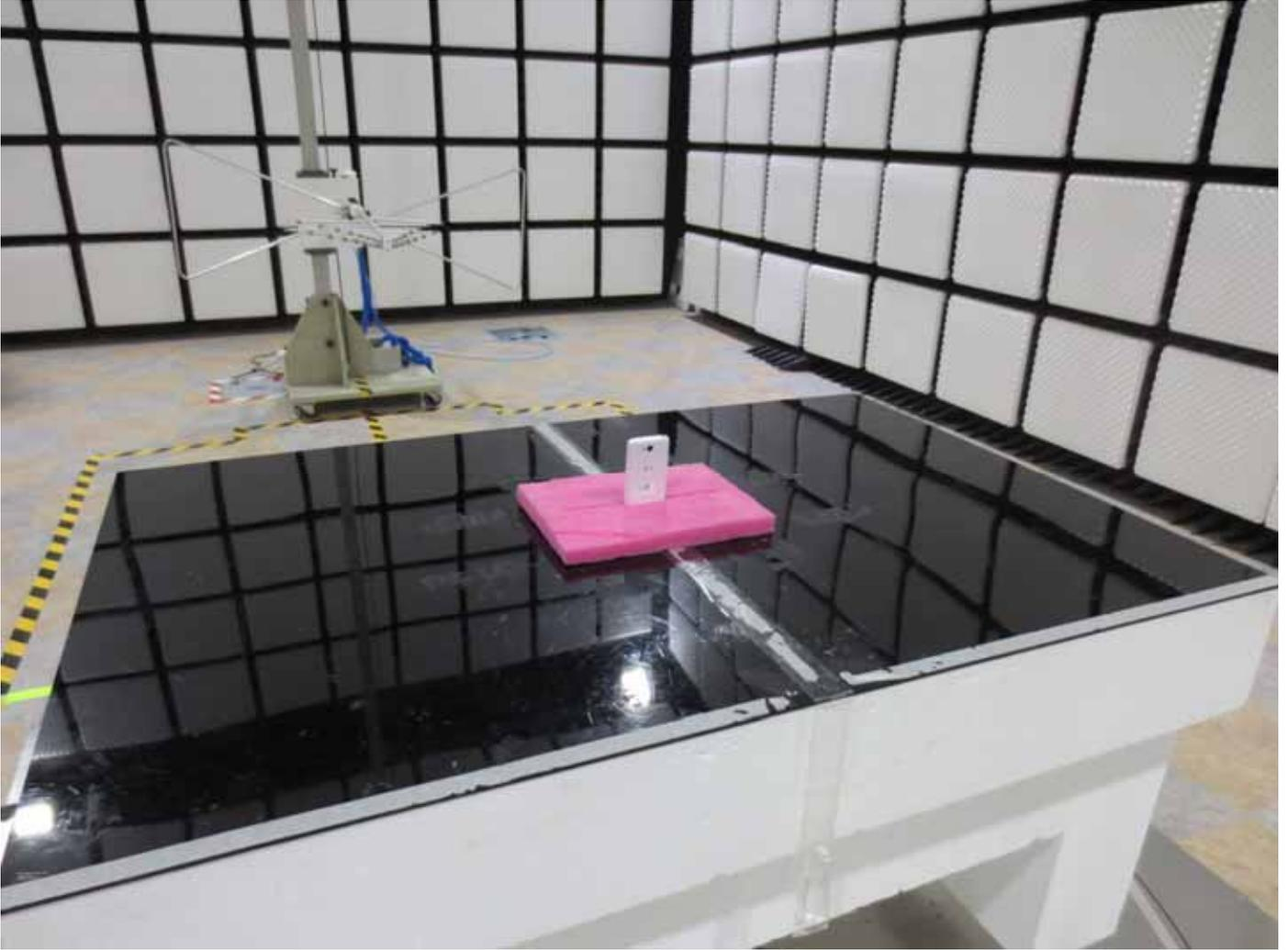
■ BT/WLAN Test Setup Photo
