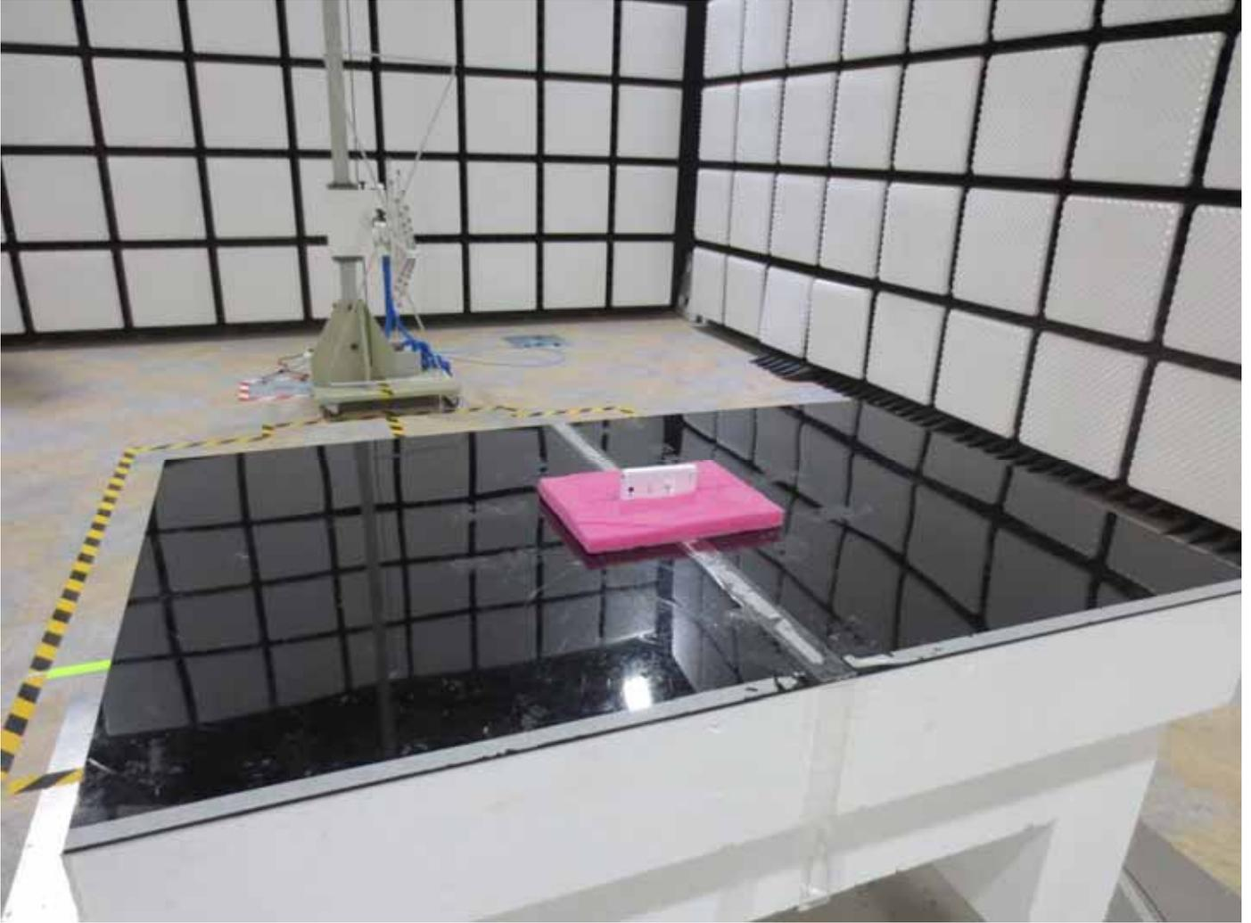
■ BT/WLAN Test Setup Photo
