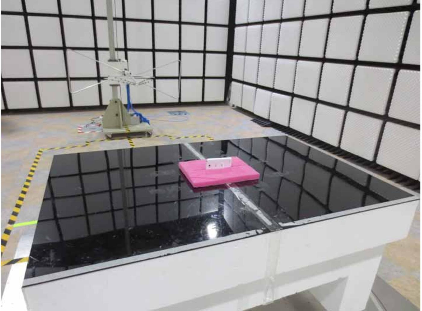
■ Conducted Emission Test Setup Photo
