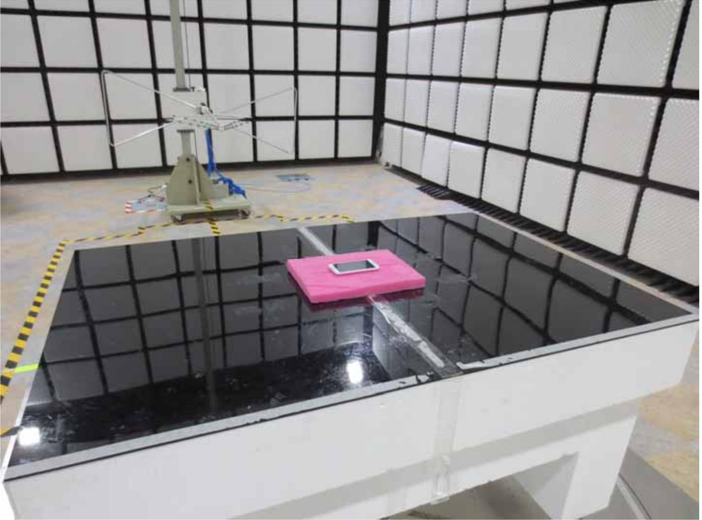
■ BT/WLAN Test Setup Photo
