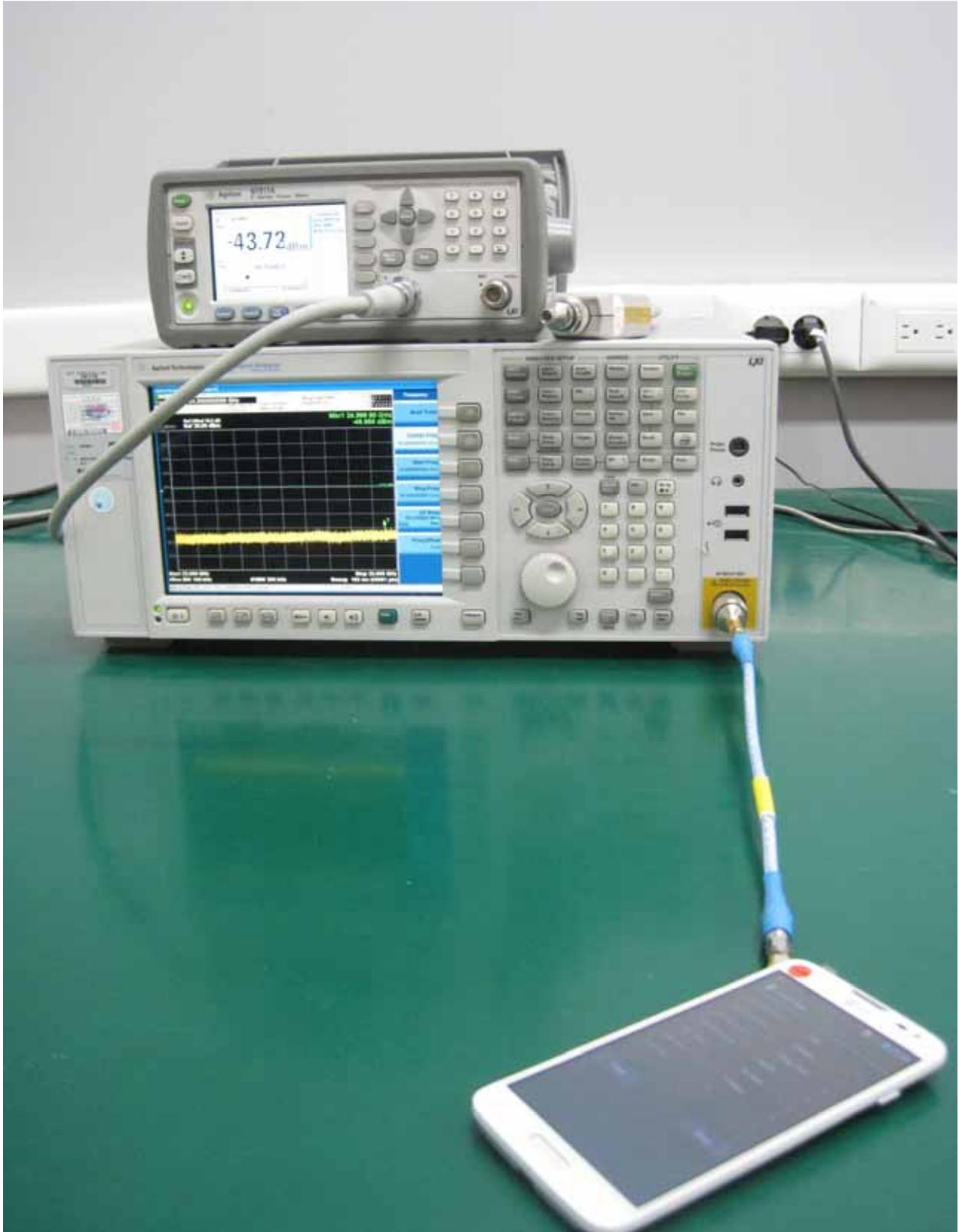
■ BT/WLAN Test Setup Photo
