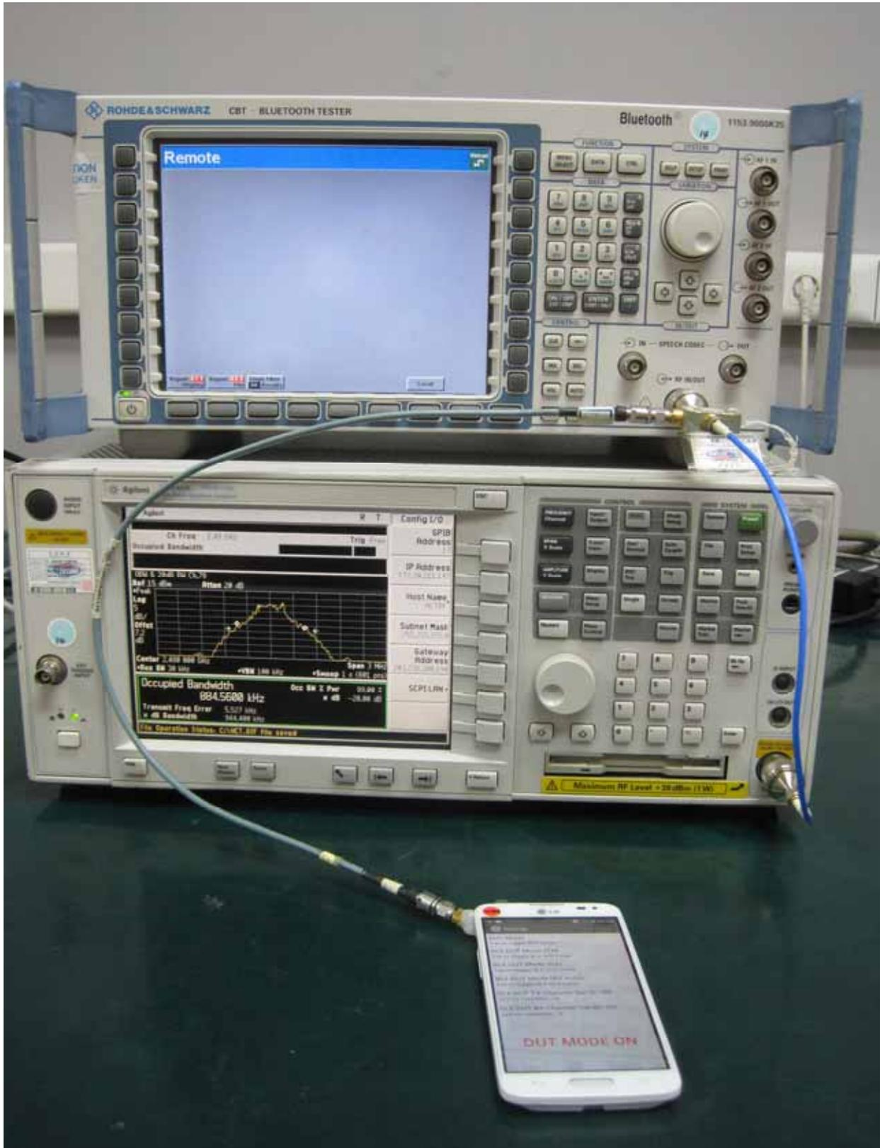
■ Conducted WLAN Test Setup Photo
