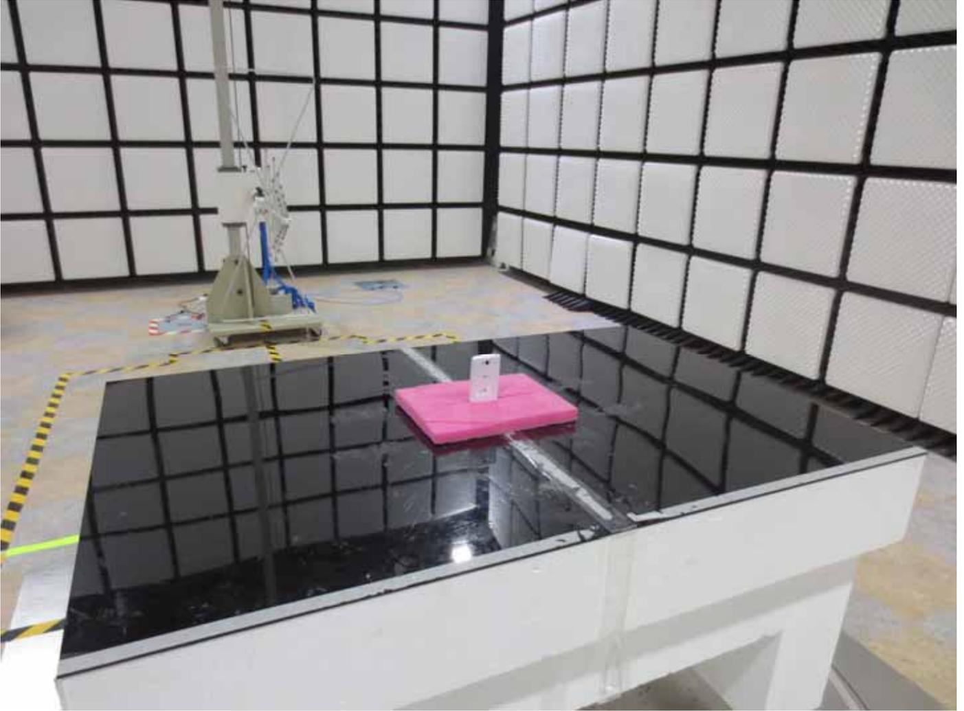
■ BT/WLAN Test Setup Photo
