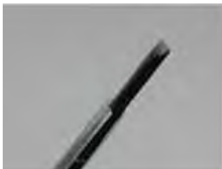
Figure 6. EX3DV4 E-field Probe
