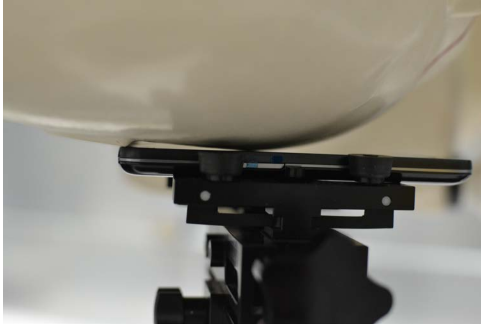
SAR Test Setup Photo 1 - Right Cheek
