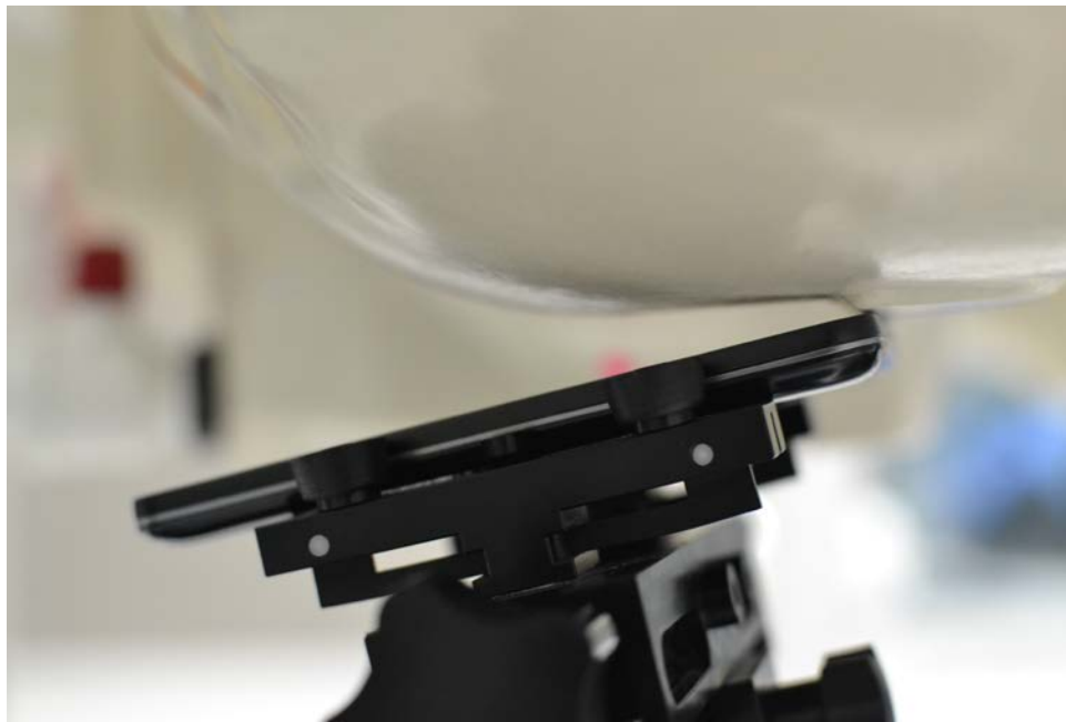
SAR Test Setup Photo 4 – Left Tilt
