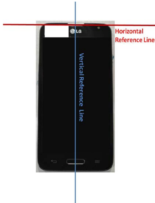
SAR Test Setup Photo 11 – Horizontal and Vertical Reference Lines
