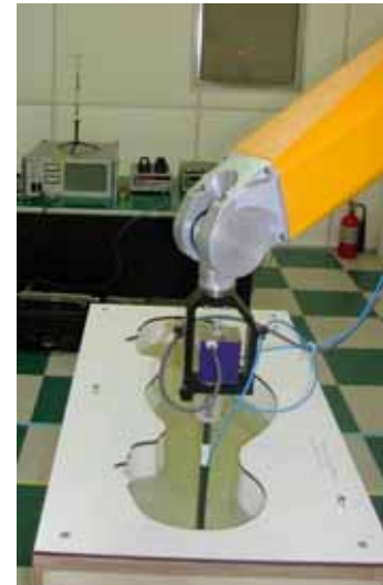
Figure 3. Photograph of the probe and the Phantom
