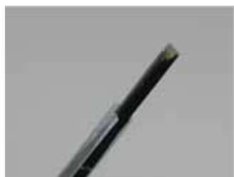
Figure 6. EX3DV4 E-field Probe
