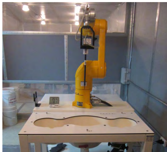
Figure 2.2 DASY5 Test System
