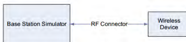
Figure 10.1 Power Measurement Setup
