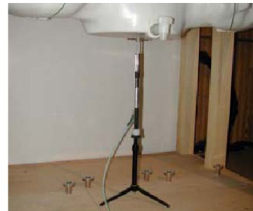
Figure 11.1 Dipole Verification Test Setup Diagram & Photo
