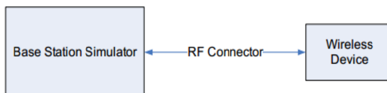
Figure 10.2 Power Measurement Setup
