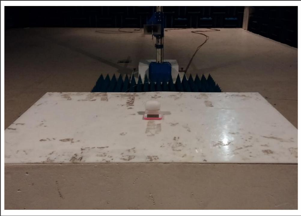
**Test Setup photo of Conducted Emissions (DTS & DSS)**
