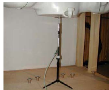
Figure 11.1 Dipole Verification Test Setup Diagram & Photo
