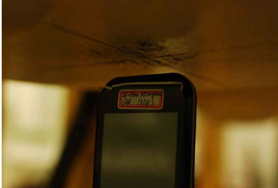
SAR Test Setup Photo 7: Top at 1.0 cm
