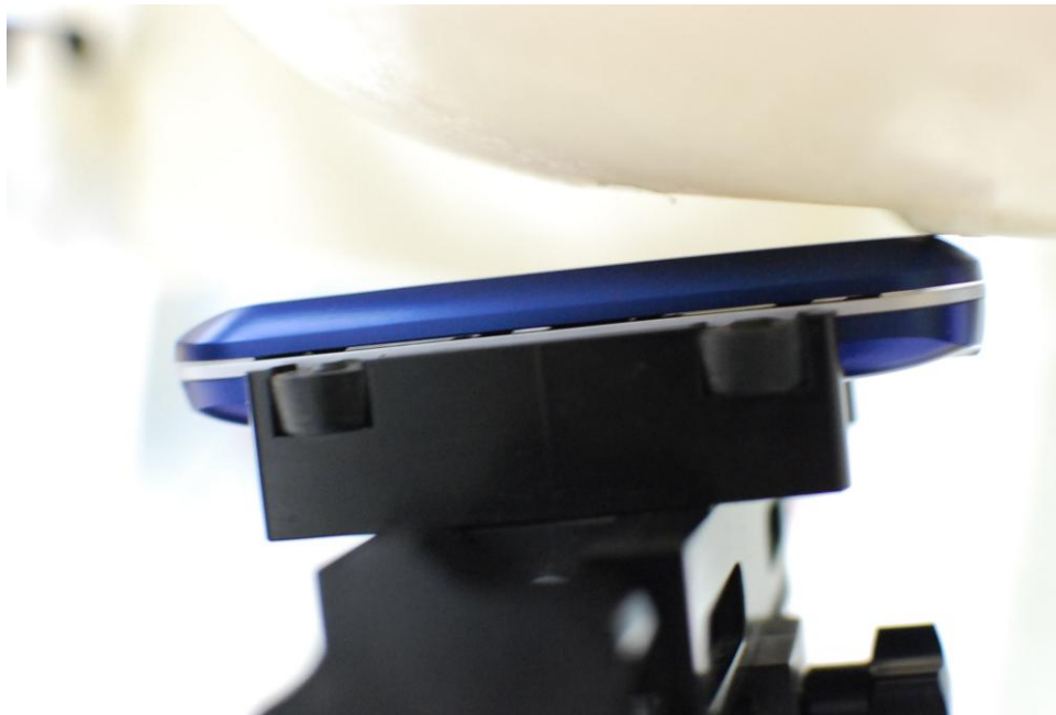
SAR Test Setup Photo 4 - Left Tilt
