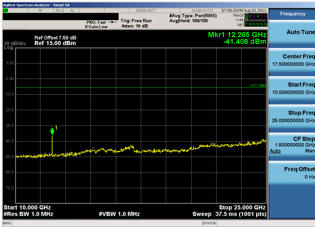
Plot 6-19. Conducted Spurious Plot (Bluetooth, 3Mbps – Ch. 39)
