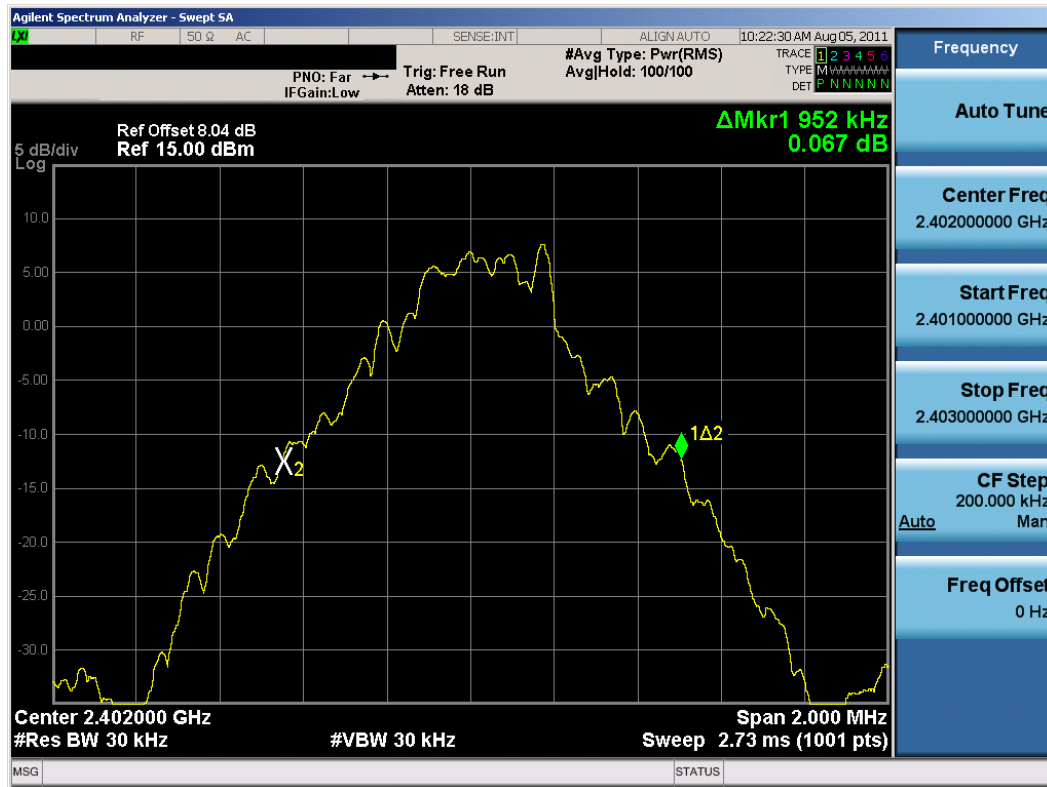
Plot 6-1. 20dB Bandwidth Plot (Bluetooth, 1Mbps – Ch. 0)
