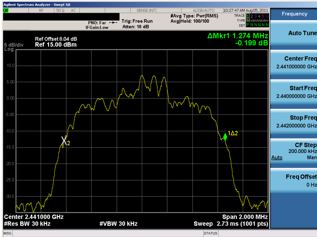
Plot 6-5. 20dB Bandwidth Plot (Bluetooth, 2Mbps – Ch. 39)
