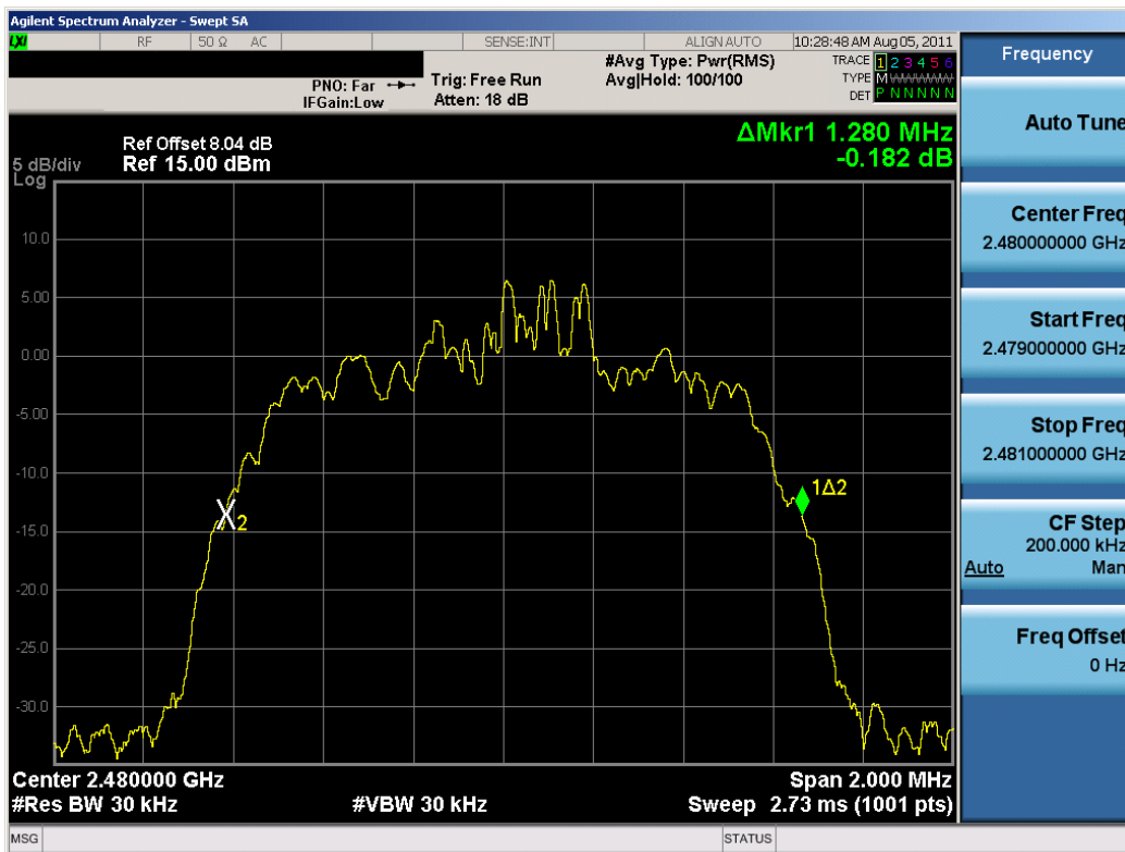
Plot 6-6. 20dB Bandwidth Plot (Bluetooth, 2Mbps – Ch. 78)
