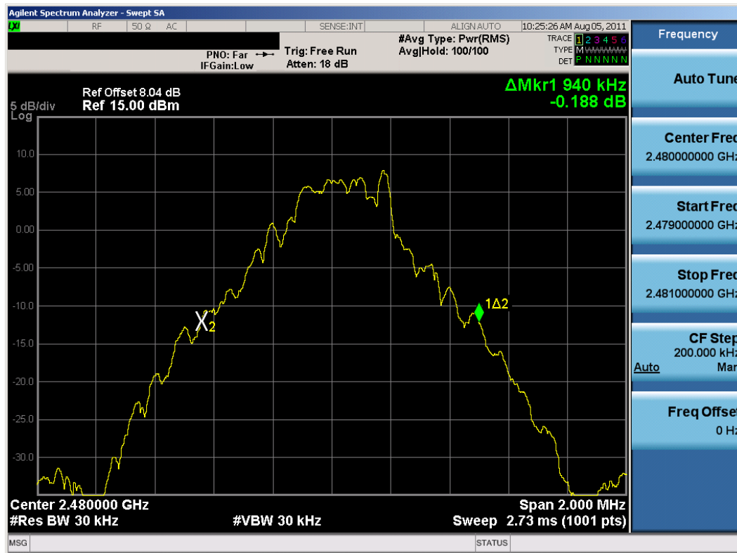
Plot 6-3. 20dB Bandwidth Plot (Bluetooth, 1Mbps – Ch. 78)
