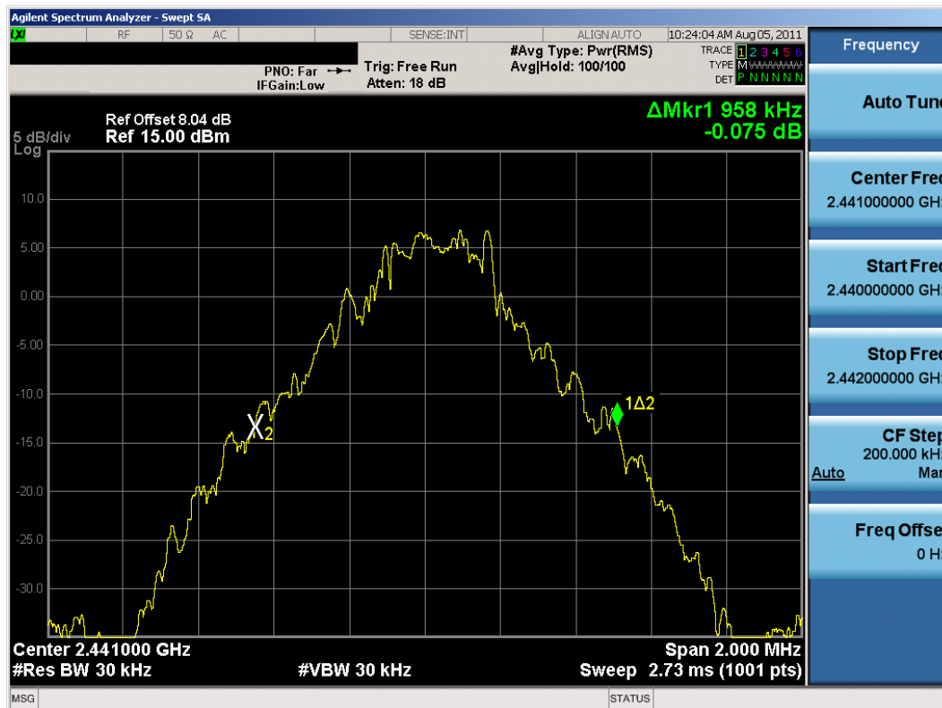
Plot 6-2. 20dB Bandwidth Plot (Bluetooth, 1Mbps – Ch. 39)
