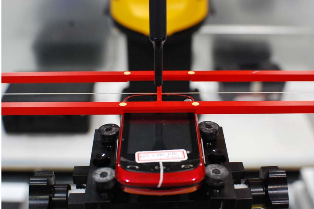
Figure 17-1 Ear Reference Point HAC Phantom Alignment
