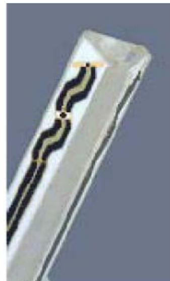
Figure 3.3 Probe Thick-Film Technique
