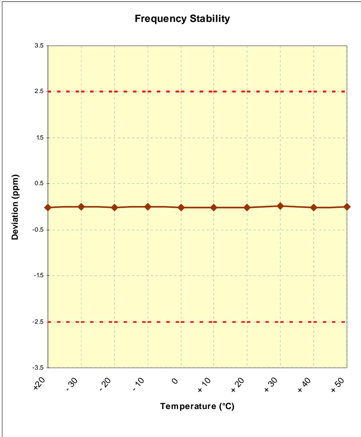
**Figure 6-2. Frequency Stability Graph (PCS CDMA Mode – Ch. 600)**
