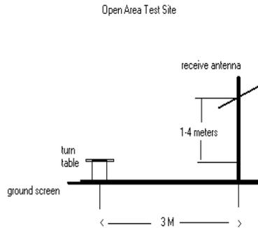
**Figure 3-1. Diagram of 3-meter outdoor test range**
