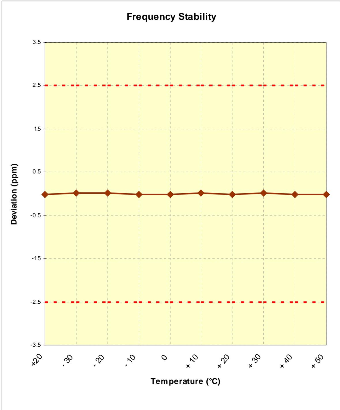
**Figure 6-1. Frequency Stability Graph (Cellular CDMA Mode – Ch. 384)**
