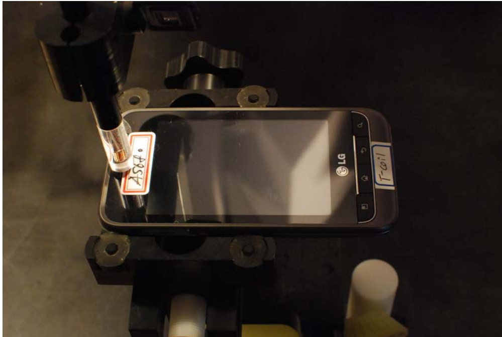
Figure 13-1 Test Setup for Wireless Device
