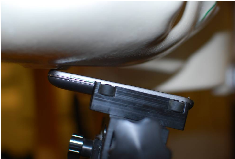
SAR Test Setup Photo 2 – Right Tilt
