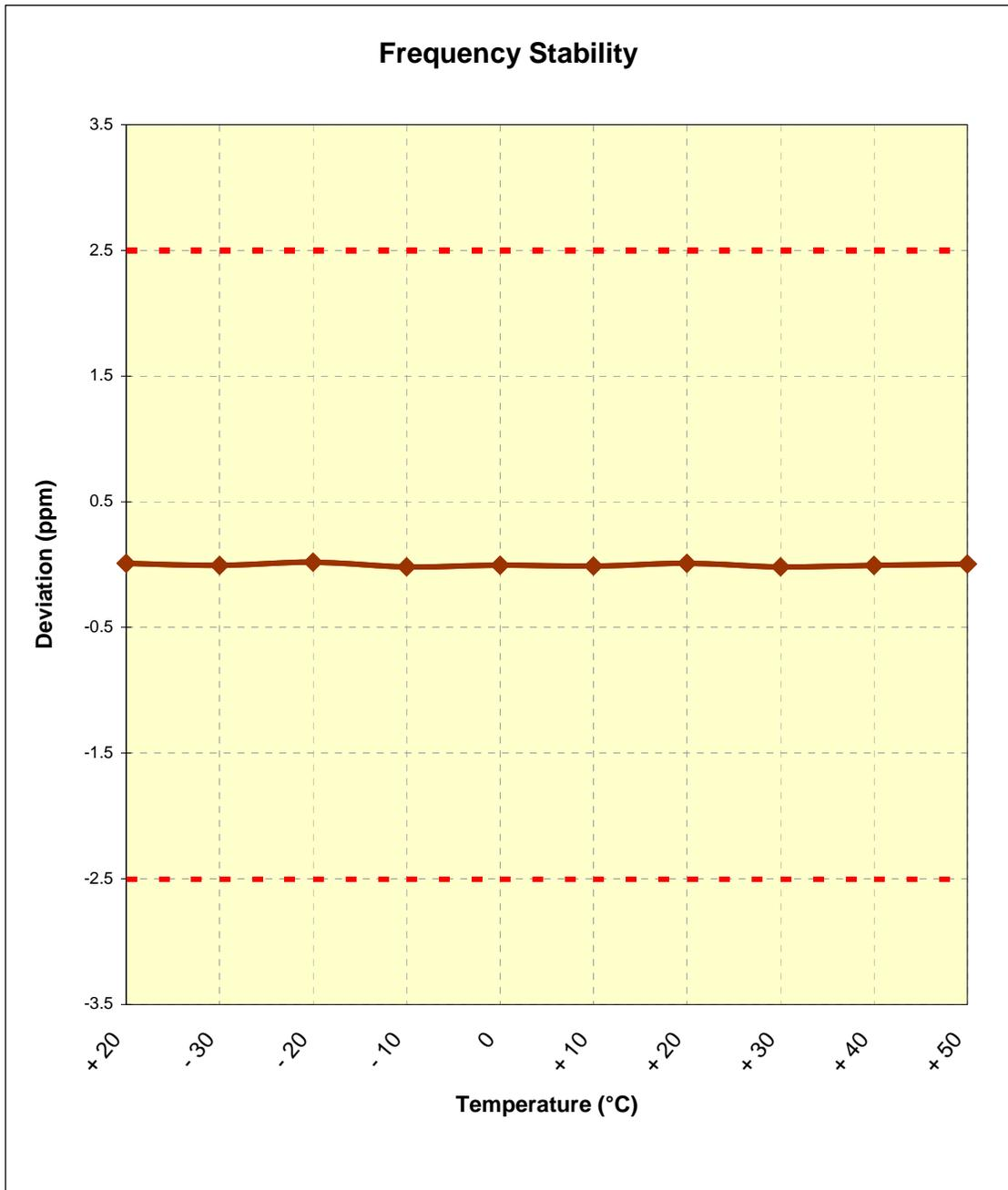
**Figure 6-1. Frequency Stability Graph (Cellular CDMA Mode – Ch. 384)**
