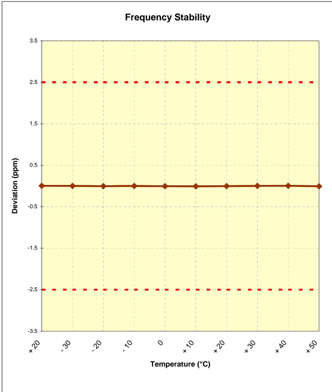
**Figure 6-2. Frequency Stability Graph (PCS CDMA Mode – Ch. 600)**
