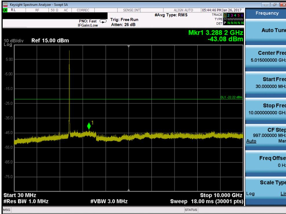
Plot 7-27. Conducted Spurious Plot (802.11b – Ch. 6)
