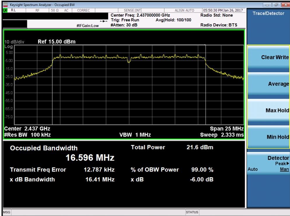
Plot 7-5. 6dB Bandwidth Plot (802.11g – Ch. 6)
