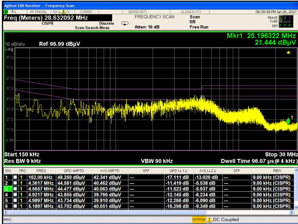
Plot 7-48. Line Conducted Plot with 802.11b (L1)
