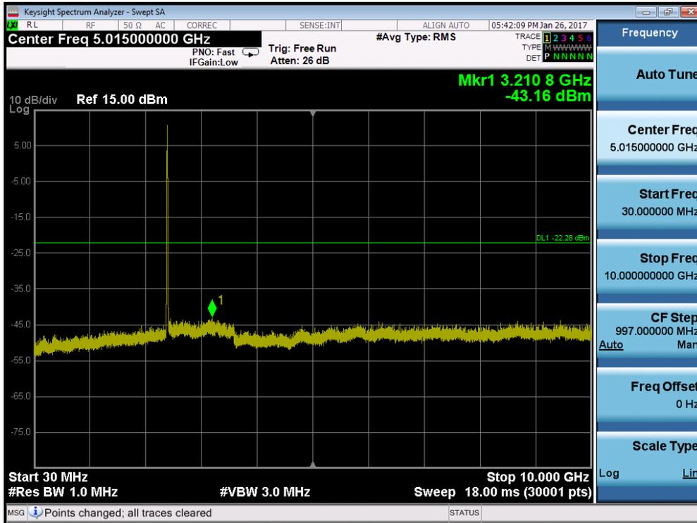
Plot 7-25. Conducted Spurious Plot (802.11b – Ch. 1)
