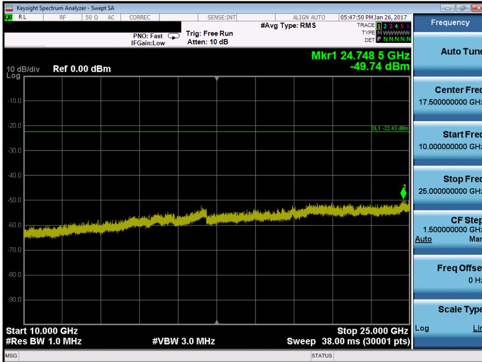
Plot 7-30. Conducted Spurious Plot (802.11b – Ch. 11)
