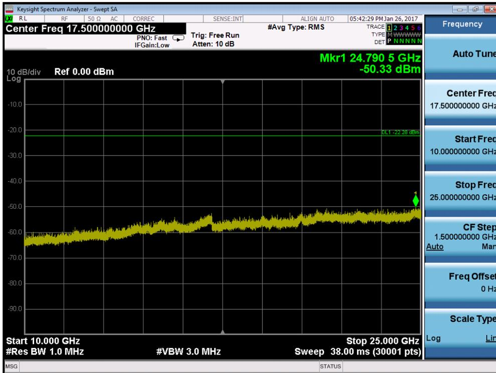
Plot 7-26. Conducted Spurious Plot (802.11b – Ch. 1)
