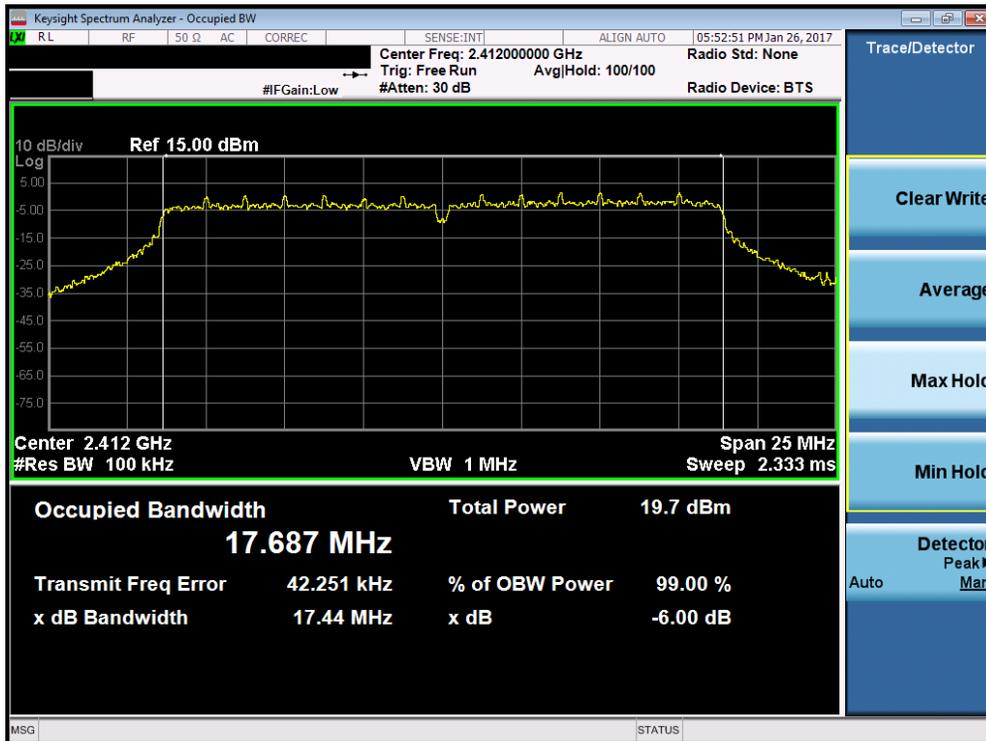
Plot 7-7. 6dB Bandwidth Plot (802.11n (2.4GHz) – Ch. 1)
