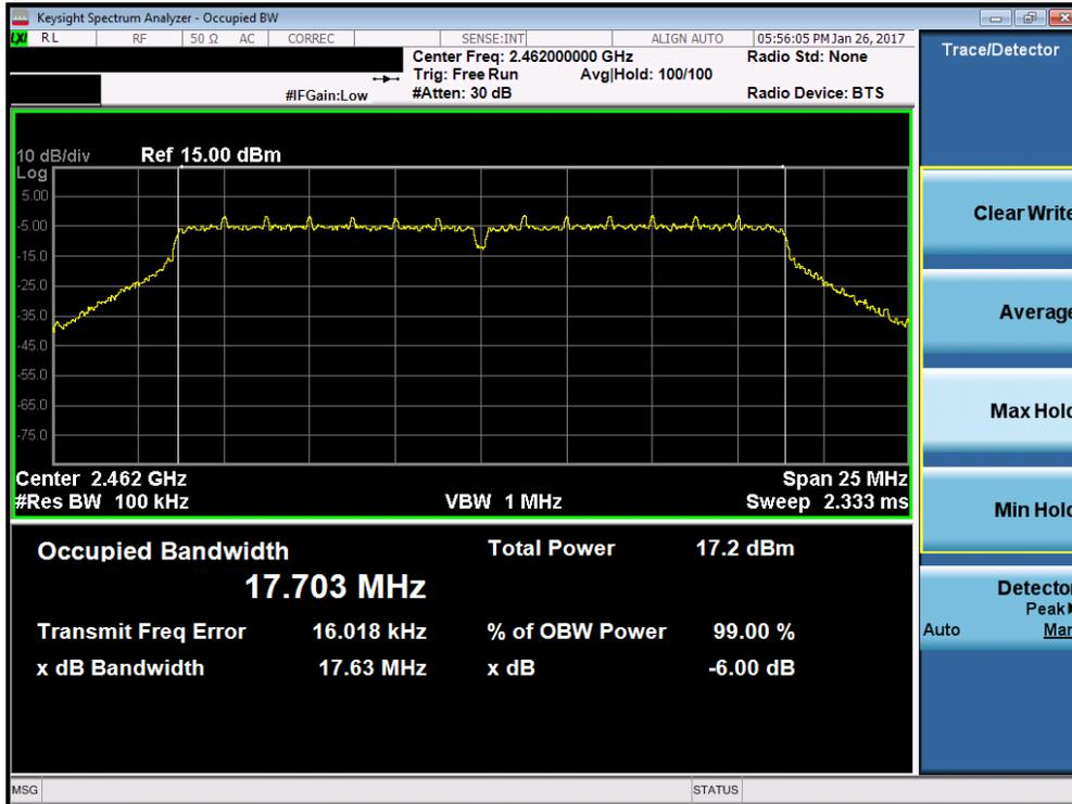
Plot 7-9. 6dB Bandwidth Plot (802.11n (2.4GHz) – Ch. 11)
