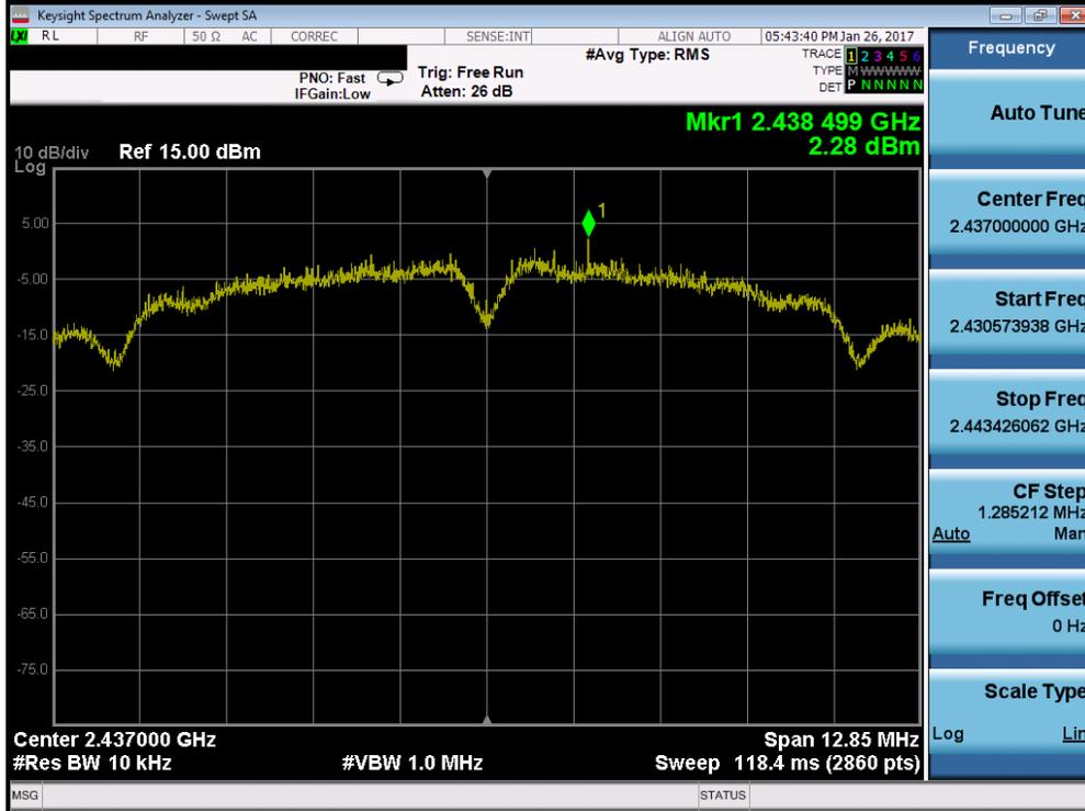
Plot 7-11. Power Spectral Density Plot (802.11b – Ch. 6)
