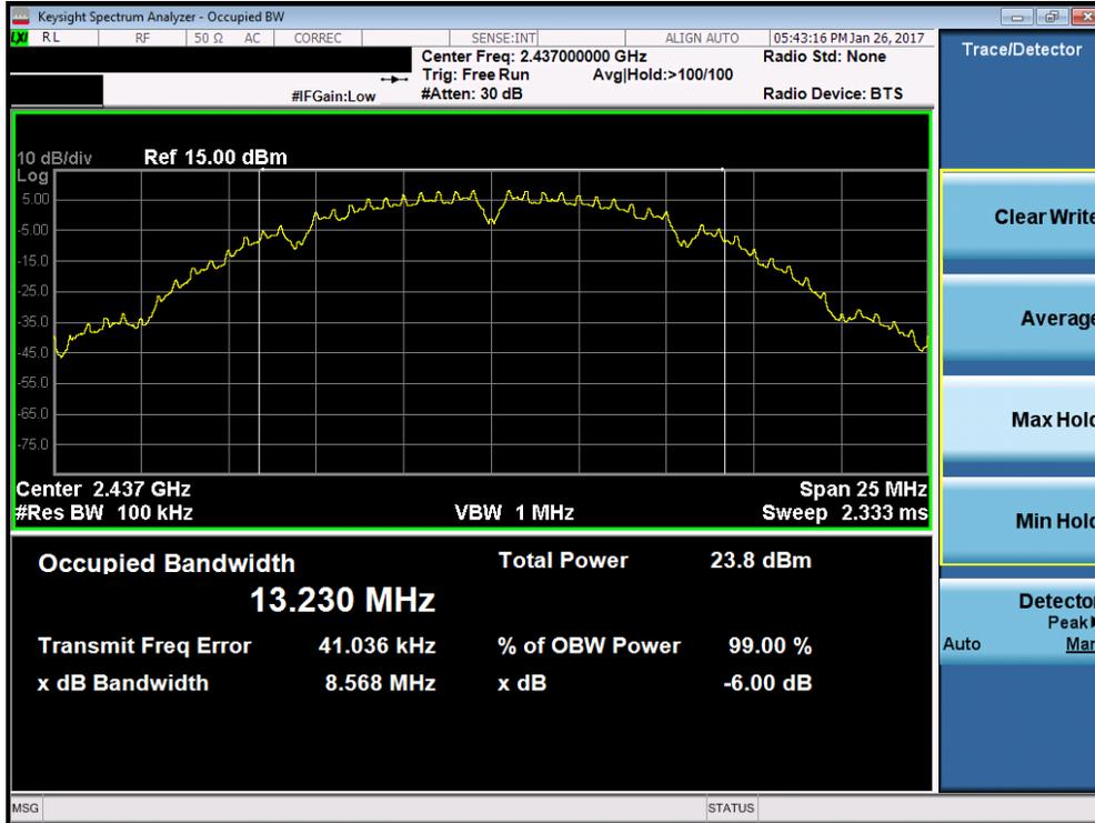
Plot 7-2. 6dB Bandwidth Plot (802.11b – Ch. 6)
