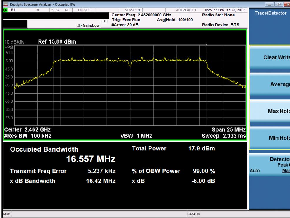
Plot 7-6. 6dB Bandwidth Plot (802.11g – Ch. 11)
