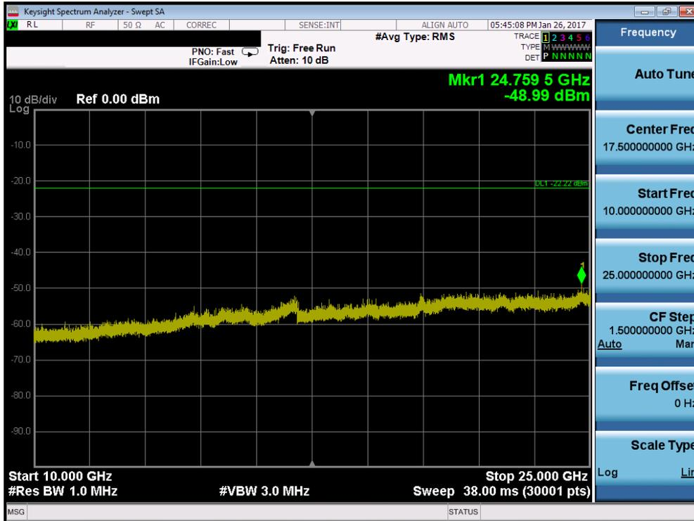
Plot 7-28. Conducted Spurious Plot (802.11b – Ch. 6)
