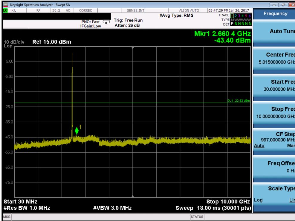
Plot 7-29. Conducted Spurious Plot (802.11b – Ch. 11)
