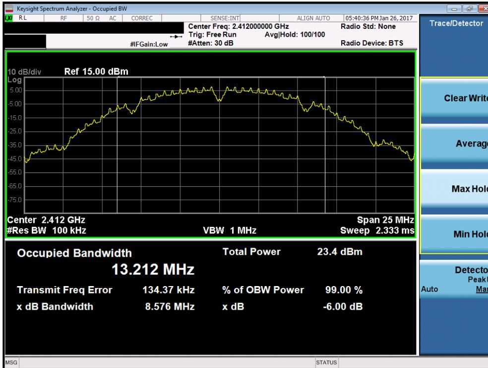
Plot 7-1. 6dB Bandwidth Plot (802.11b – Ch. 1)
