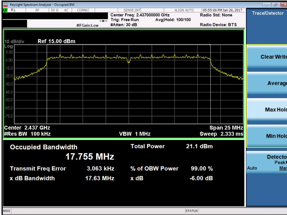
Plot 7-8. 6dB Bandwidth Plot (802.11n (2.4GHz) – Ch. 6)
