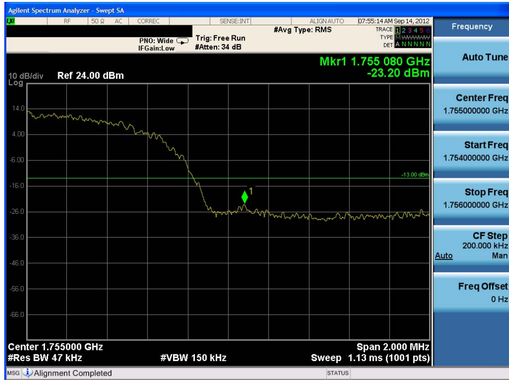
Plot 7-11. Band Edge Plot (AWS WCDMA Mode – Ch. 1862)
