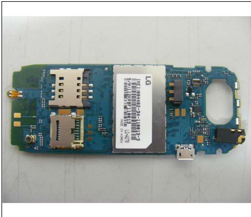
***Bottom view of main board (Removing Shield)***
