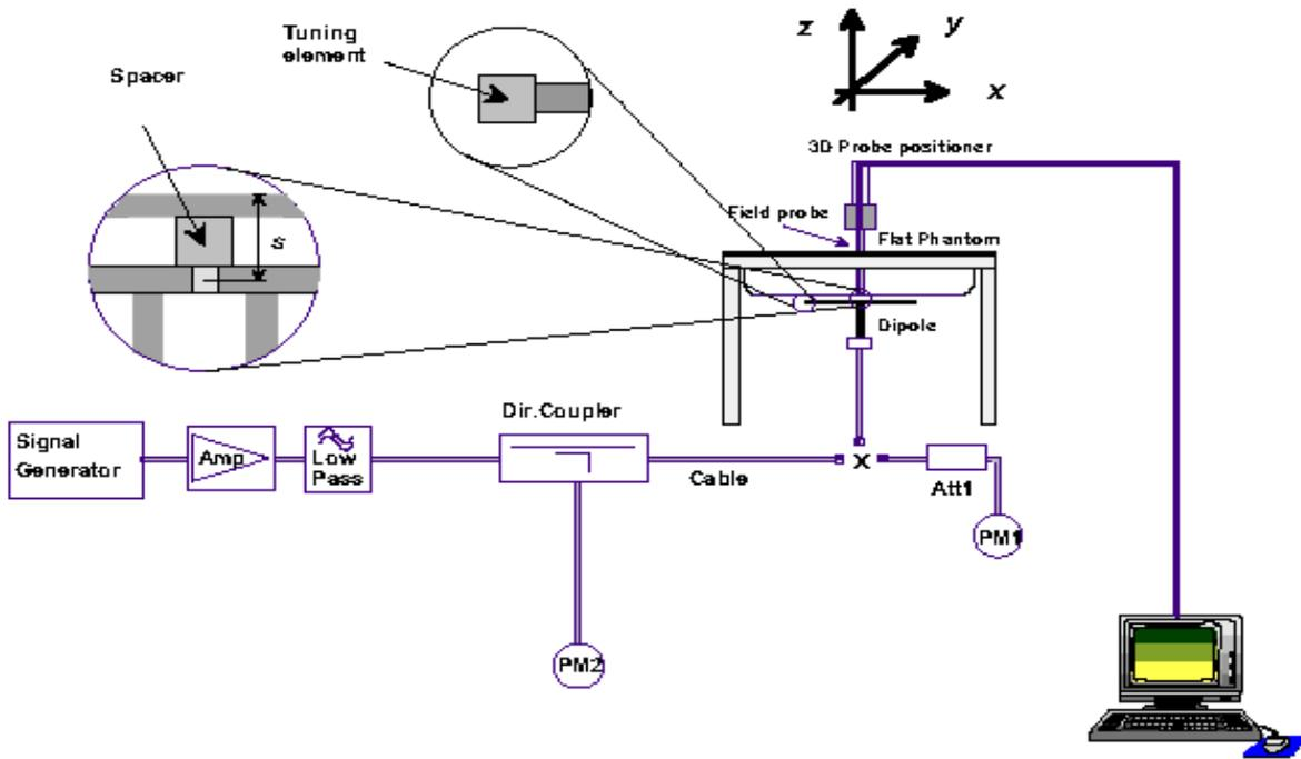
Fig b. System verification Setup Diagram
