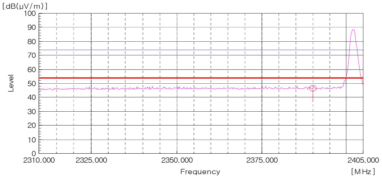
AV Detector: RBW: 1 MHz, VBW: 10 Hz (2 310 MHz - 2 405 MHz), Worst case (Low, Vertical)
