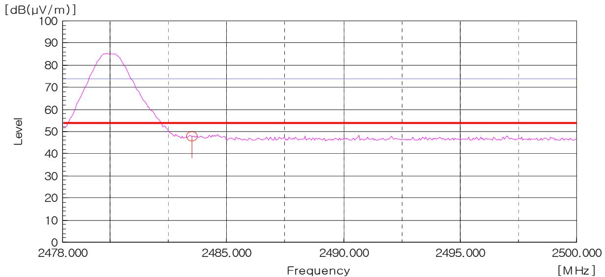
AV Detector: RBW: 1MHz, VBW: 10 Hz (2 478.0 MHz - 2 500.0 MHz), Worst case (High, Vertical)
